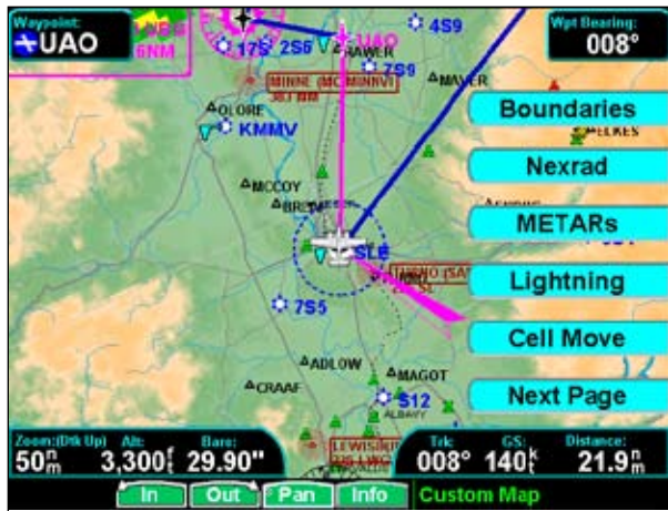
Custom Map page with Boundaries, Nexrad, Metars, Lightning, and Cell Movement Menu Items (Page 4)
