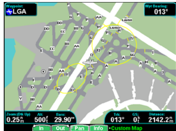
Custom Map page with detail for an-airport where SafeTaxi Hot Spots and LAHSO information is available.
