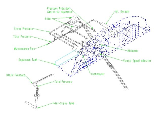
Figure: Pitot-Static System Schematic
