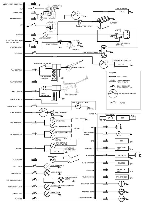
Fig.: Electrical System Schematic
