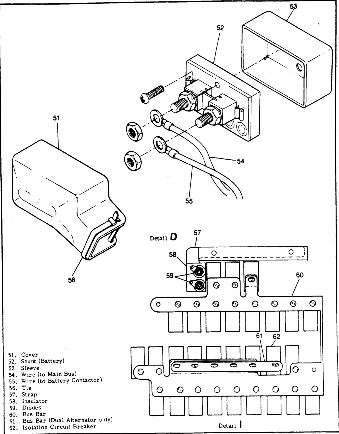
Figure 17-6B. Dual Alternator System Installation (Sheet 6 of 8)
