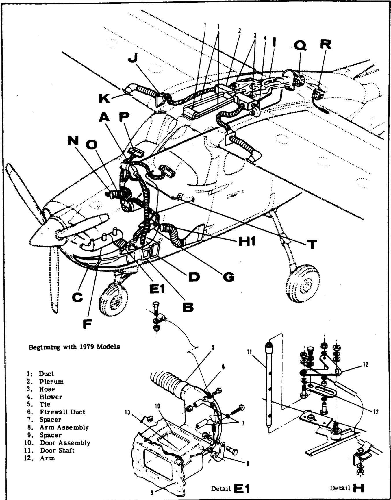
Figure 15-1. Heating, Ventilating and Pressurization System (Sheet 2 of 5)
