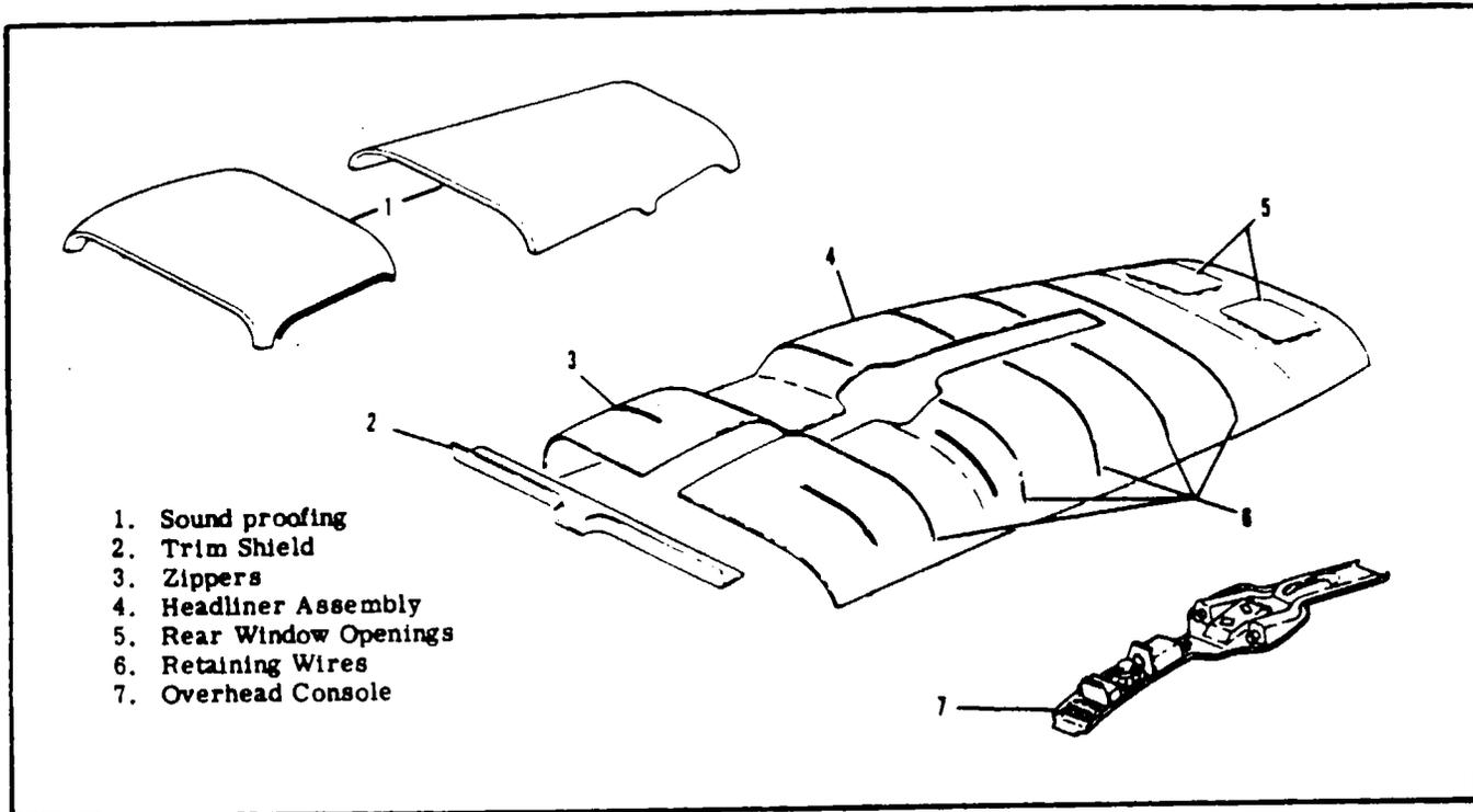
Figure 3-9. Cabin Headliner Installation
