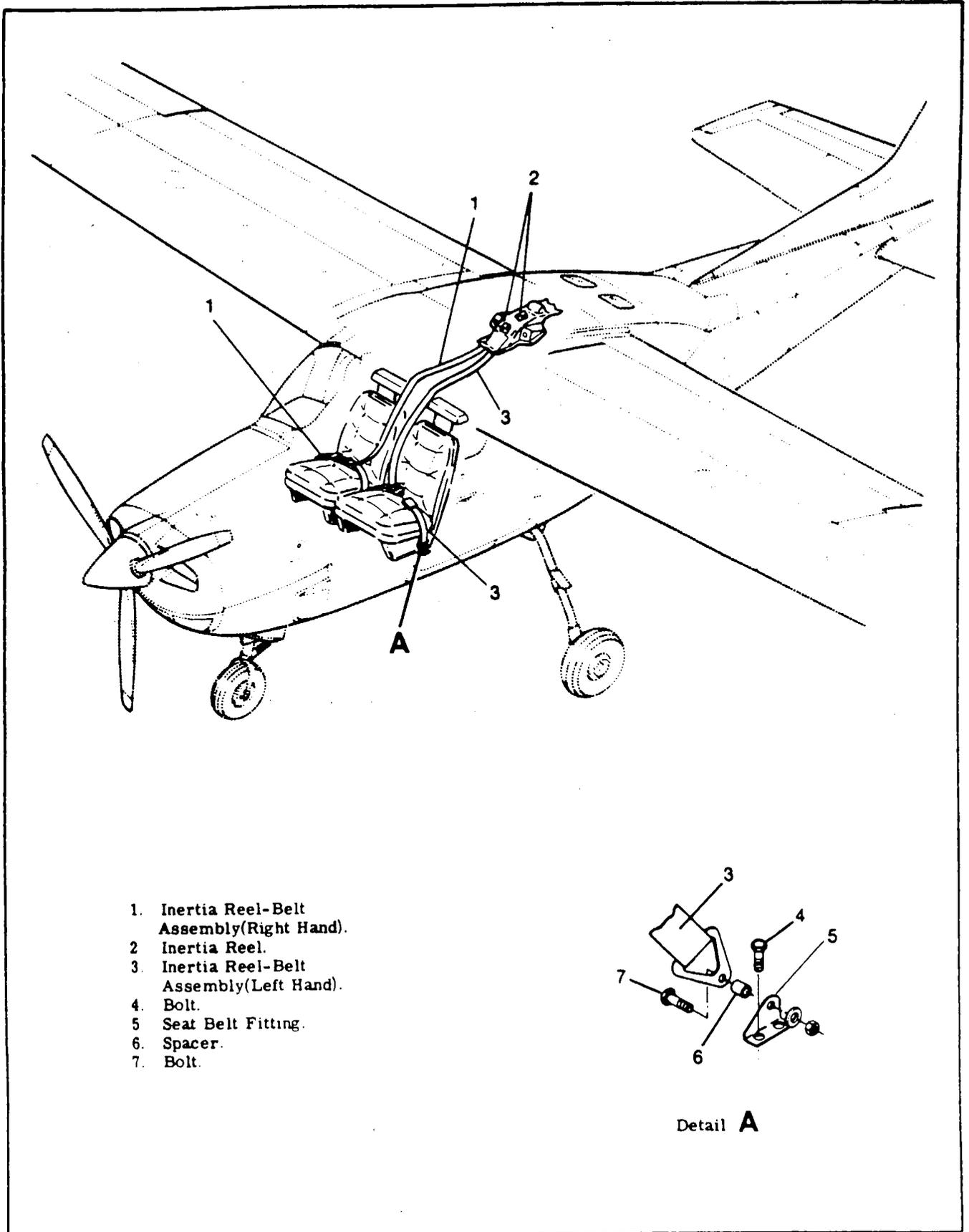
Figure 3-9B. Inertia Reel Harness
