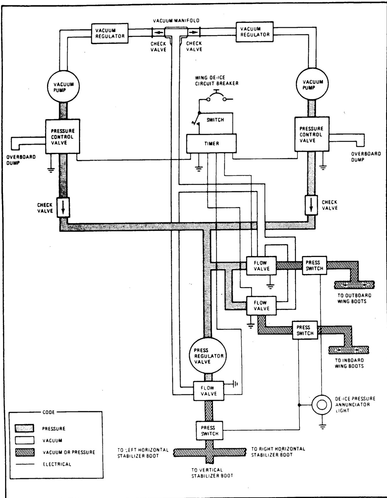
Figure 15-4B. Surface De-Ice System Components Schematic.
