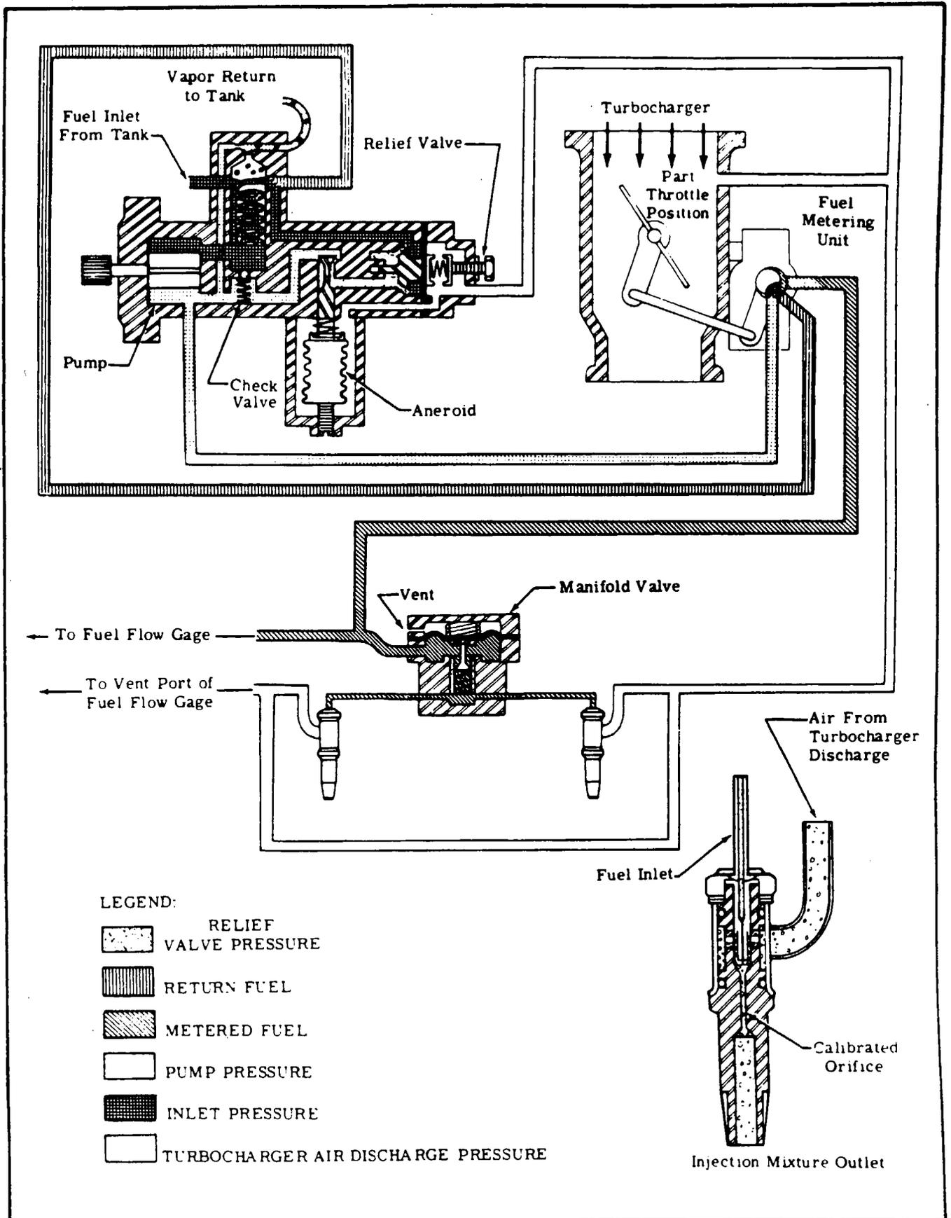
Figure 12-6. Fuel System Schematic
