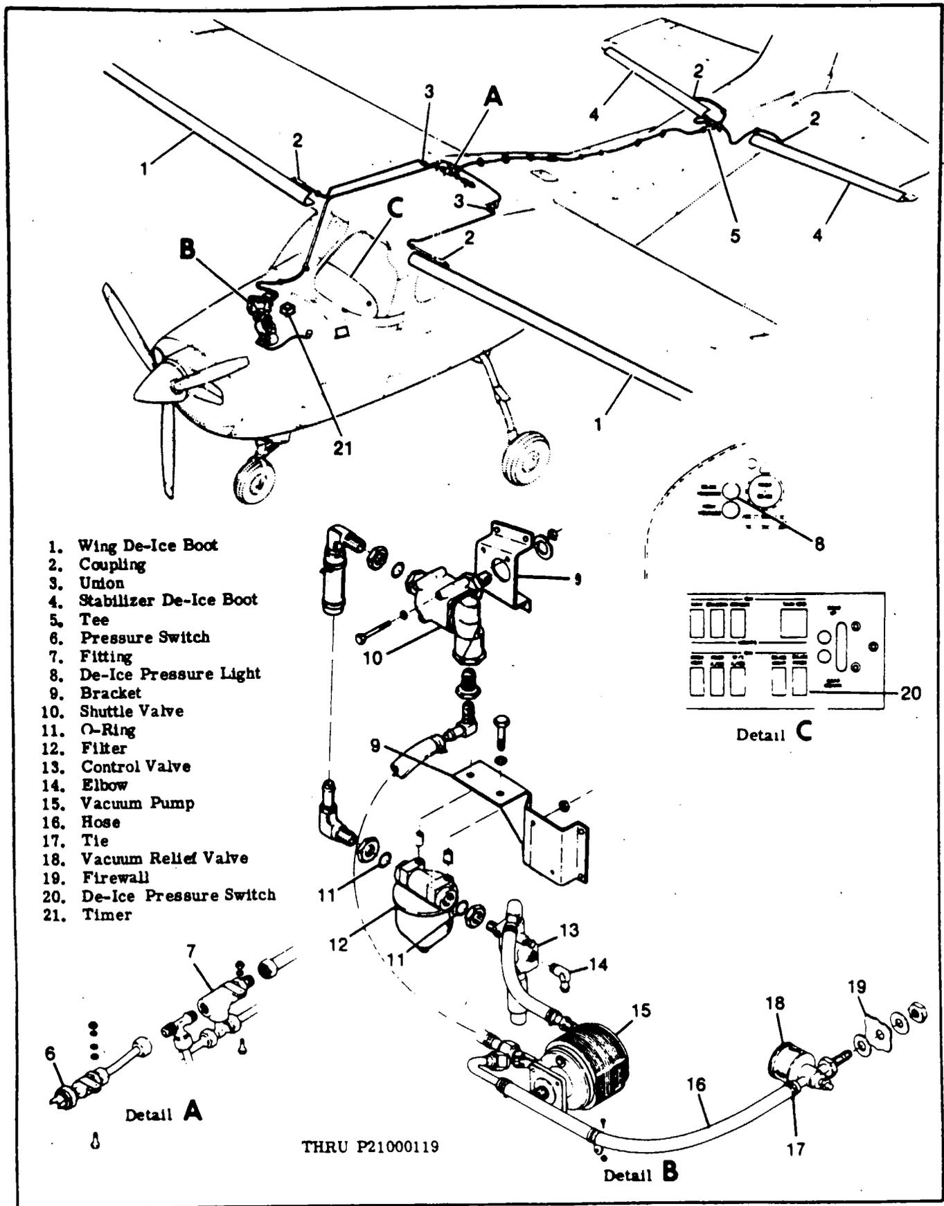
Figure 15-3. Wing and Horizontal Stabilizer One-Cycle De-ice System
