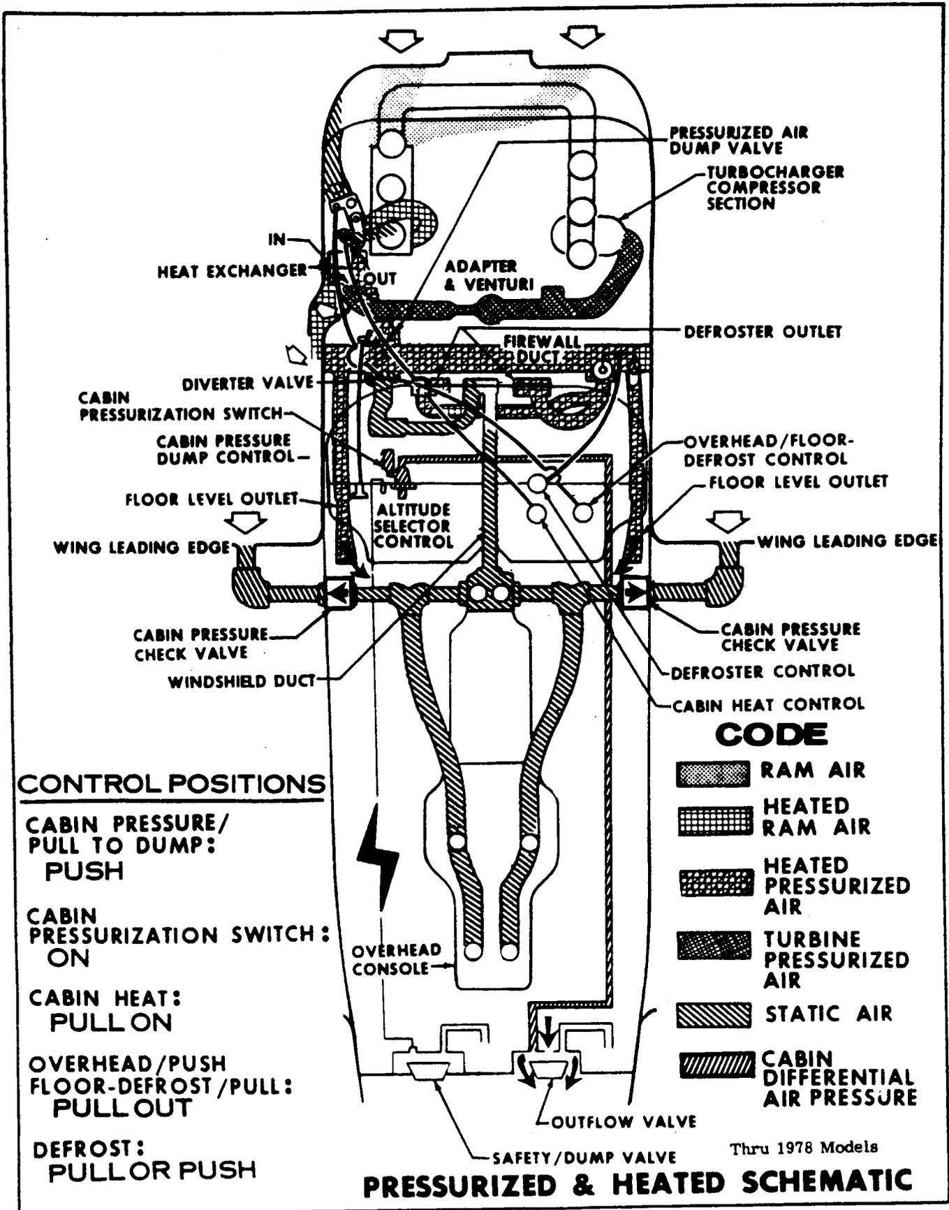
Figure 15-2. Cabin Air Flow Schematic (Sheet 3 of 6)
