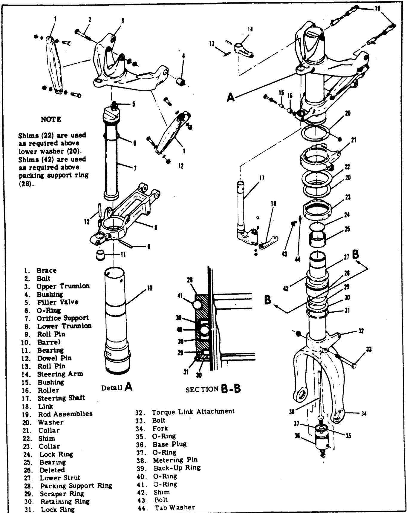
Figure 5-16. Nose Gear Shock Strut Assembly
