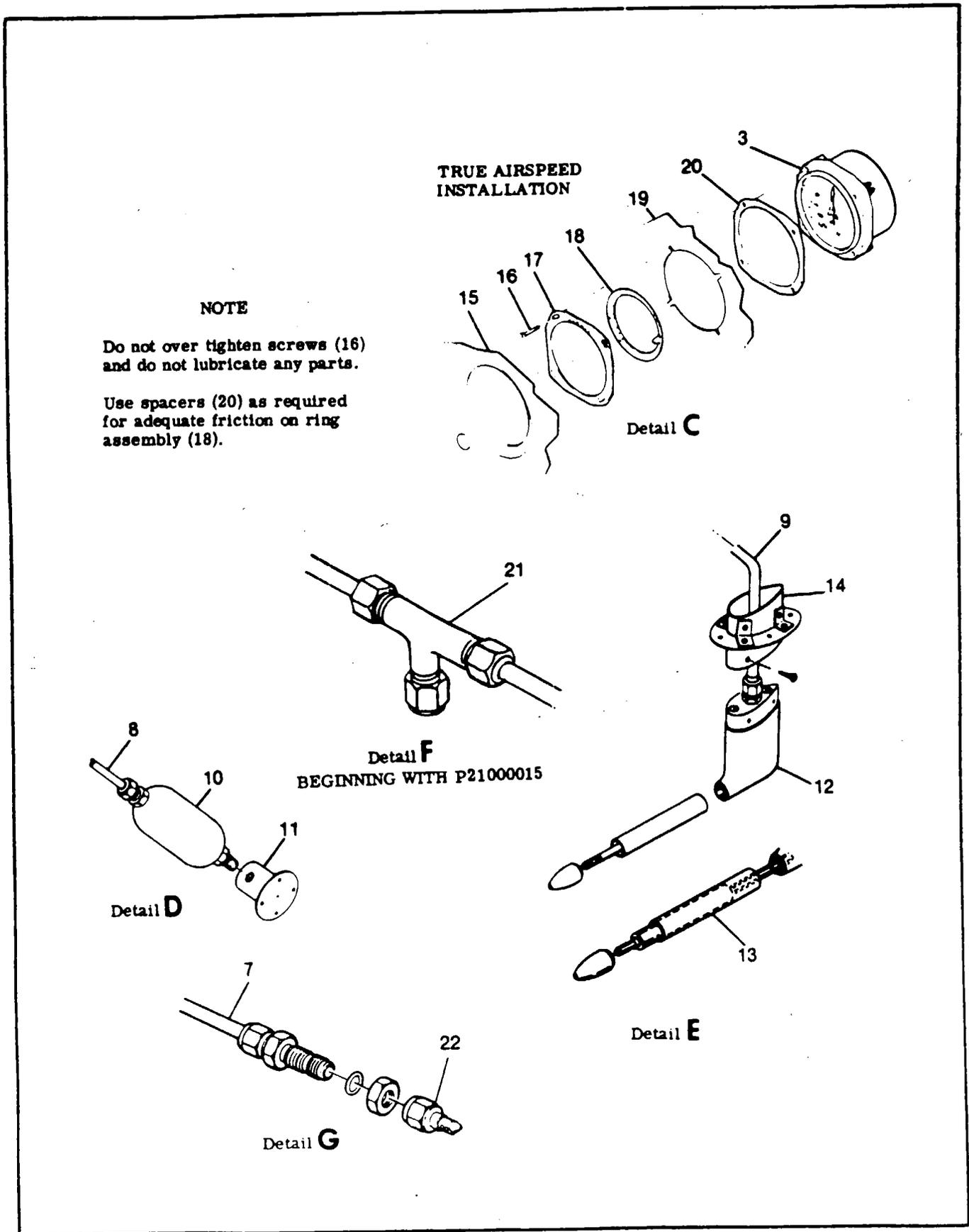
Figure 16-2. Pitot Static System (Sheet 2 of 2)
