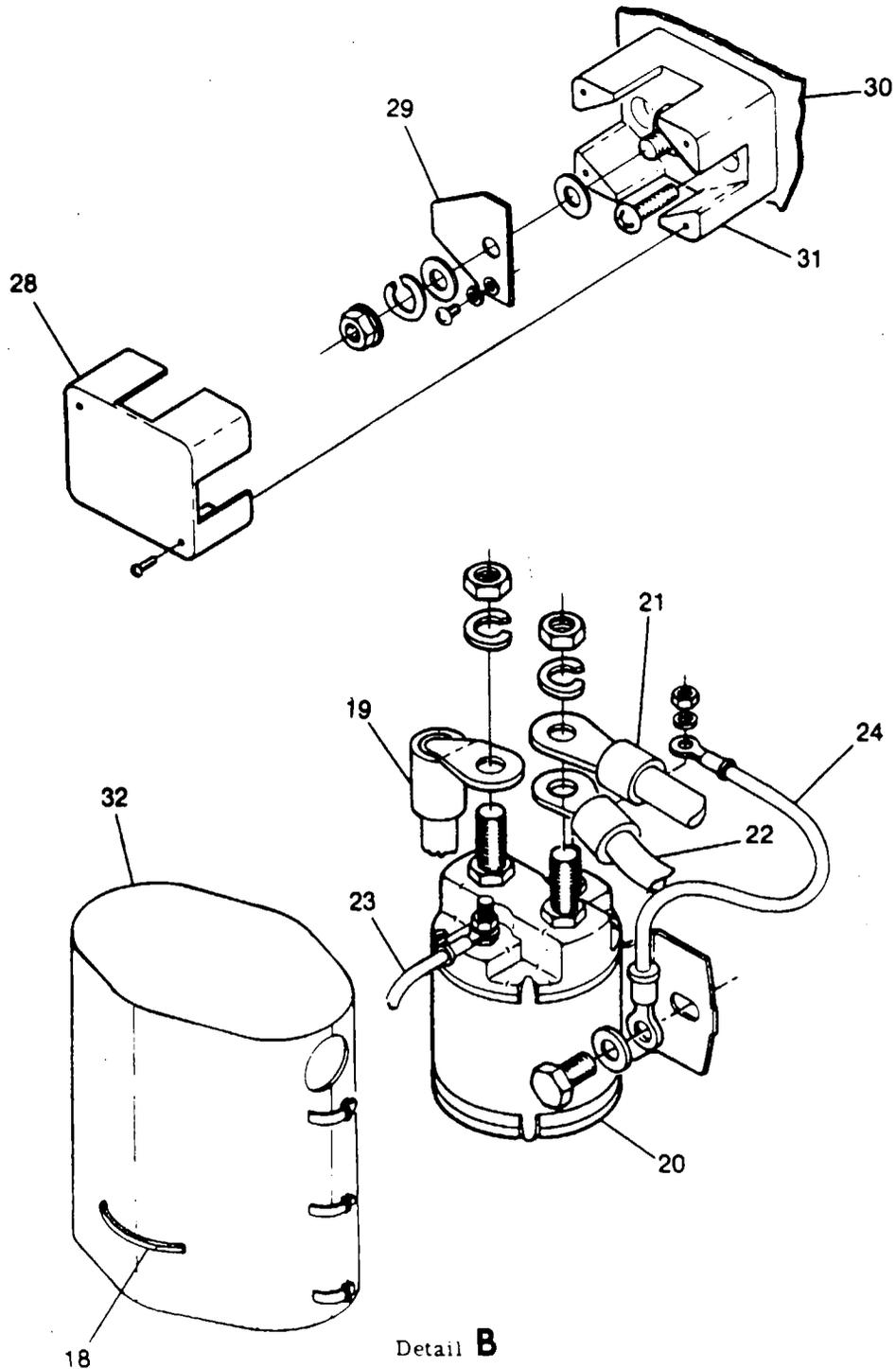
Figure 17-2. Battery and Electrical Equipment Installation (Sheet 4 of 4)
