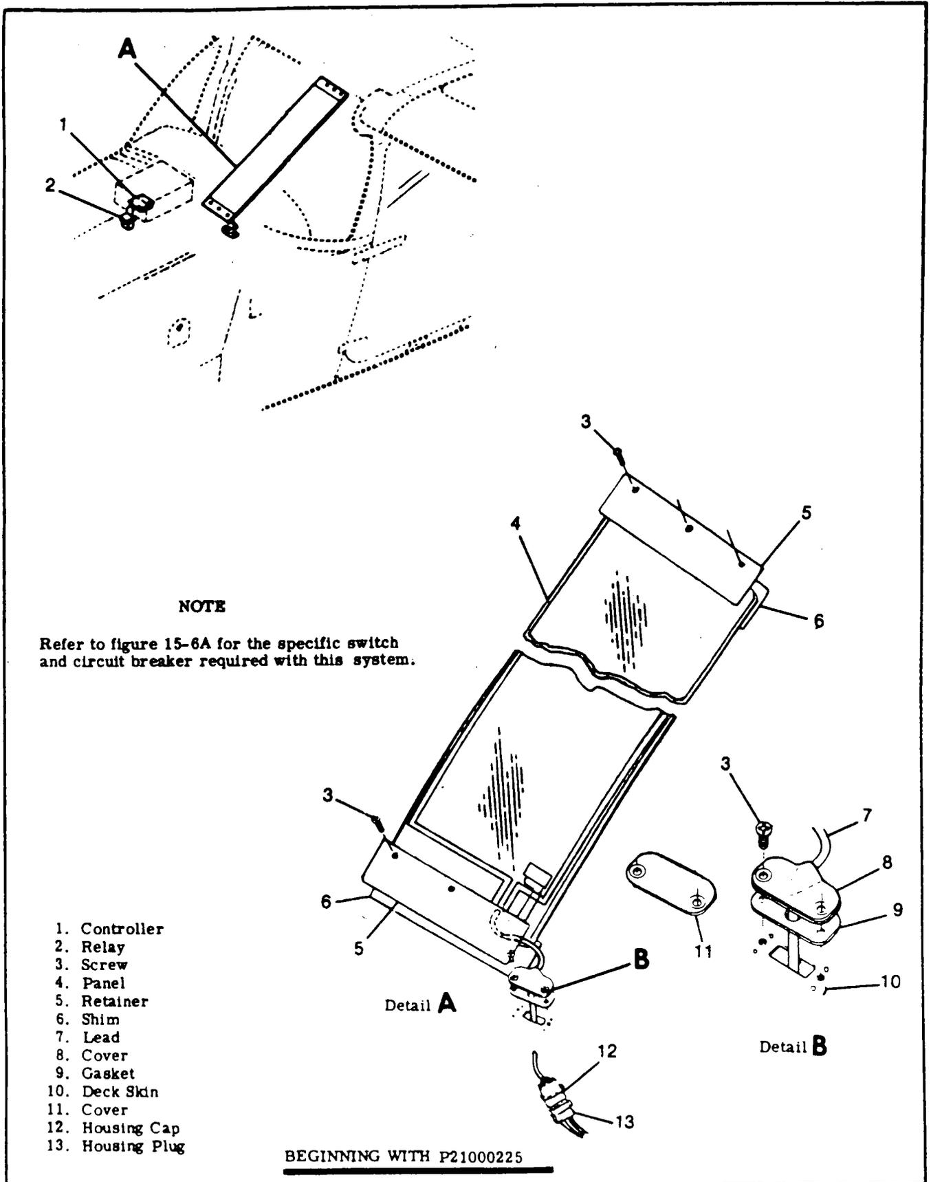
Figure 15-6C. Windshield Anti-Ice Panel Installation (Fixed)
