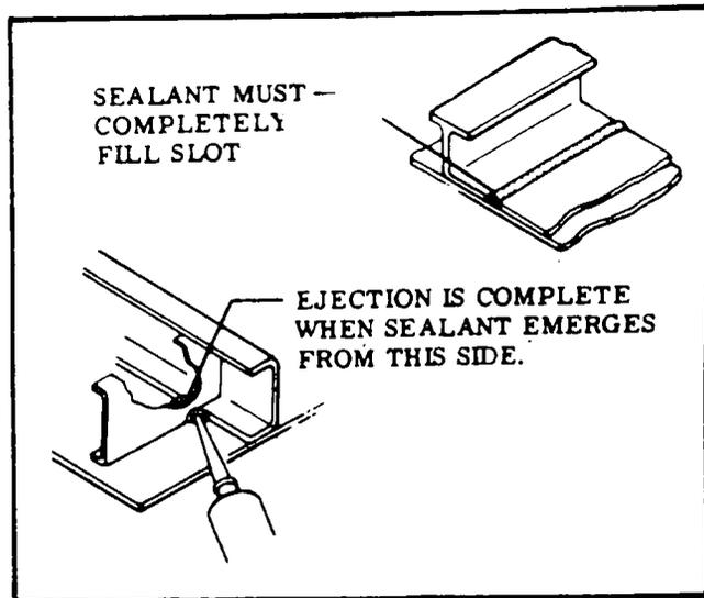
Figure 18-6. Injection Sealing
