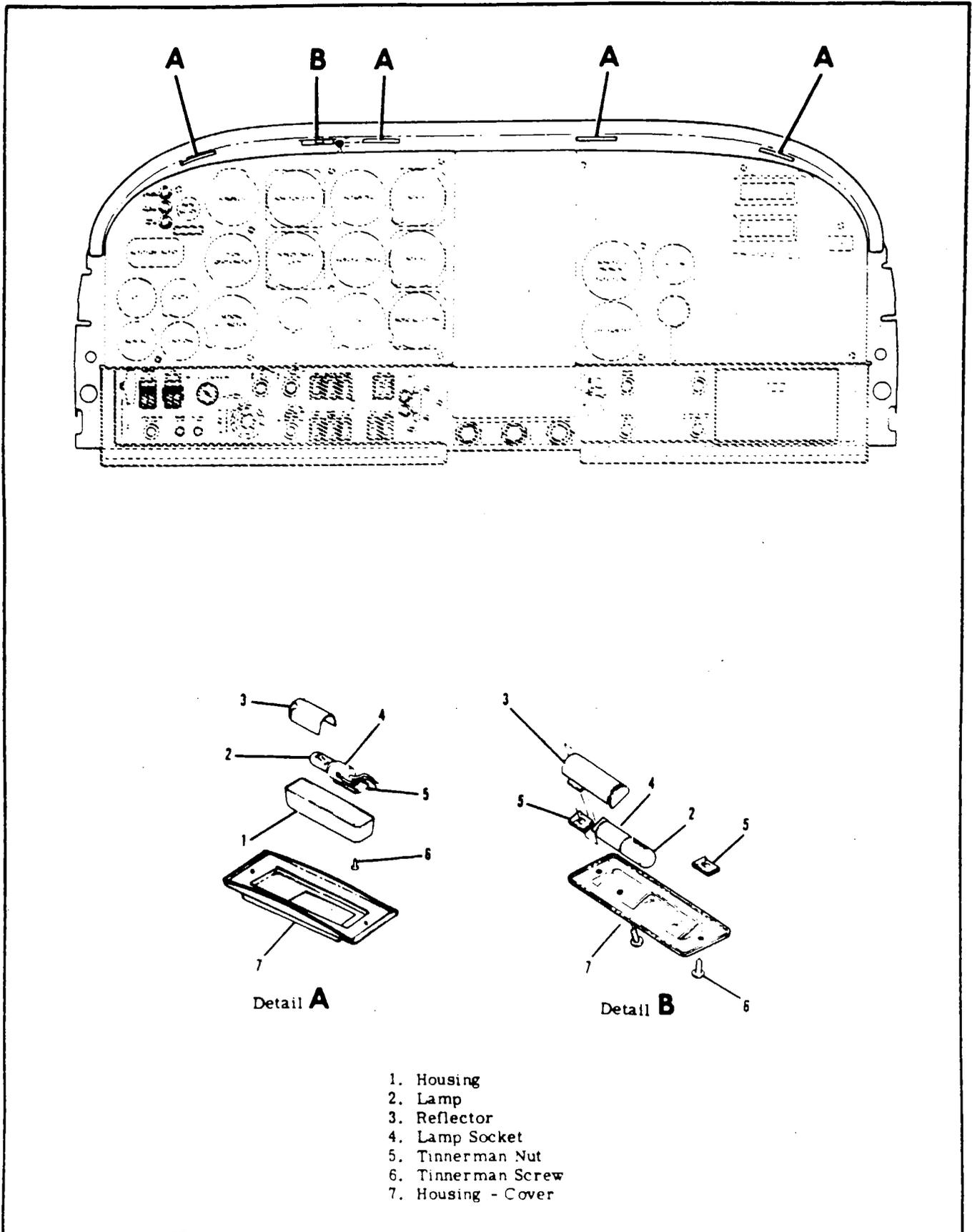
Figure 17-10. Instrument Panel Glare Shield Light Installation
