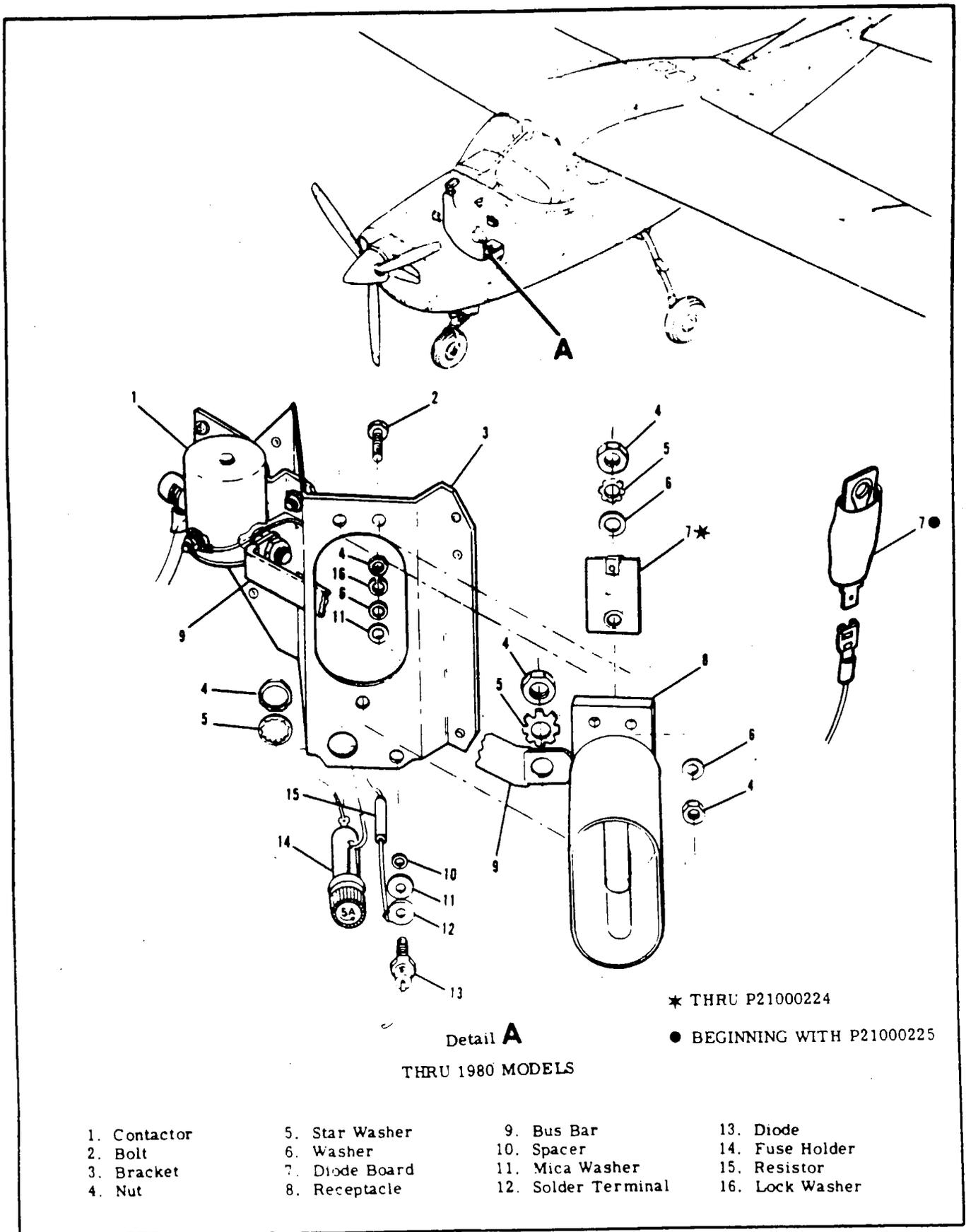
Figure 17-3. Ground Service Receptacle Installation (Sheet 1 of 2)
