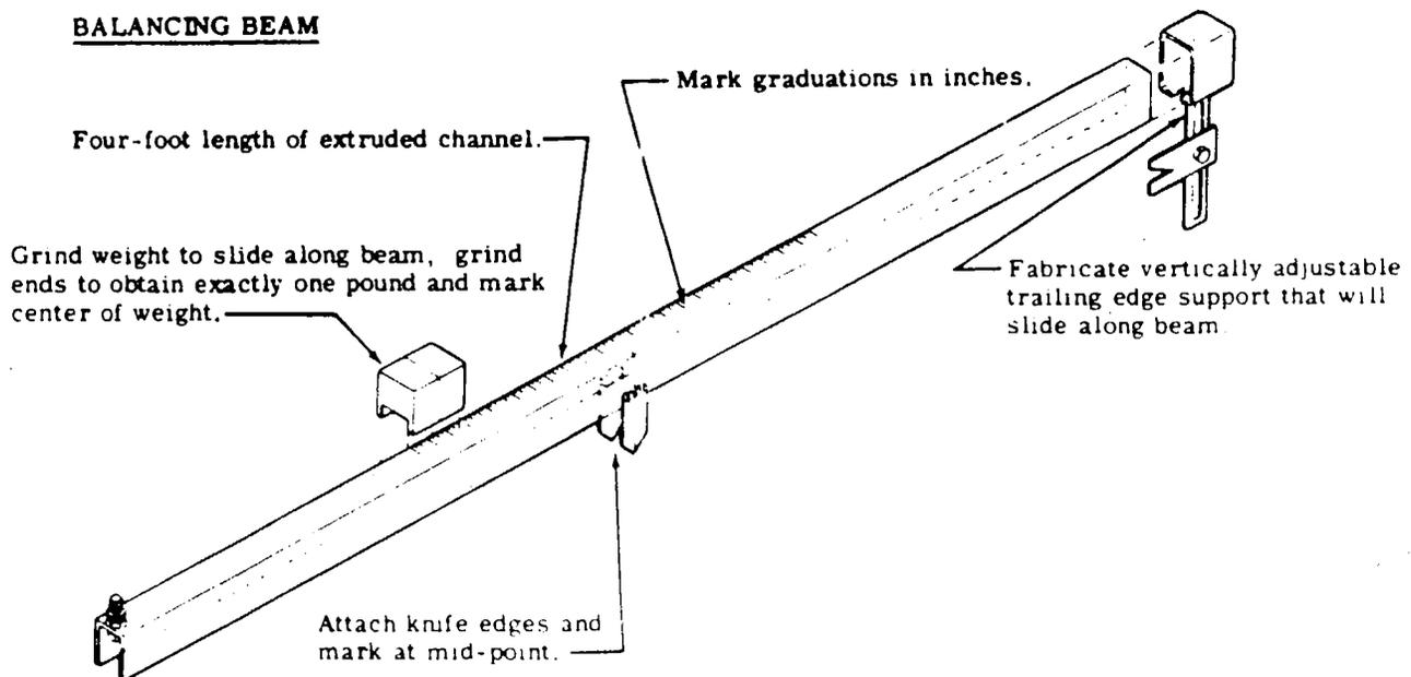
Figure 18-2. Control Surface Balancing (Sheet 3 of 4).
