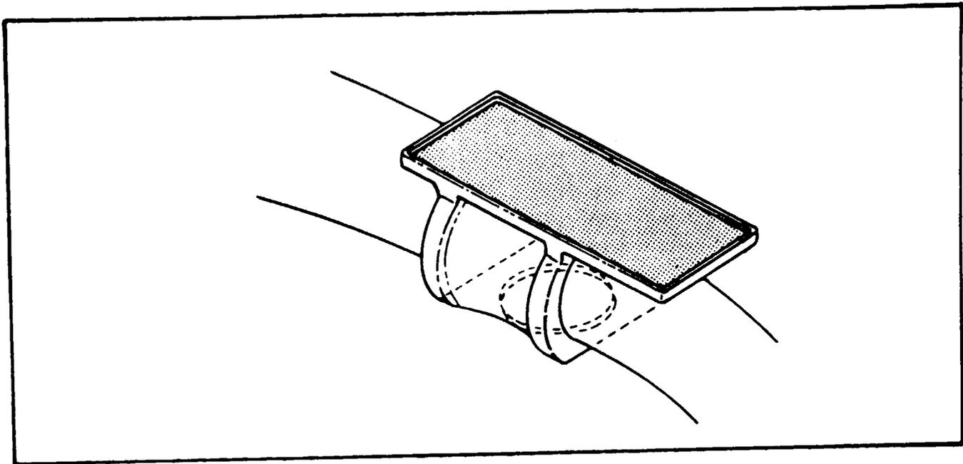
Figure 5-33. Landing Gear Strut Step Installation
