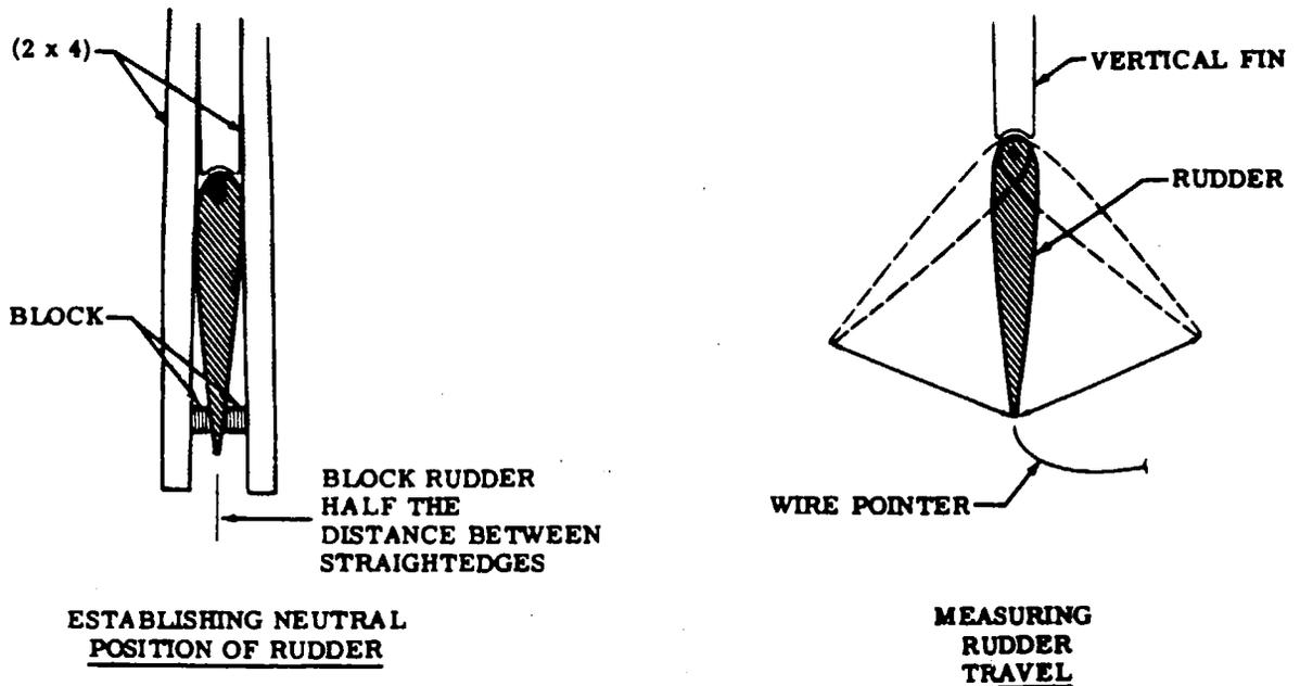
1. Establish neutral position of rudder by clamping straightedge (such as wooden 2 x 4) on each side of fin and rudder and blocking trailing edge of rudder half the distance between straightedges as shown.
