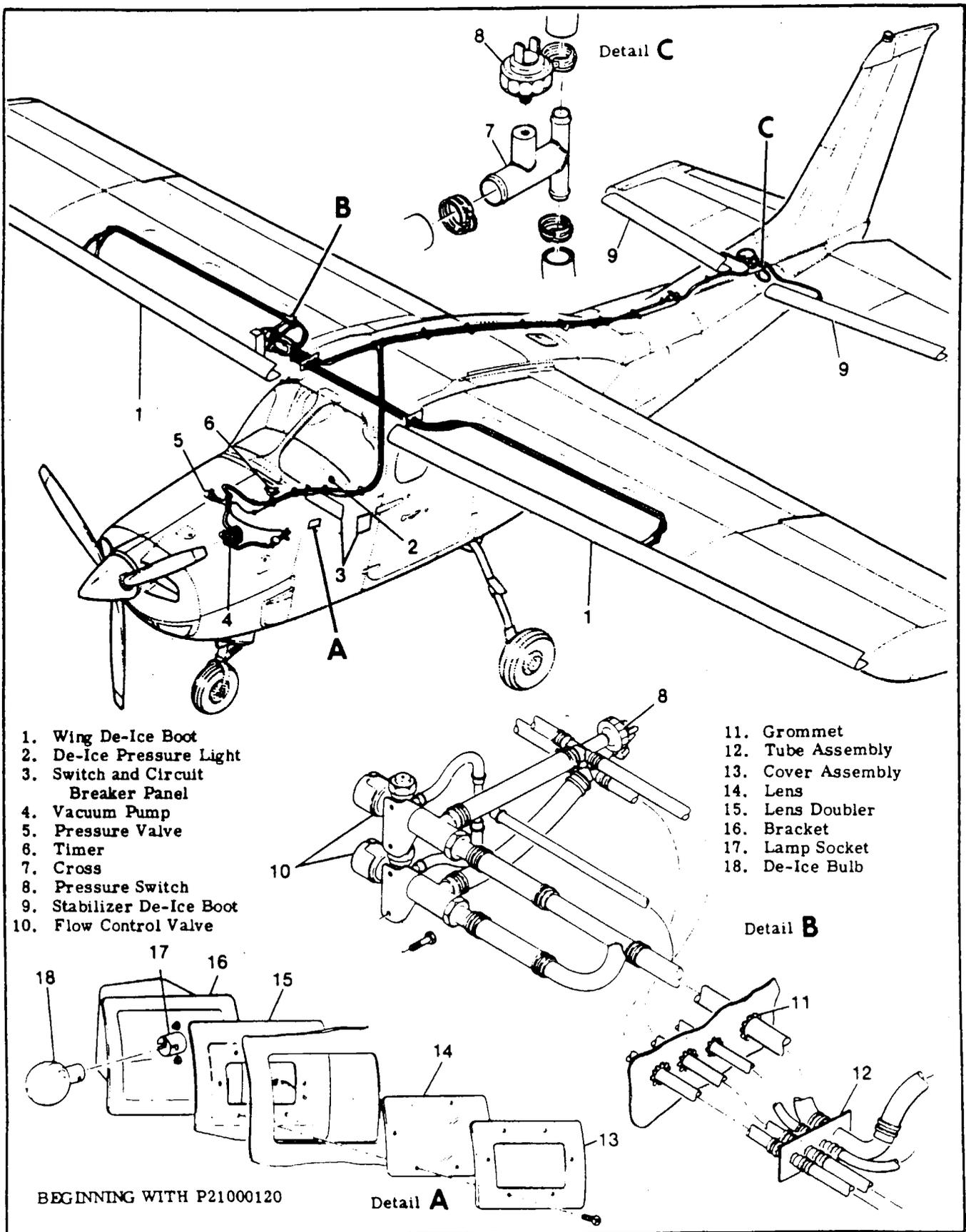
Figure 15-4. Wing and Horizontal Stabilizer Three-Cycle De-ice System
