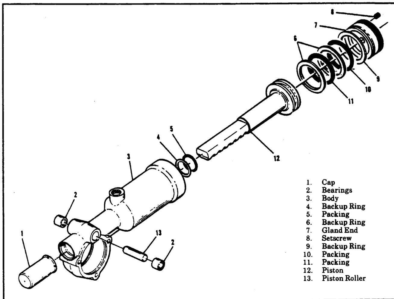
Figure 5A-12. Main Landing Gear Actuator
