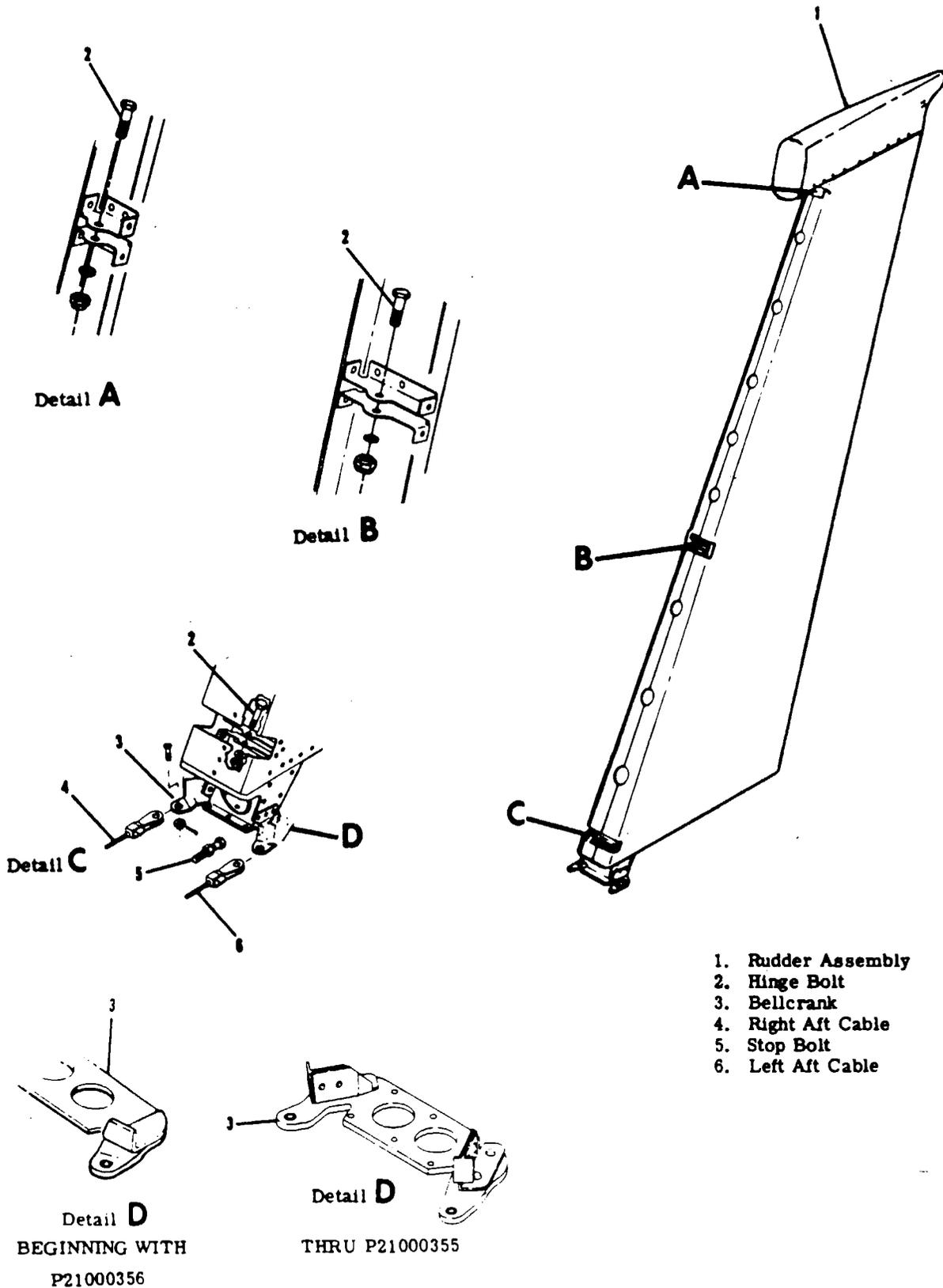
Figure 10-4. Rudder Installation
