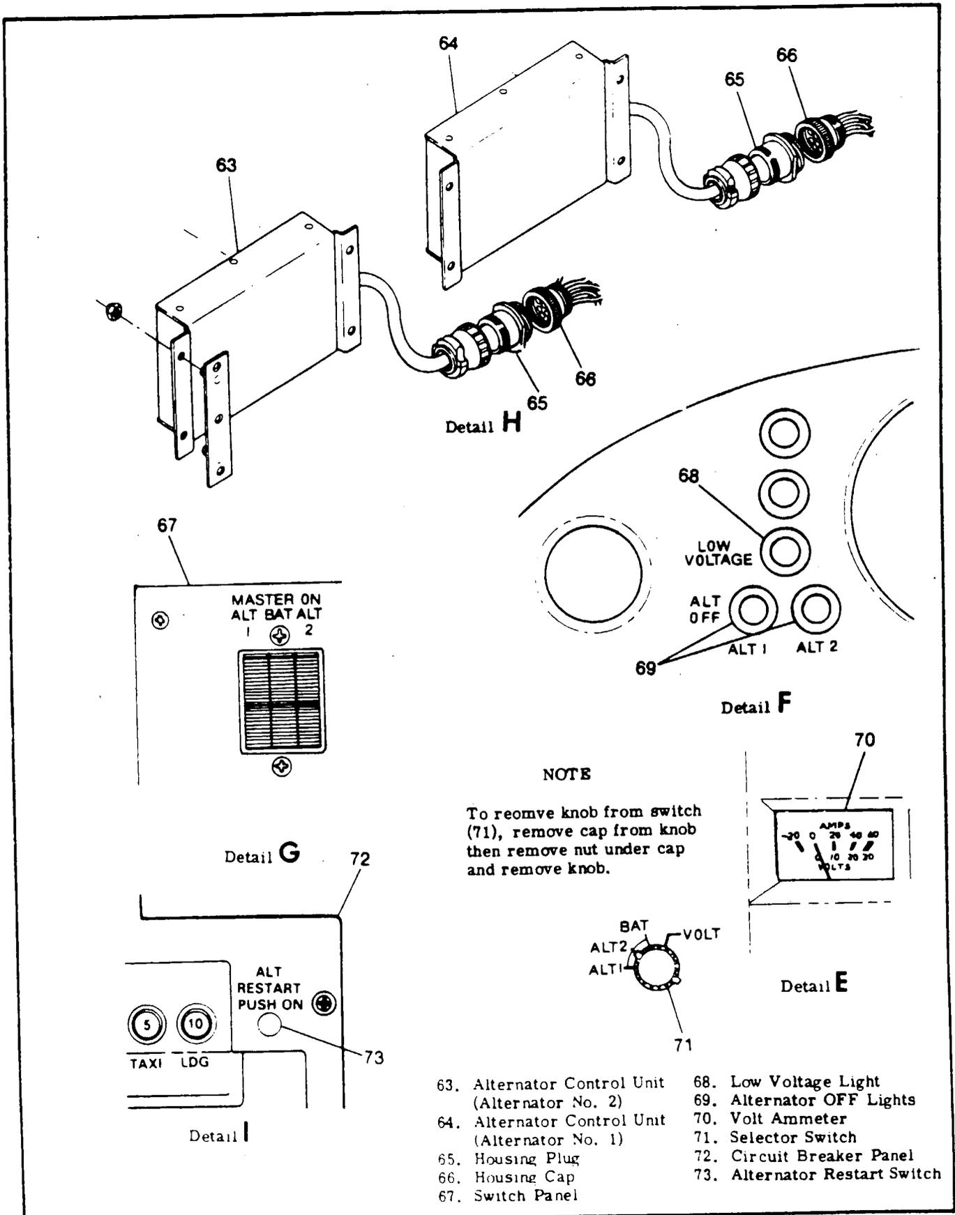
Figure 17-6B. Dual Alternator System Installation (Sheet 7 of 8)
