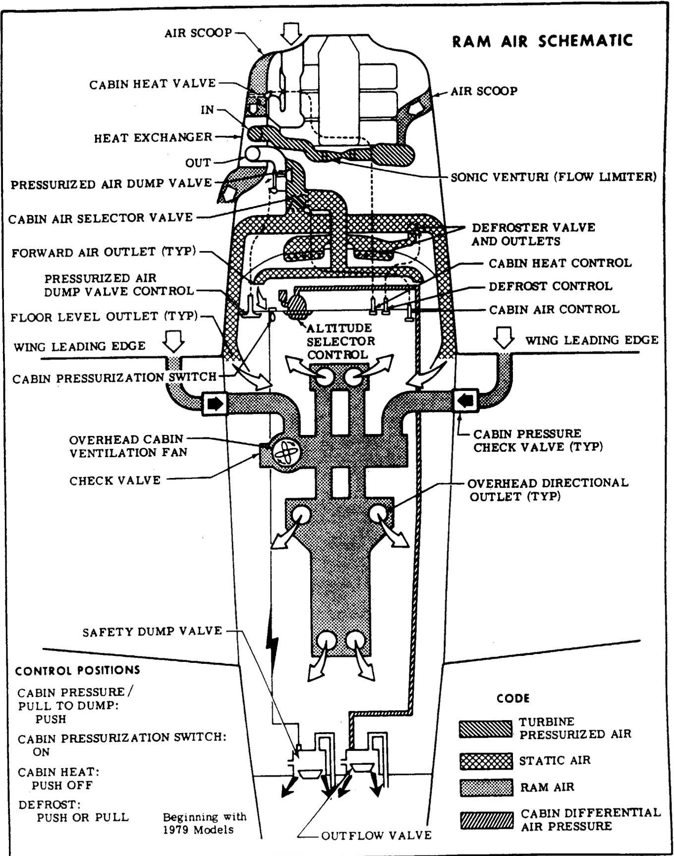
Figure 15-2. Cabin Air Flow Schematic (Sheet 4 of 6)
