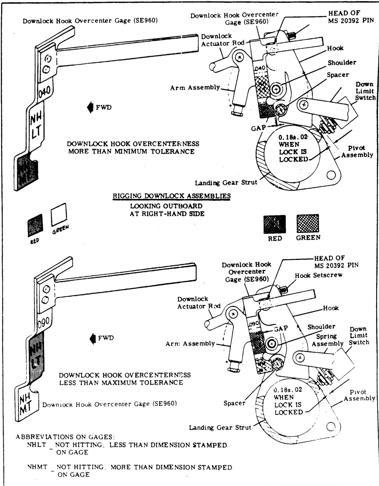
Figure 5A-10. Rigging Main Landing Gear (Sheet 2 of 3)
