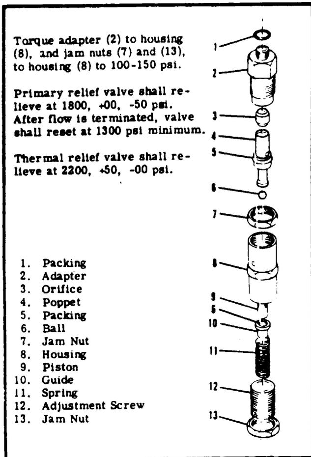
Figure 5A-4. Relief Valve Assembly
