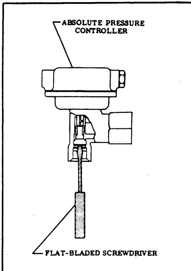
Figure 12-18. Controller Adjustment
