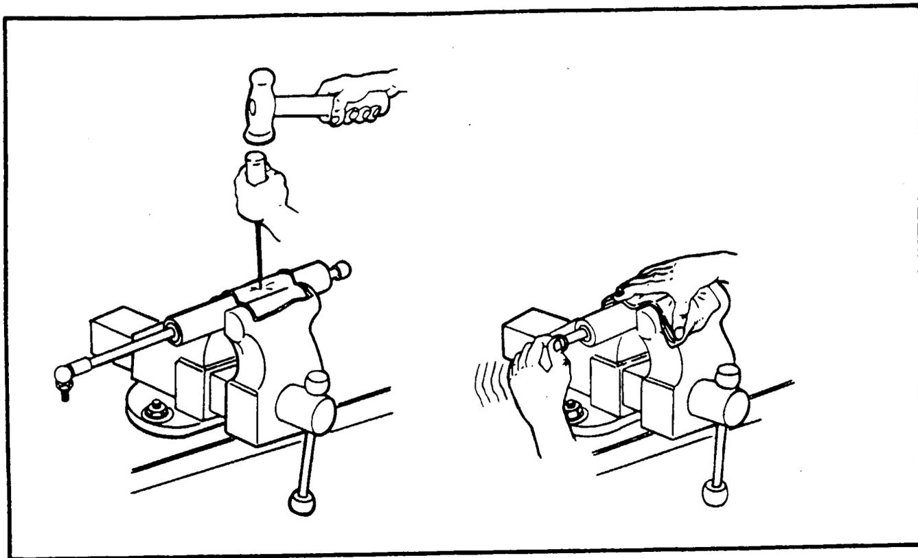
Figure 3-6A. Disposal of Gas Spring Assembly
