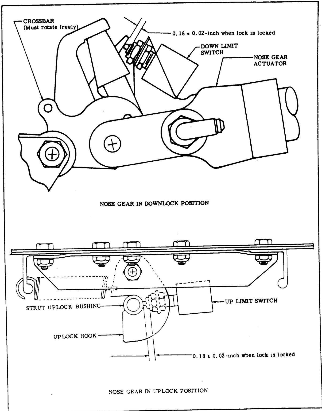
Figure 5-37. Rigging Nose Landing Gear
