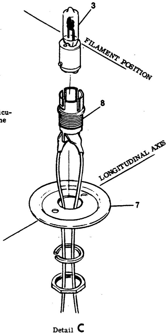
Figure 17-9. Flashing Beacon Installation (Sheet 2 of 2)
