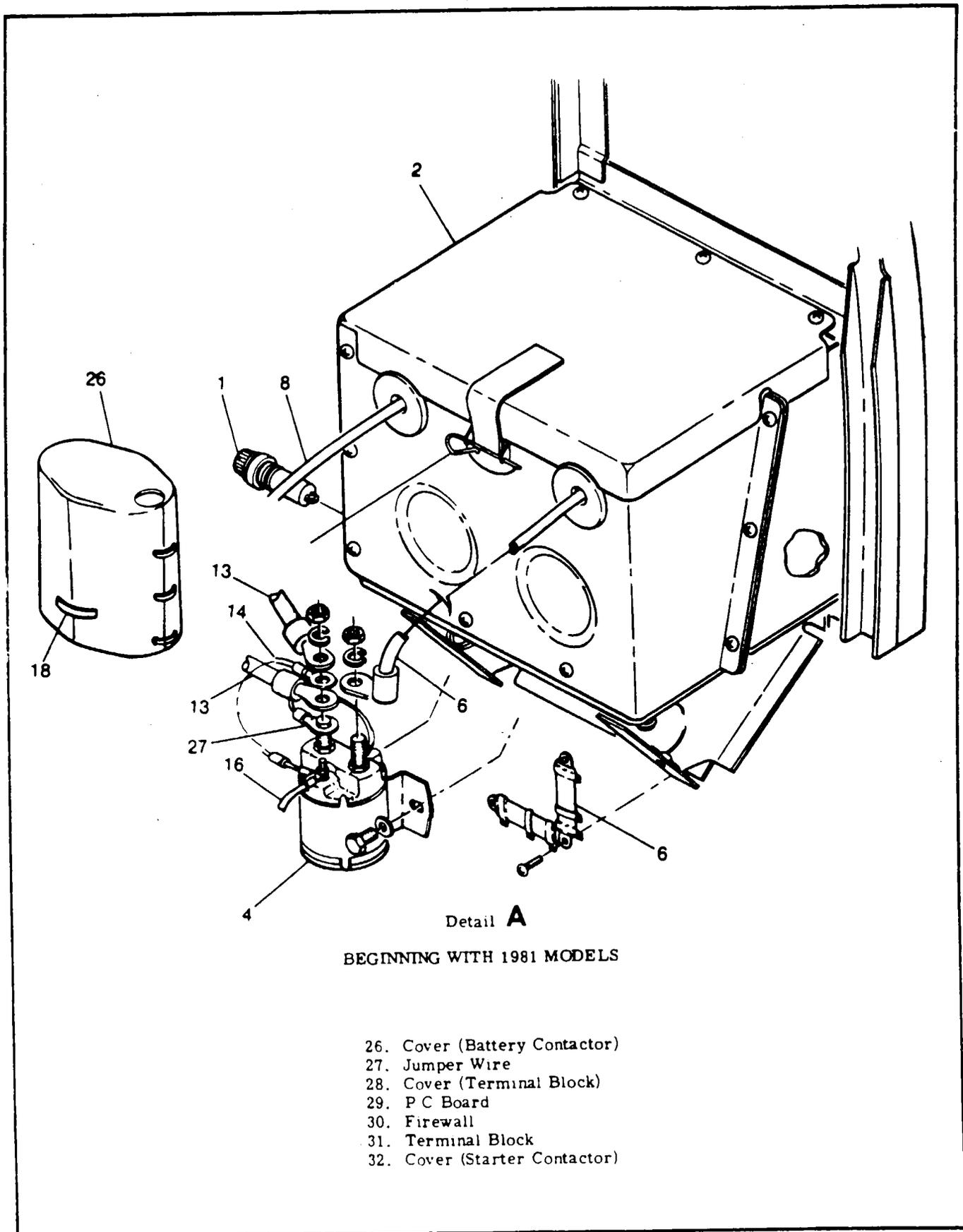
Figure 17-2. Battery and Electrical Equipment Installation (Sheet 3 of 4)
