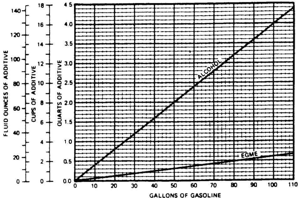
Figure 2-3. Fuel Additive Mixing Ratio Chart
