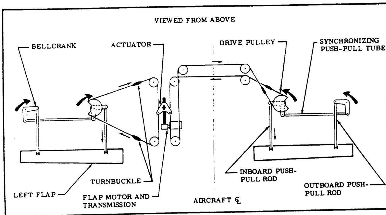
Figure 7-3. Flap System Schematic
