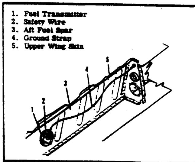
Figure 16-6. Fuel Transmitter Installation
