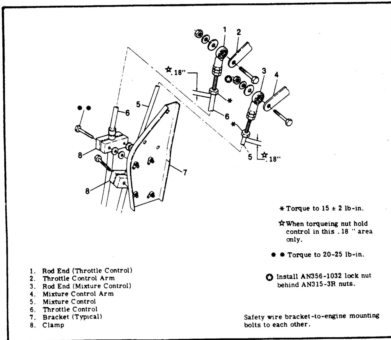
Figure 12-12. Engine Controls
