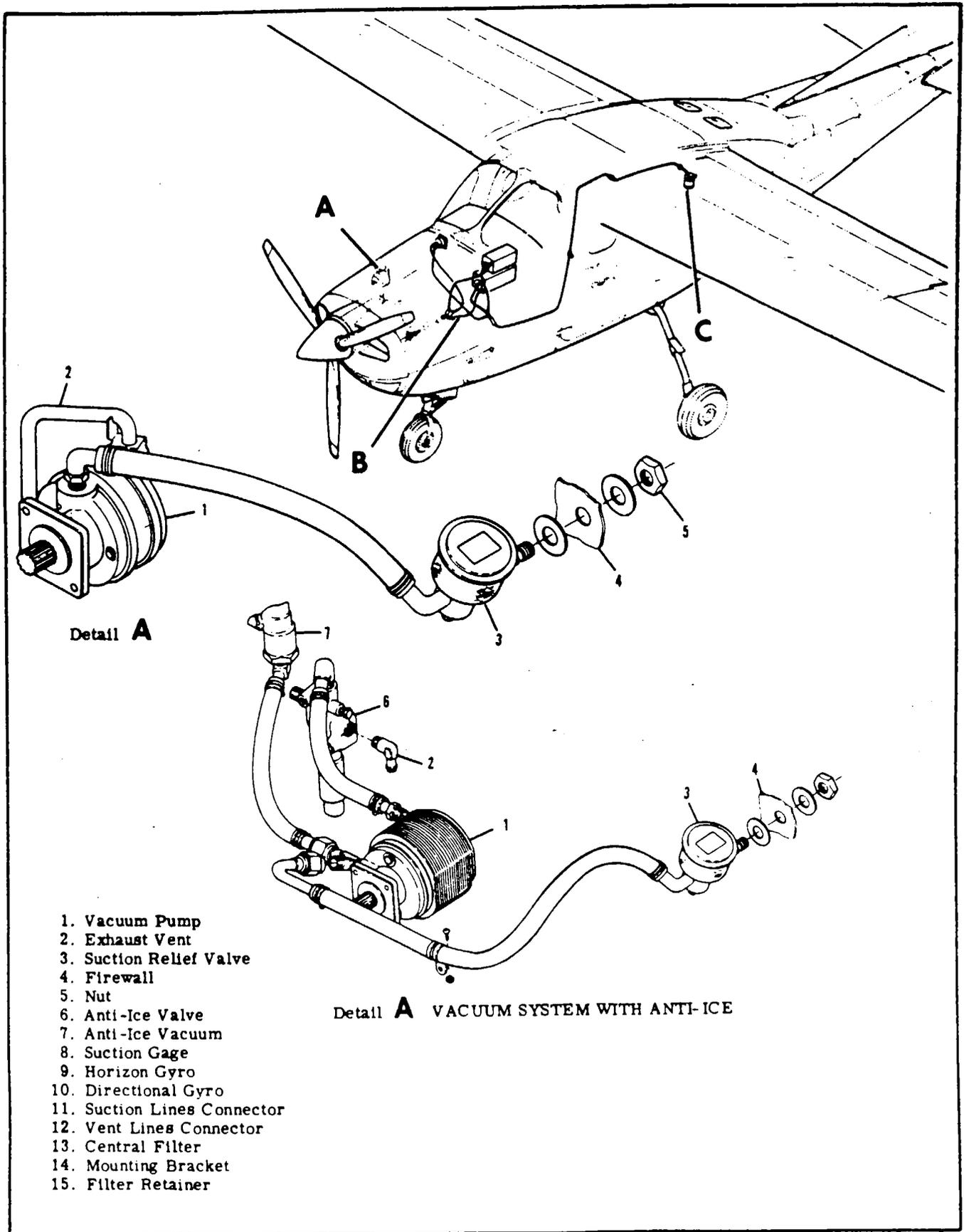
Figure 16-4. Vacuum System (Sheet 1 of 3)
