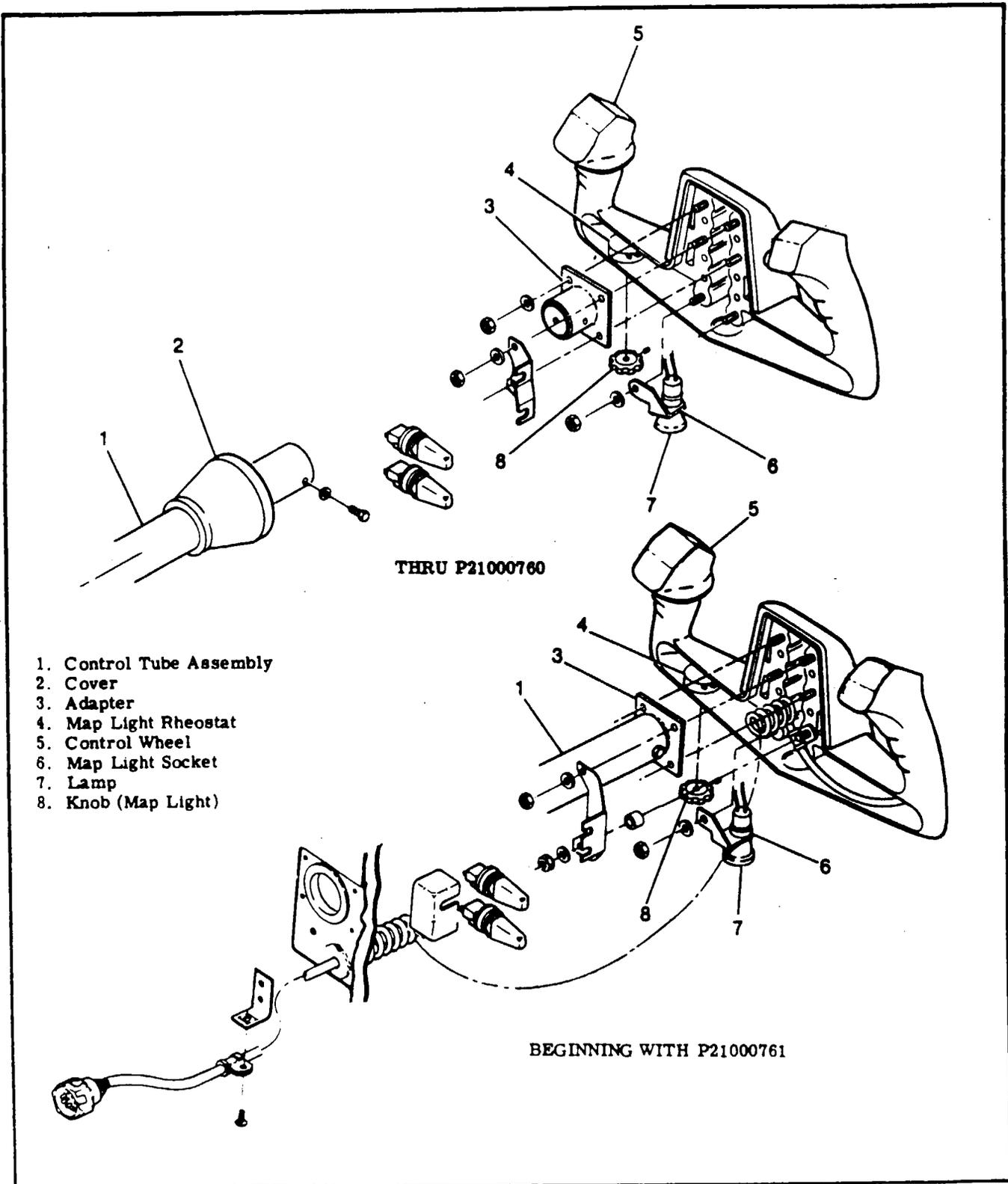
Figure 17-14. Control Wheel Map Light Installation
