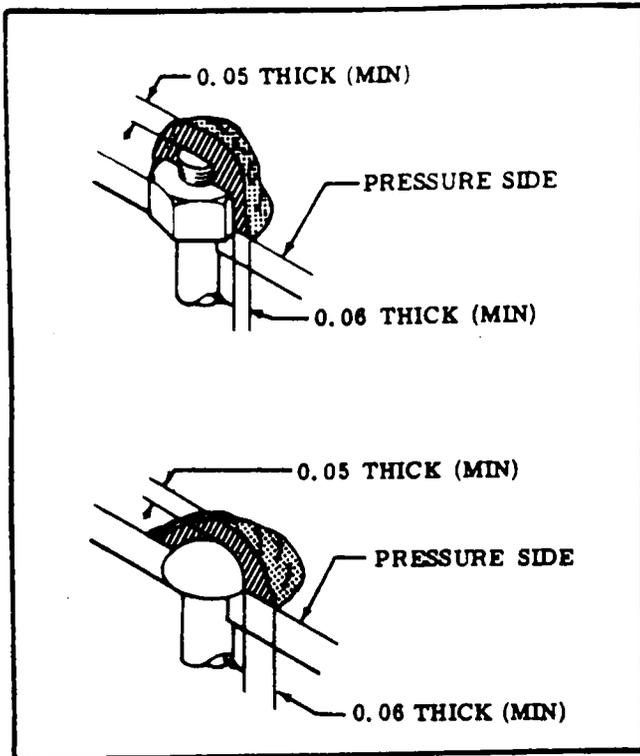
Figure 18-8. Fastener Sealing
