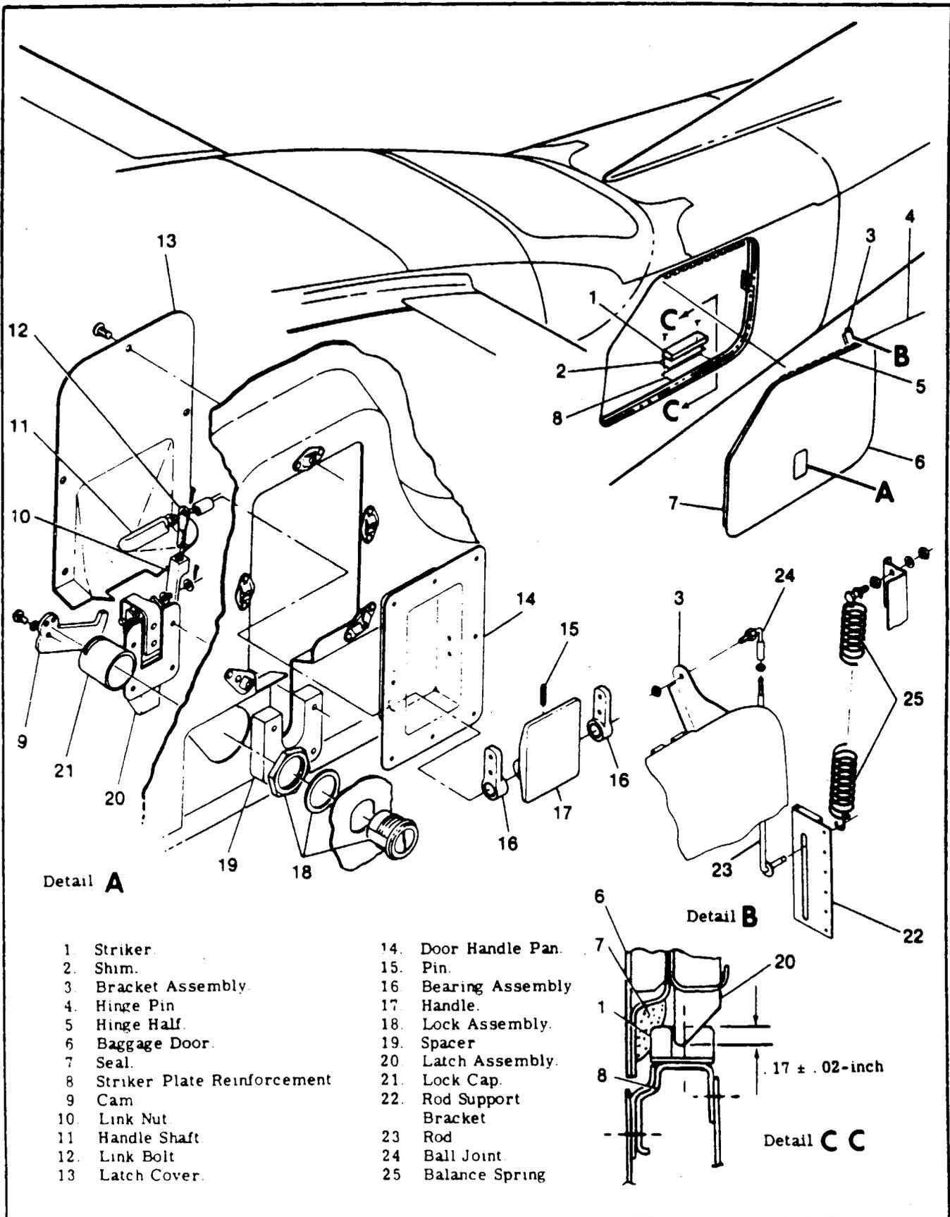
Figure 3-7A. Baggage Door Installation
