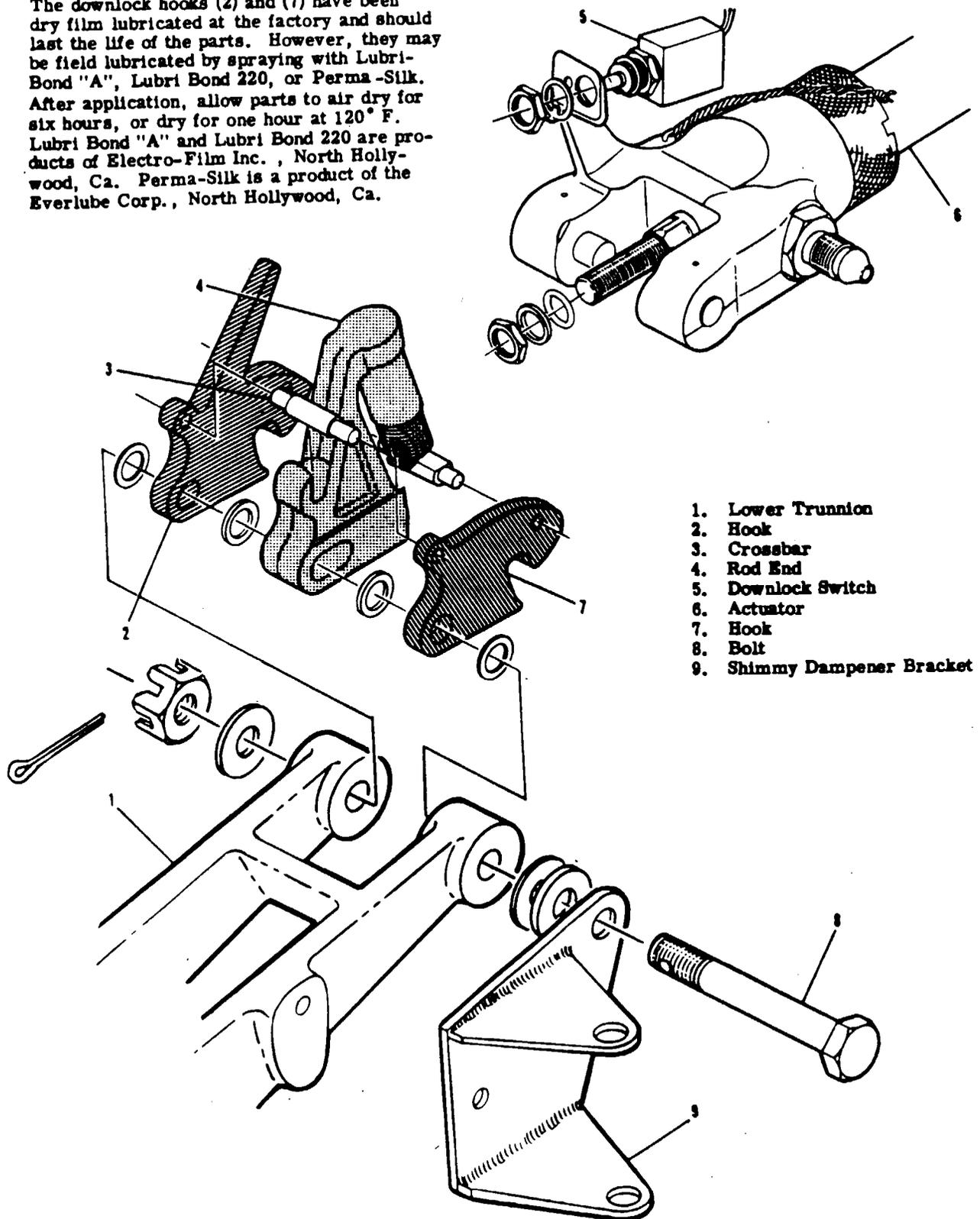
Figure 5-20. Nose Gear Downlock Mechanism
