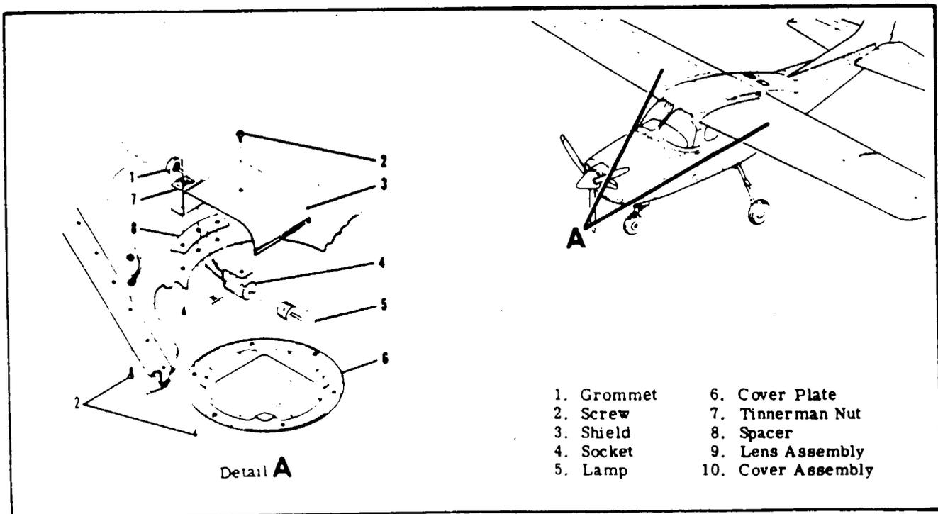
Figure 17-13. Courtesy Light Installation
