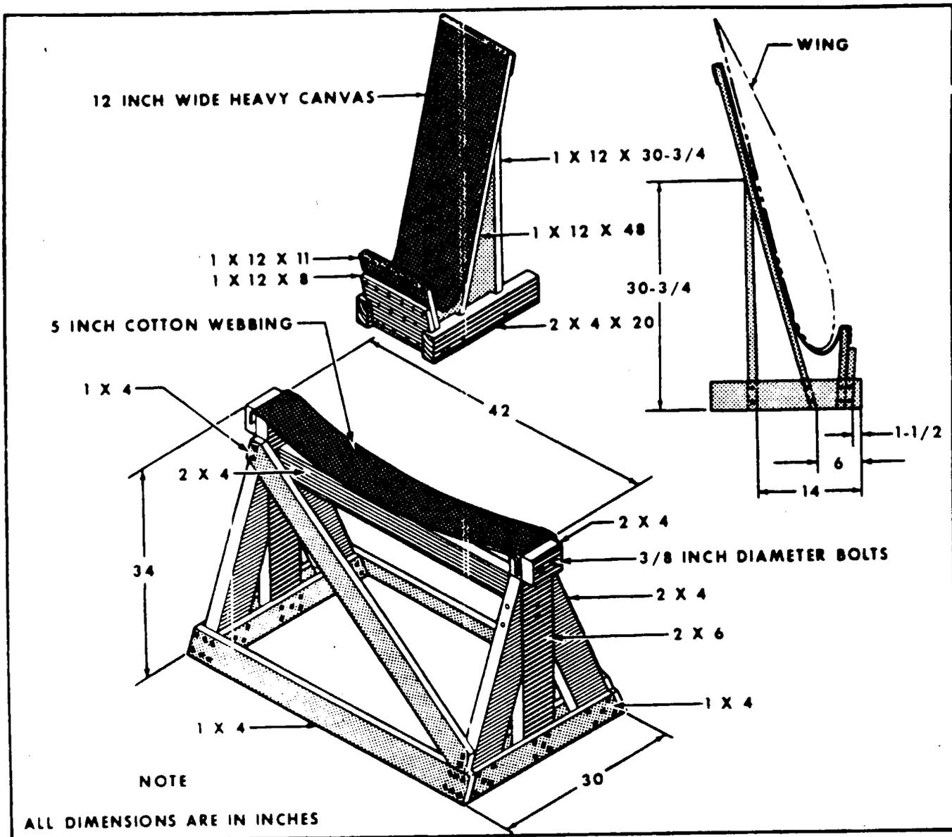
Figure 18-1. Wing and Fuselage Support Stands
