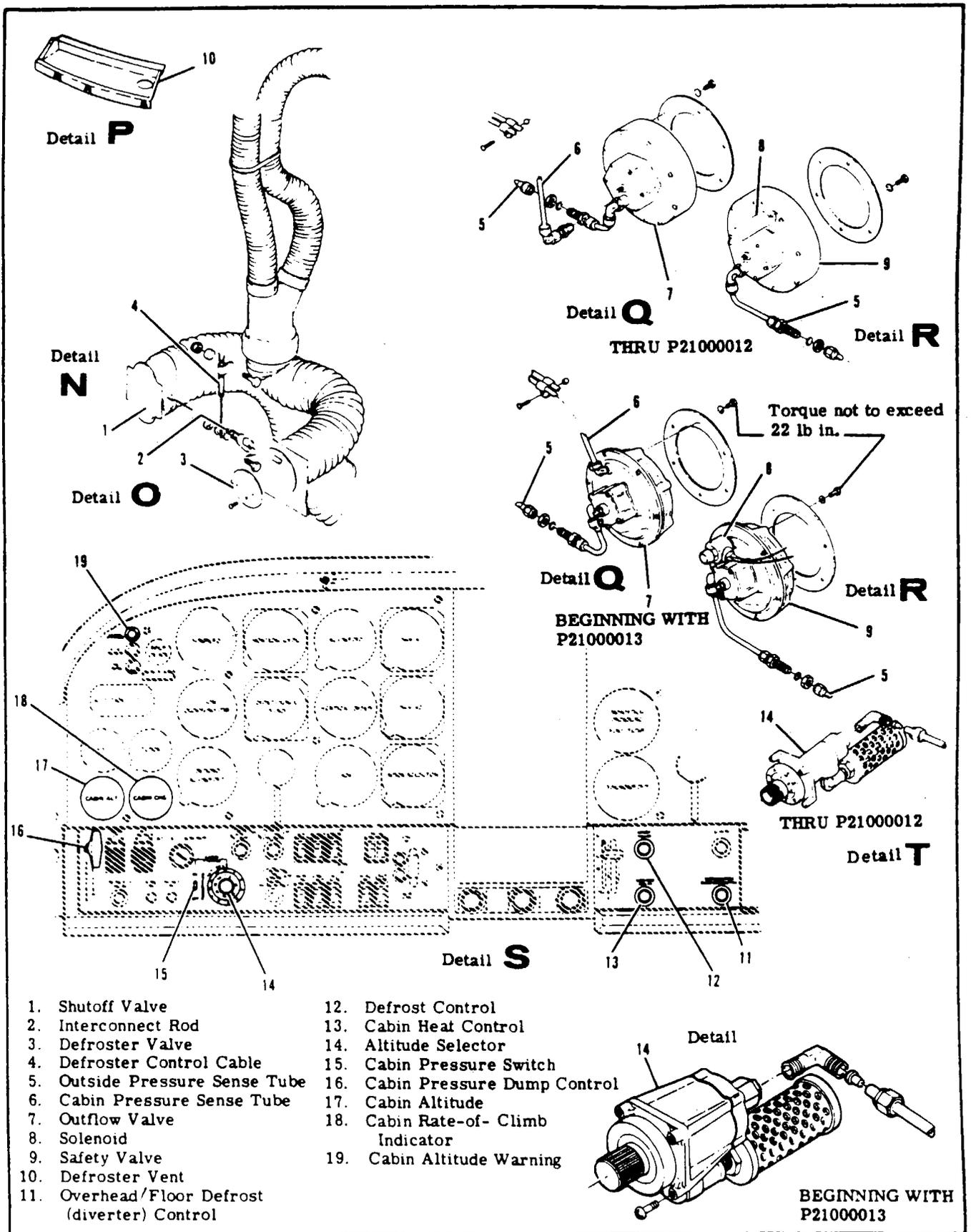
Figure 15-1. Heating, Ventilating and Pressurization System (Sheet 5 of 5)
