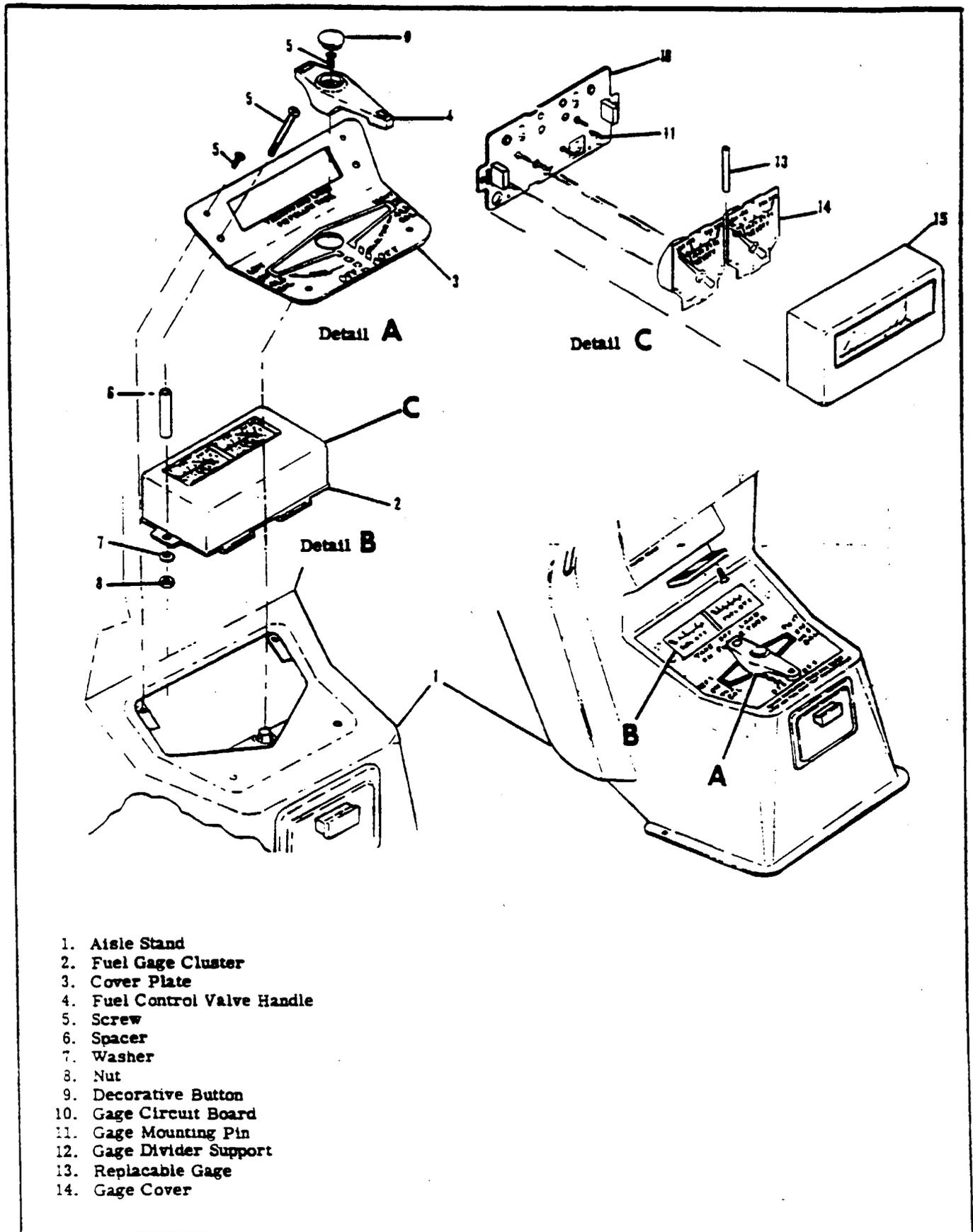
Figure 16-5. Fuel Gage Installation
