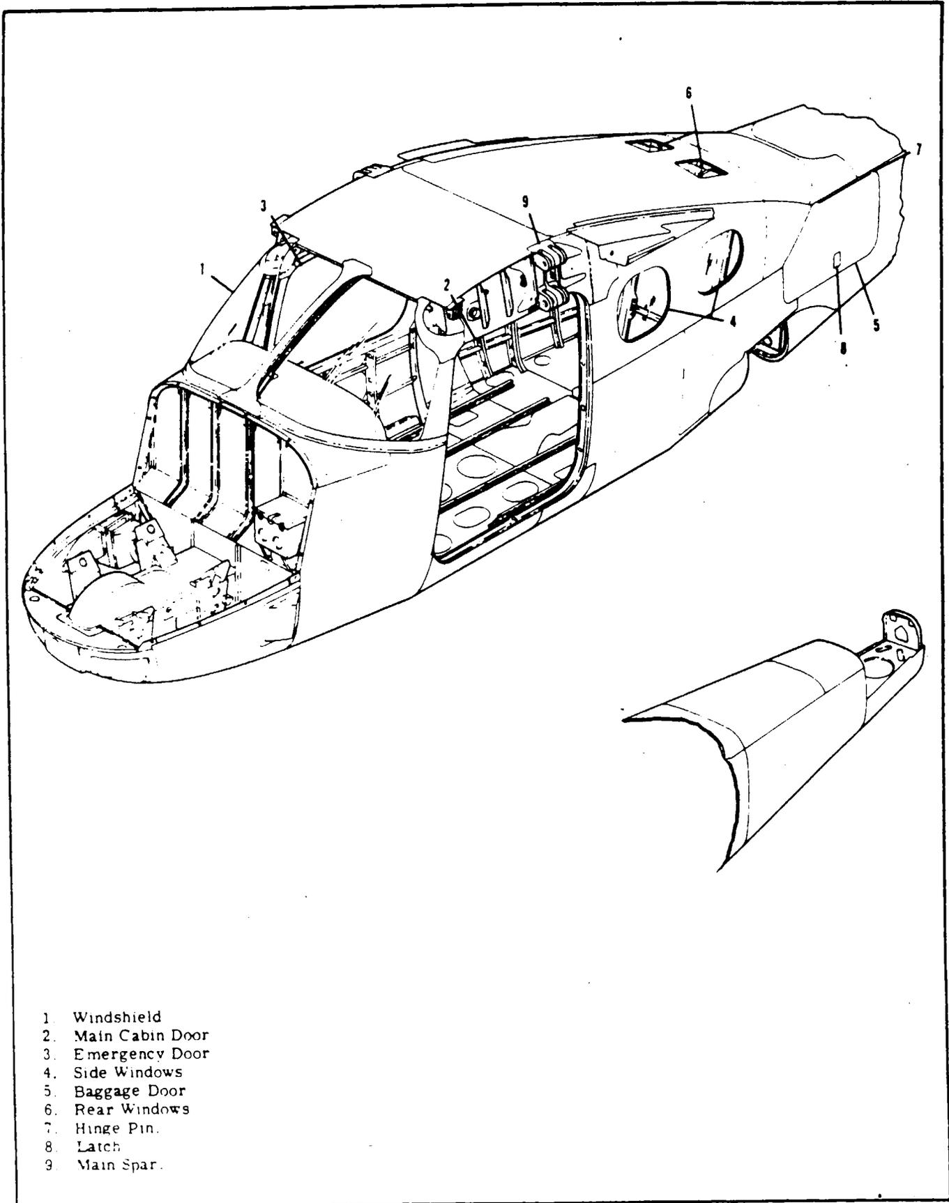
Figure 3-1 A. Fuselage Assembly.
