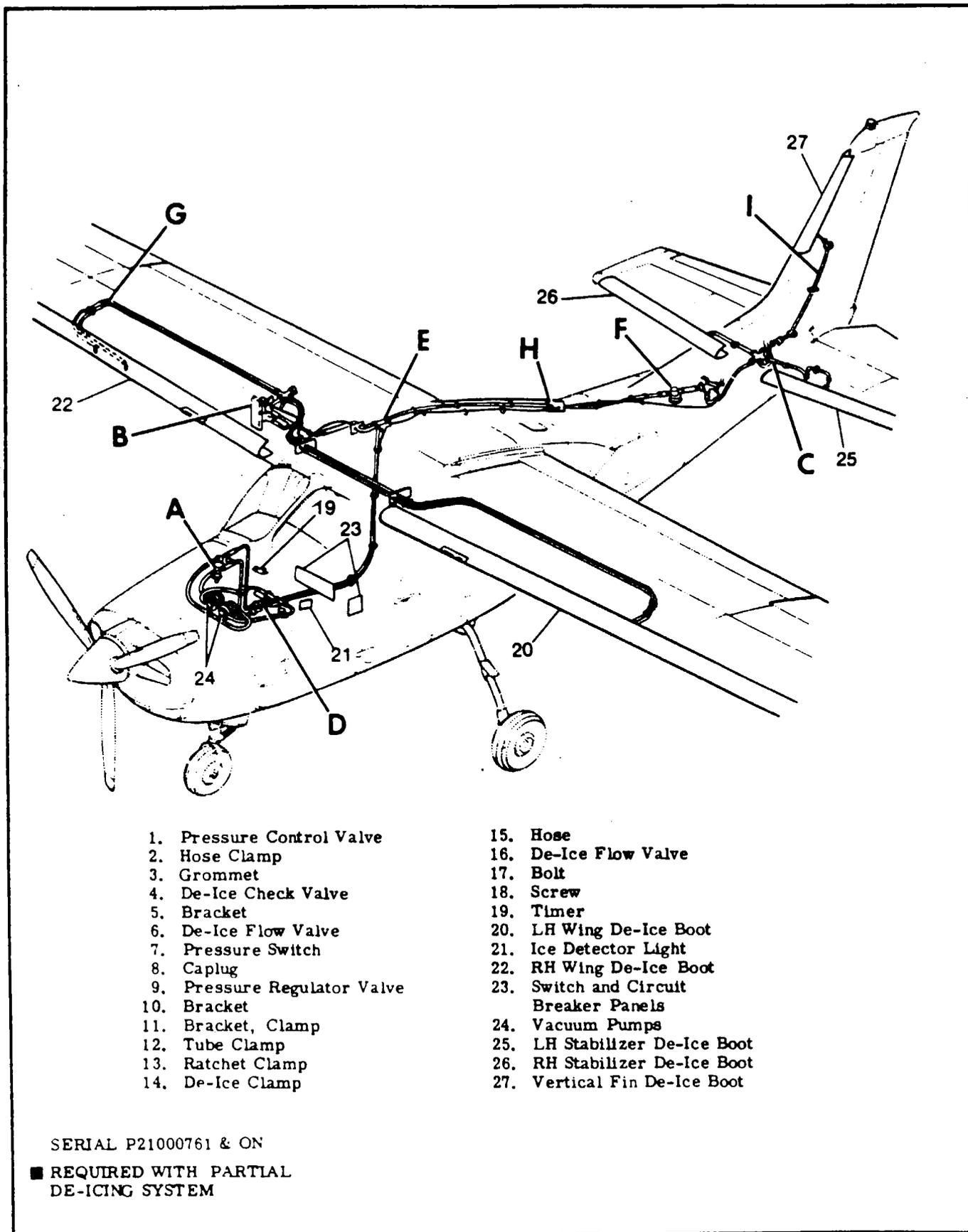
Figure 15-4A. Wing, Horizontal Stabilizer and Vertical Fin De-Icing System (Sheet 3 of 5)
