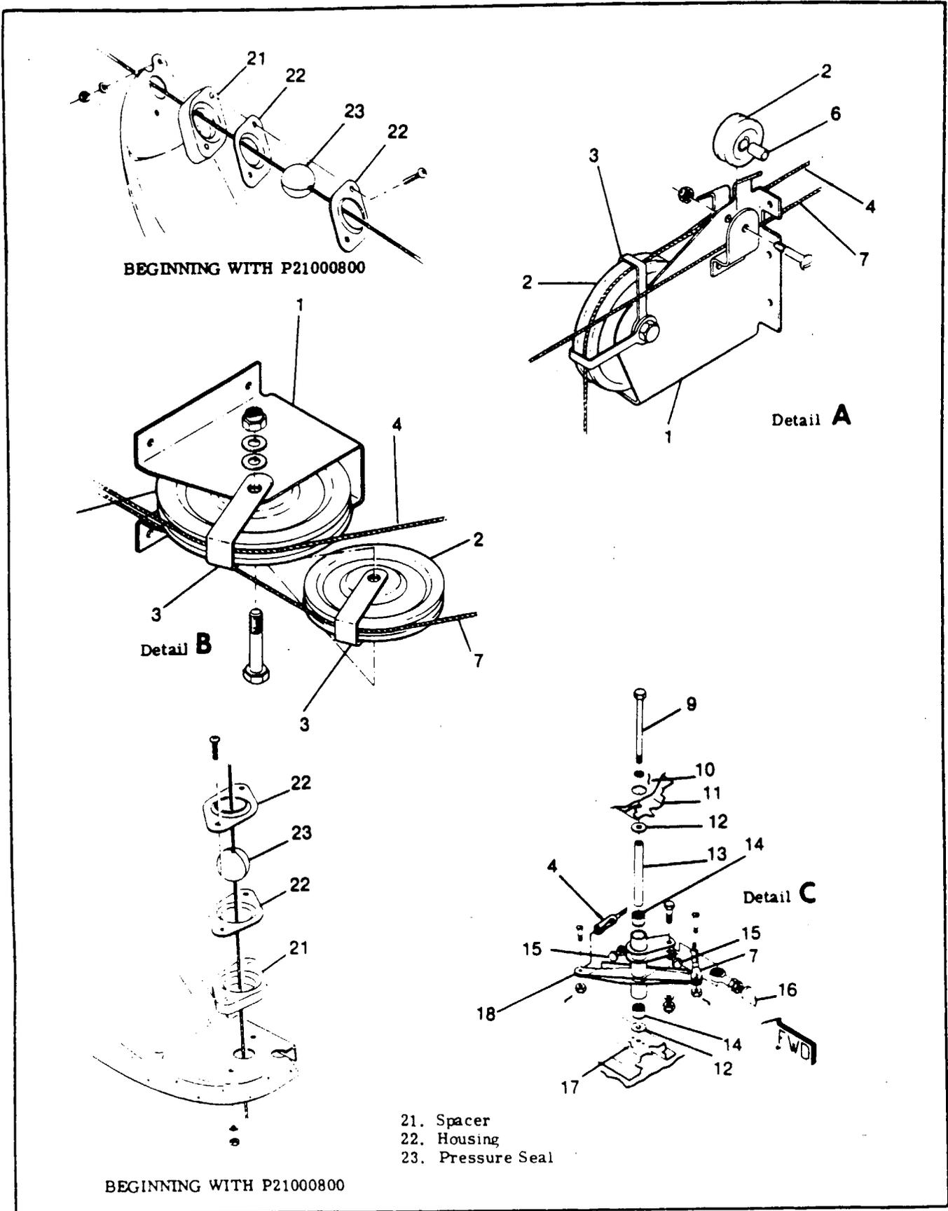
Figure 6-1. Aileron Control System (Sheet 2 of 2)
