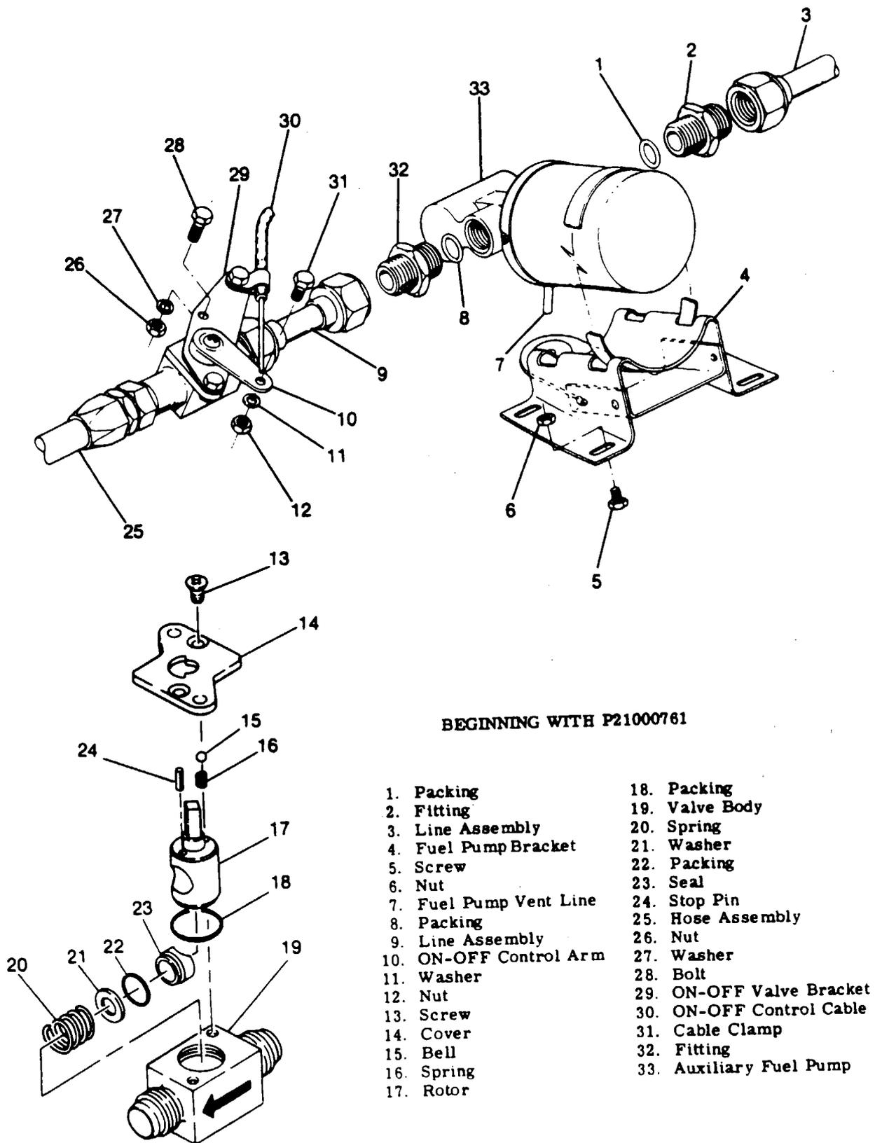
Figure 13-14. Auxiliary Fuel Pump and ON-OFF Valve.
