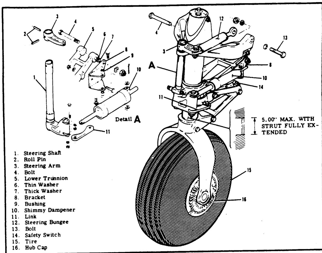
Figure 5-15. Nose Gear Installation
