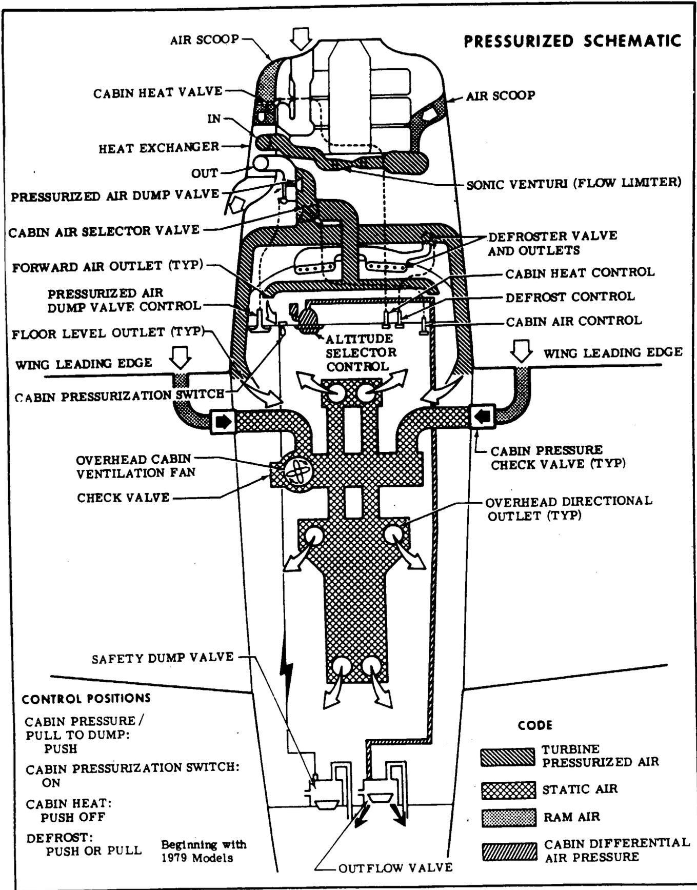
Figure 15-2. Cabin Air Flow Schematic (Sheet 5 of 6)
