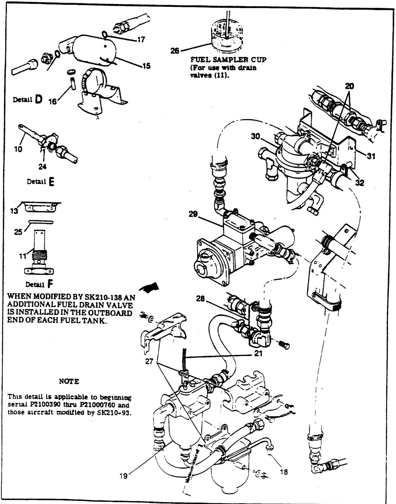
Figure 13-2. Fuel System (Sheet 3 of 4)
