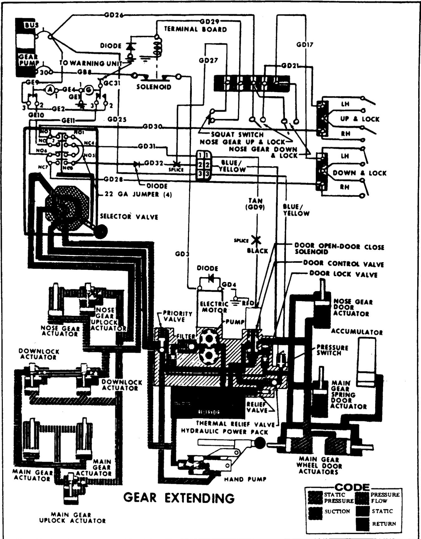
Figure 5-38. Hydraulic and Electrical System Schematic (Sheet 4 of 7)
