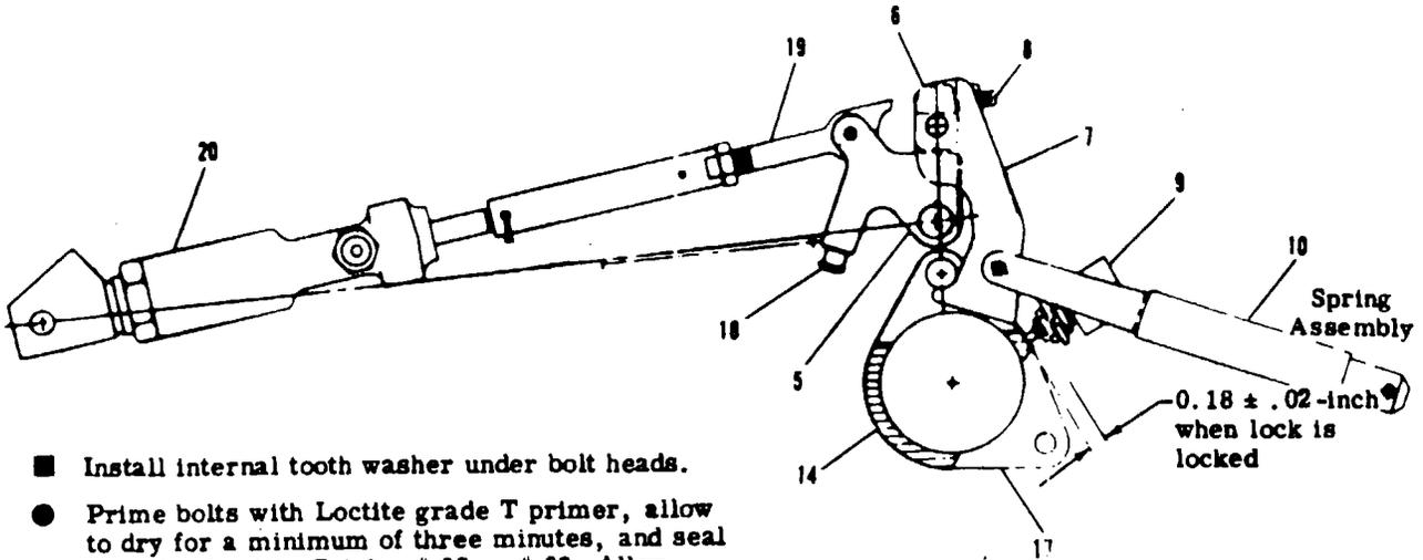
■ Install internal tooth washer under bolt heads.
