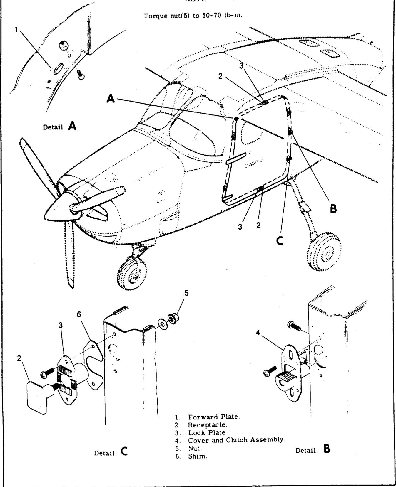
Figure 3-5A. Main Door Receptacle Installation (Sheet 1 of 2).
