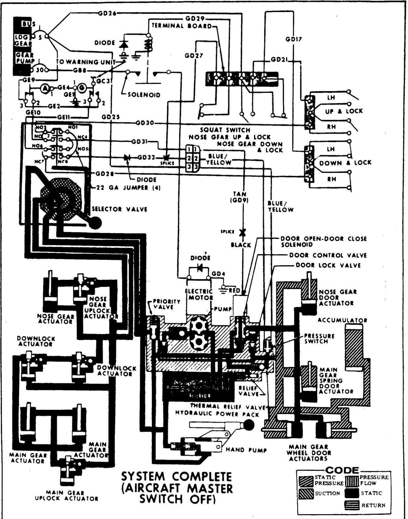
Figure 5-38. Hydraulic and Electrical System Schematic (Sheet 7 of 7)
