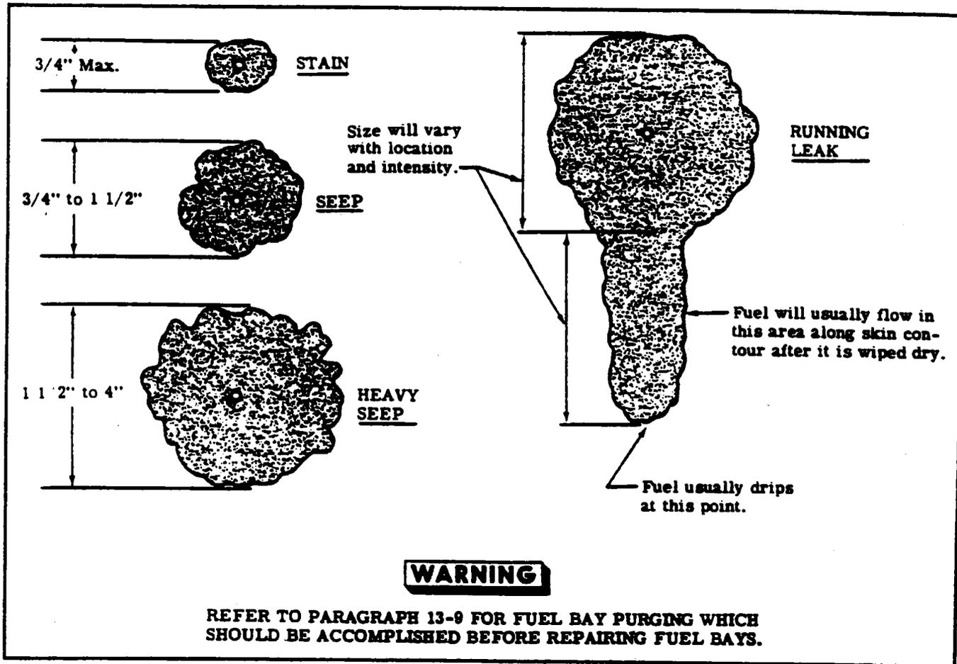
Figure 13-3. Classification of Fuel Leaks.
