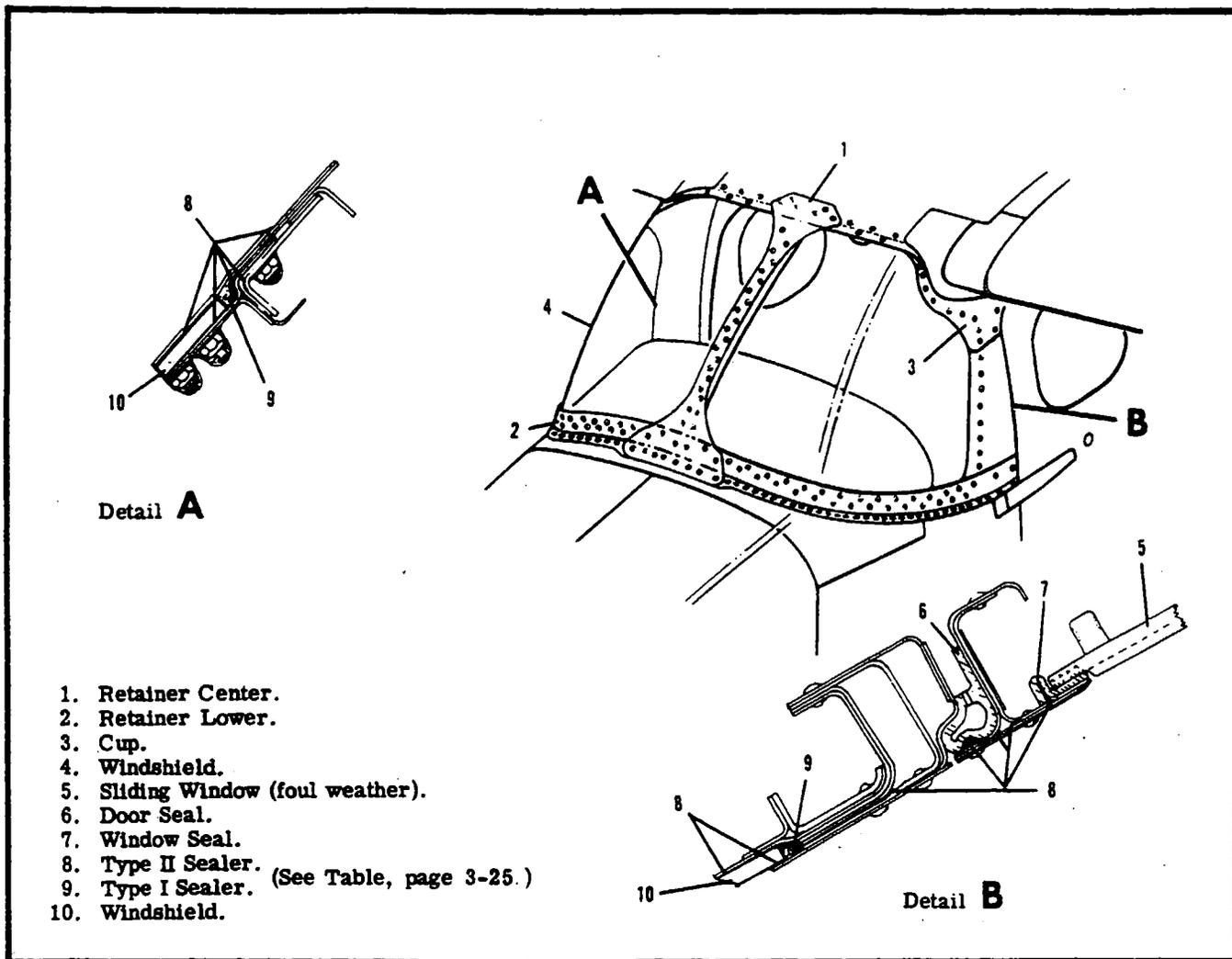
Figure 3-2. Windshield Installation.
