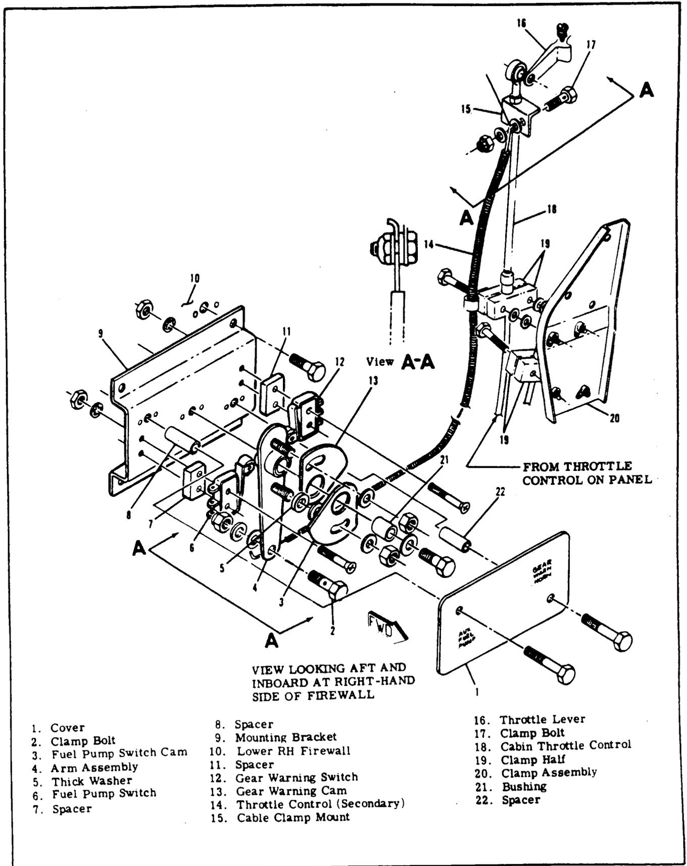
Figure 13-7. Throttle-Operated Microswitches
