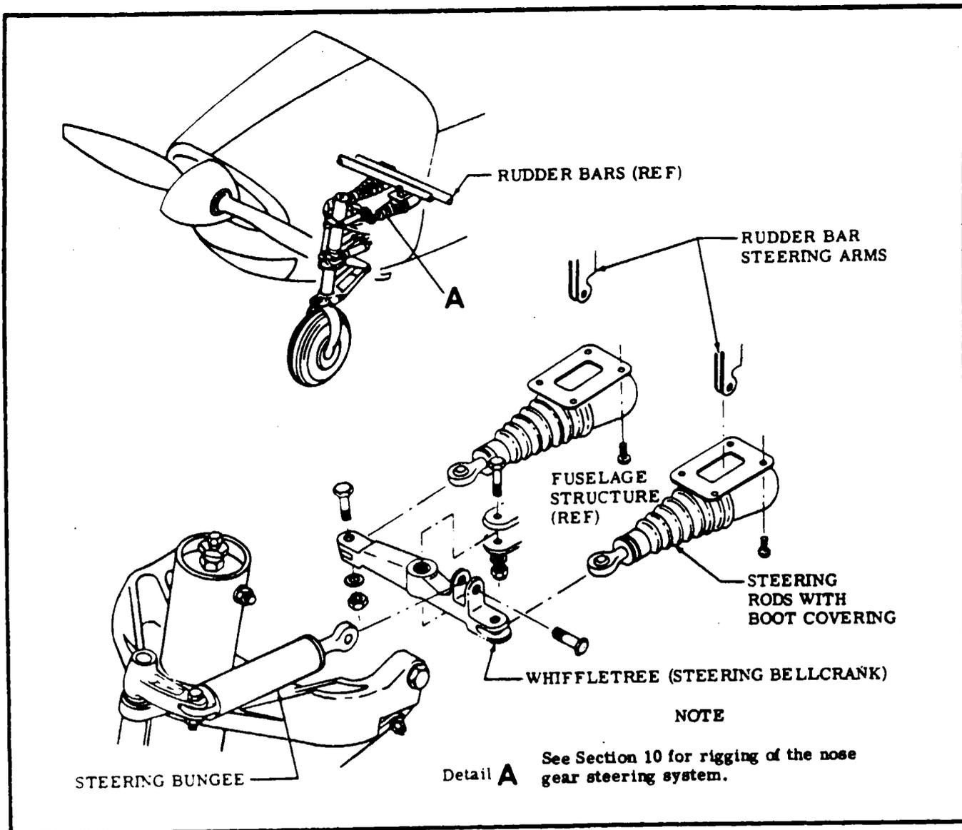
Figure 5-23. Nose Wheel Steering System
