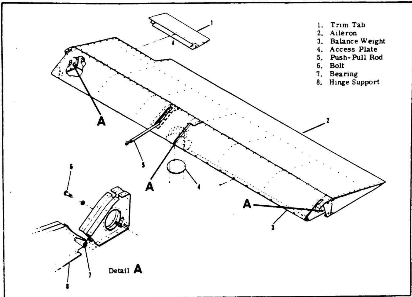
Figure 6-3. Aileron Installation
