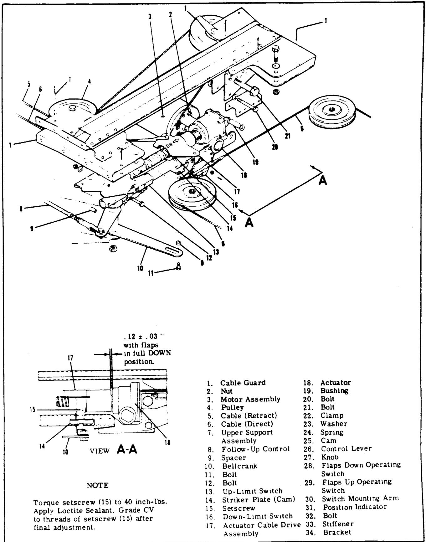
Figure 7-1. Wing Flap Control System (Sheet 2 of 3).
