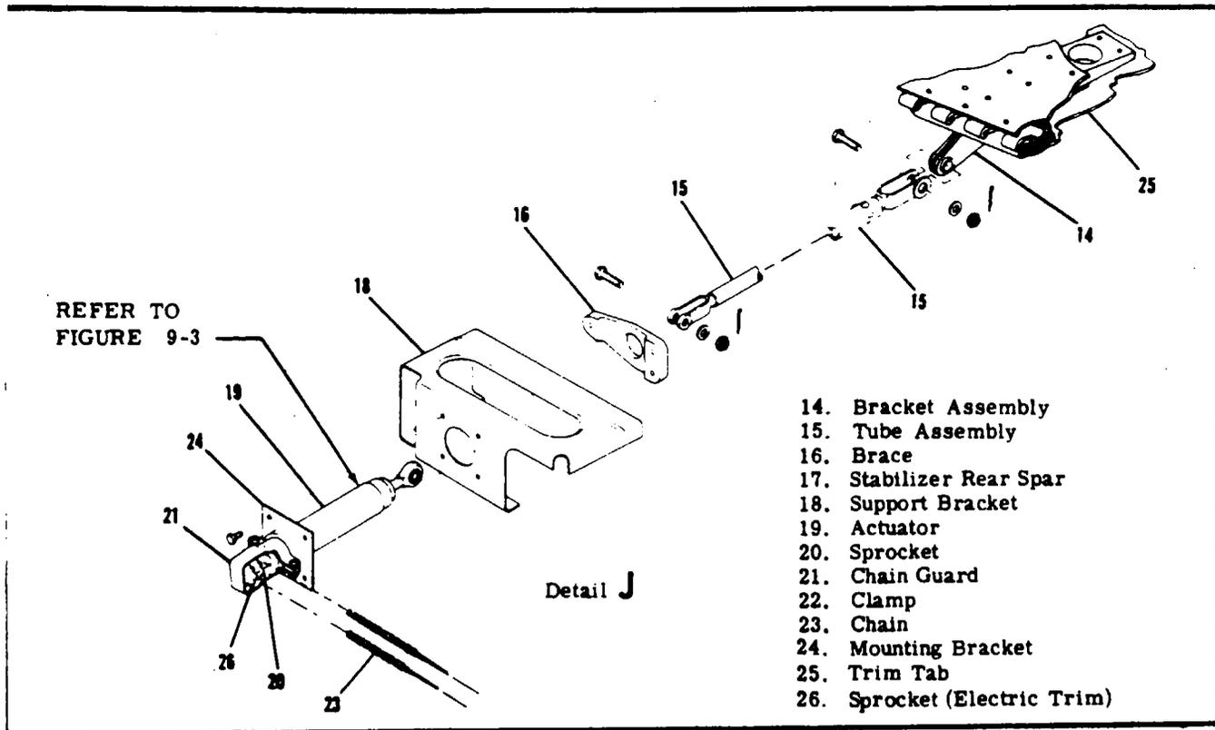
Figure 9-1. Elevator Trim Tab Control System (Sheet 2 of 2)
