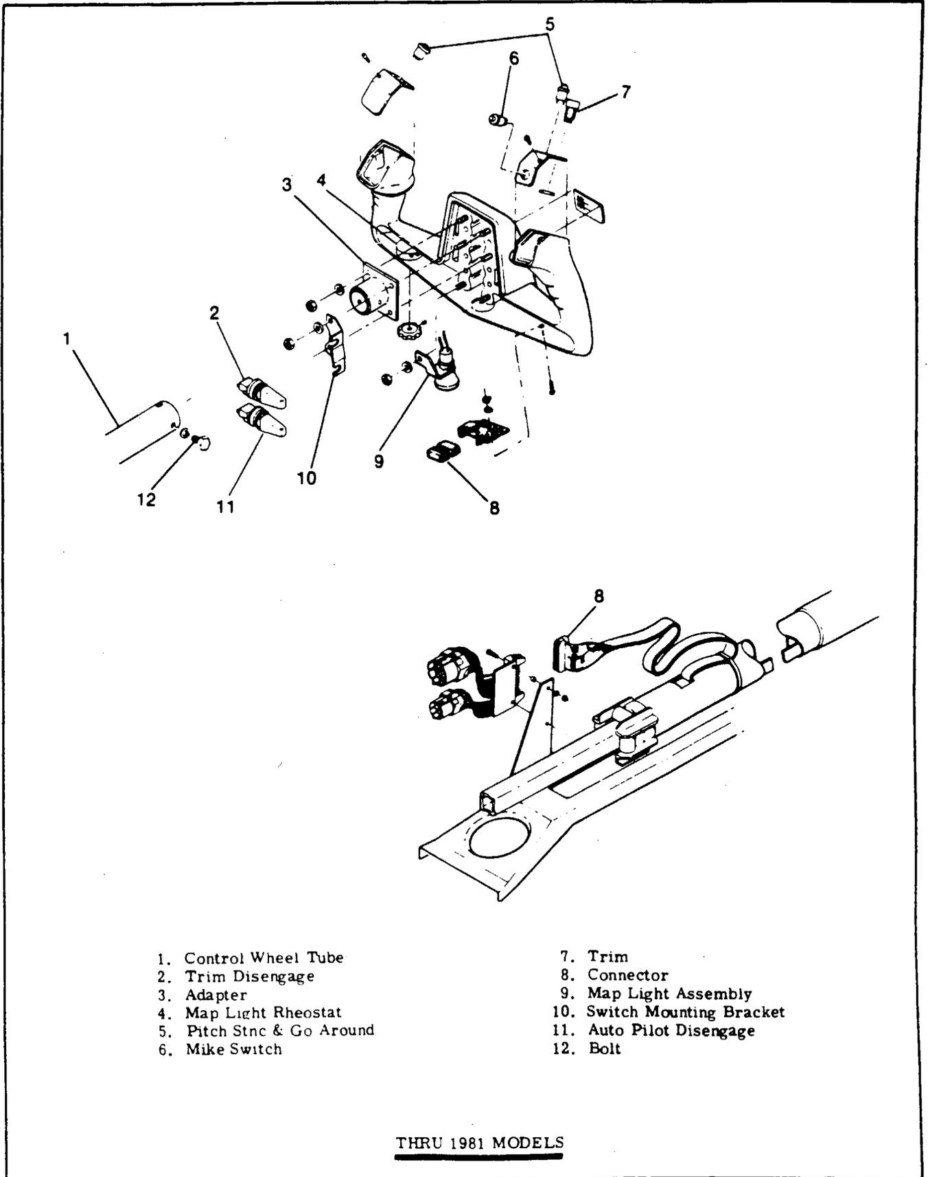
Figure 6-2. Control Column Installation (Sheet 3 of 5)
