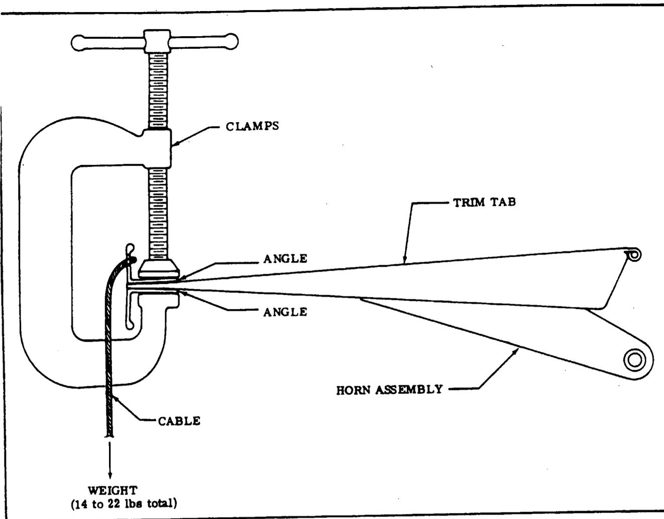
Figure 9-8. Trim Tab Simulated Air Load Test
