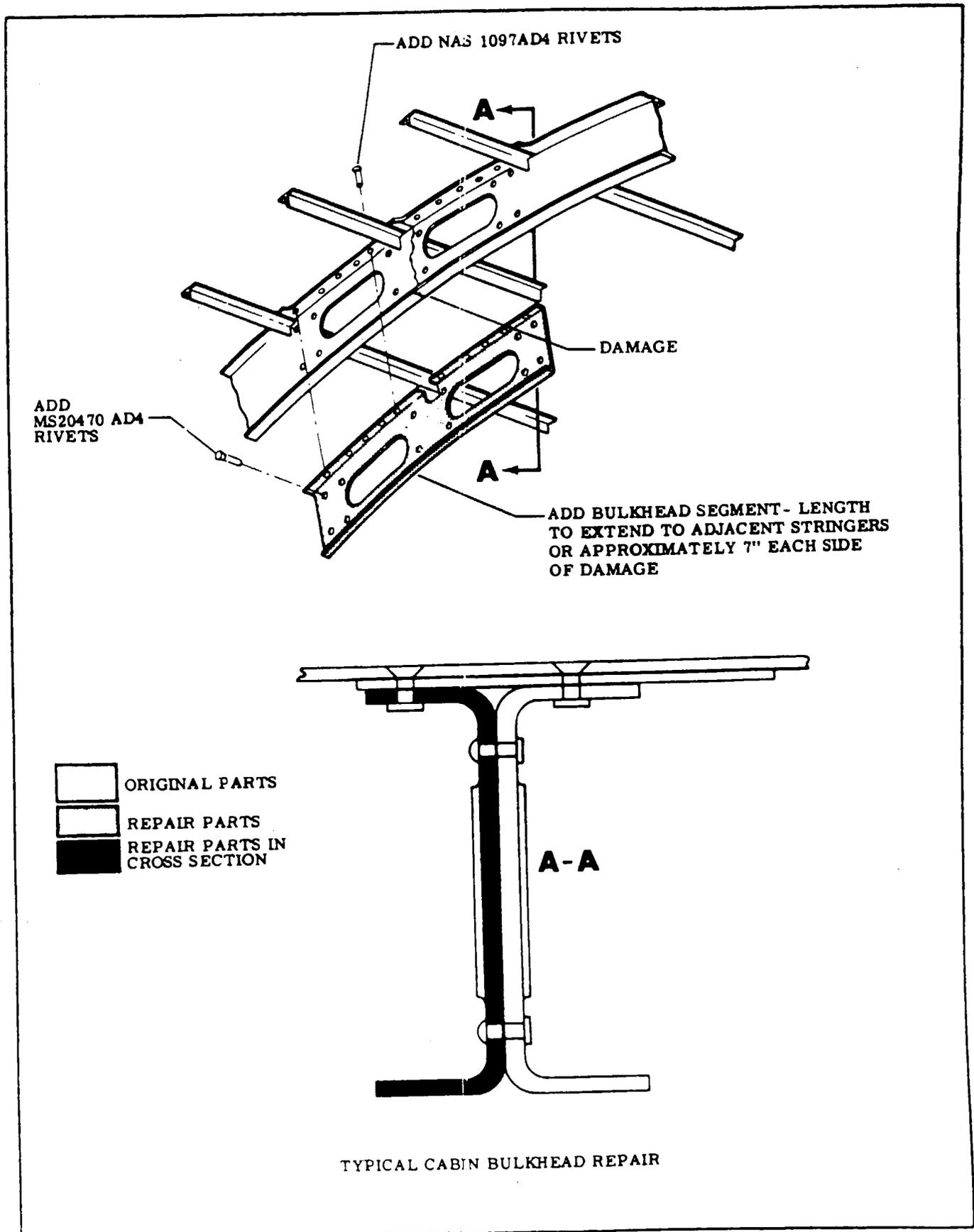
Figure 18-15. Typical Cabin Bulkhead Repair (Sheet 2 of 2)
