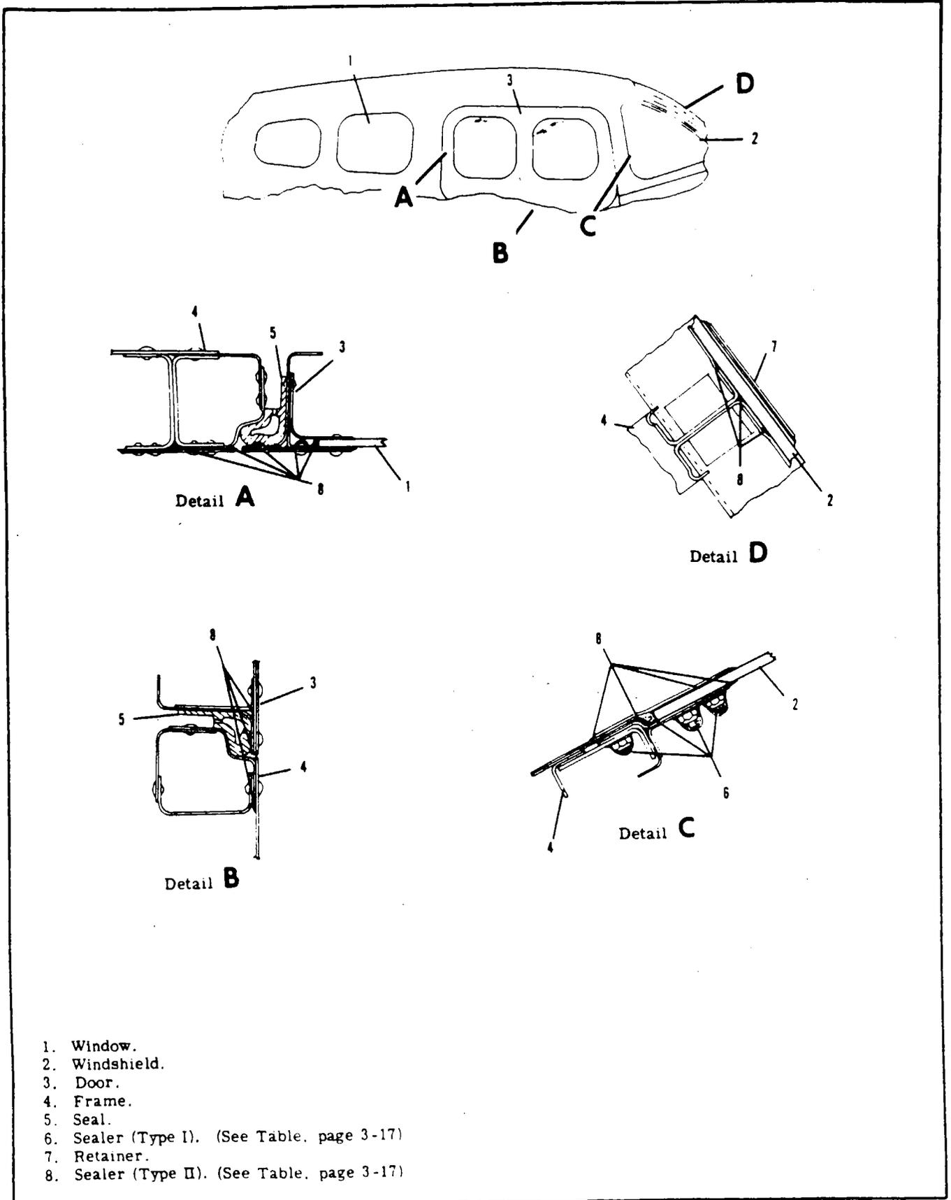
Figure 3-7. Door and Window Sealing.
