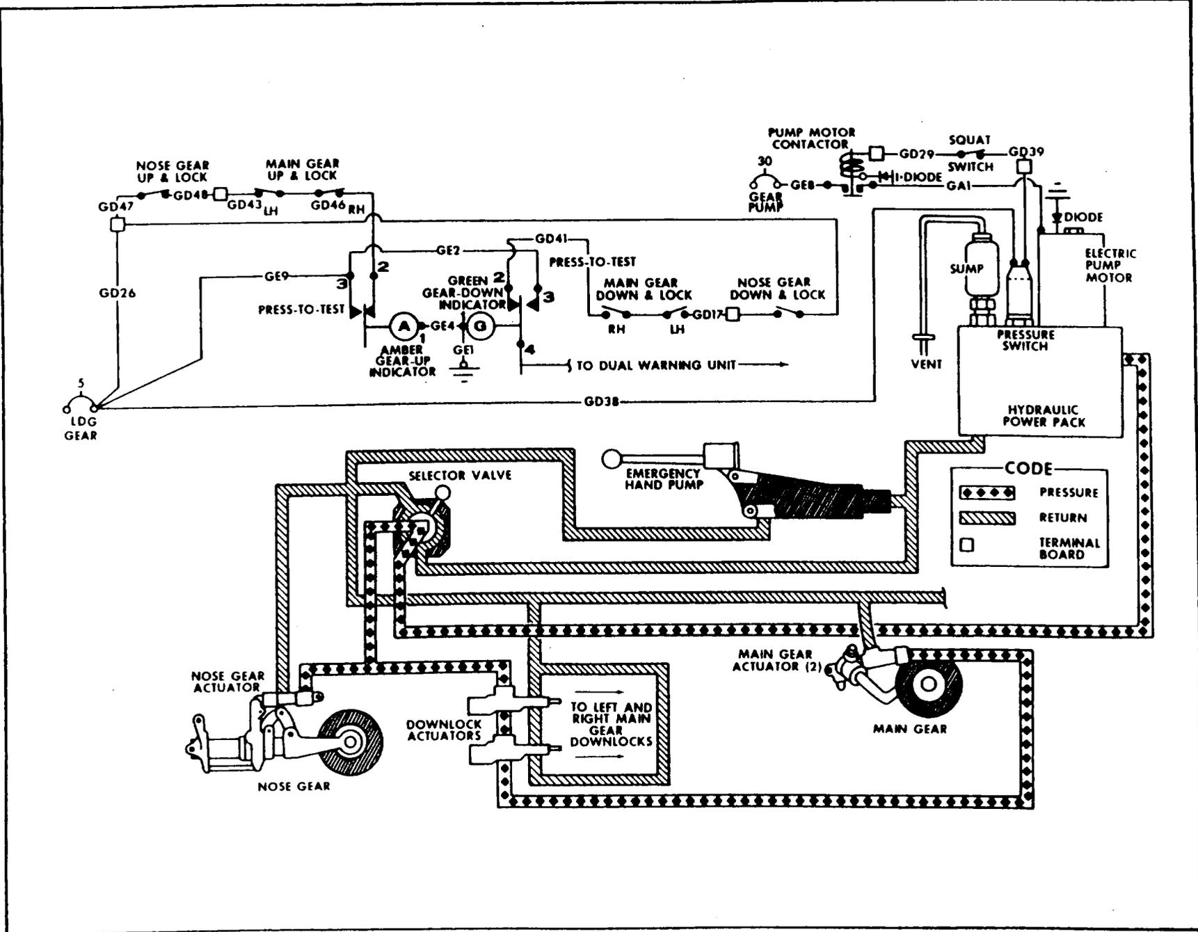
Figure 5A-1. Landing Gear Schematic (Sheet 2 of 4)
