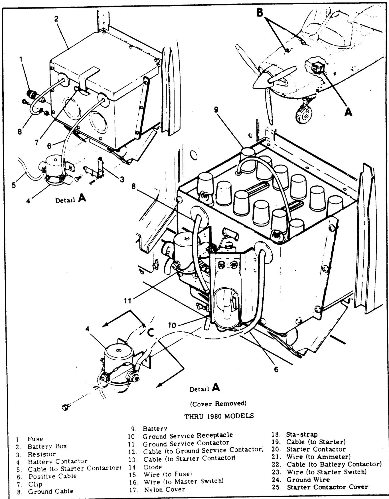
Figure 17-2. Battery and Electrical Equipment Installation (Sheet 1 of 4)
