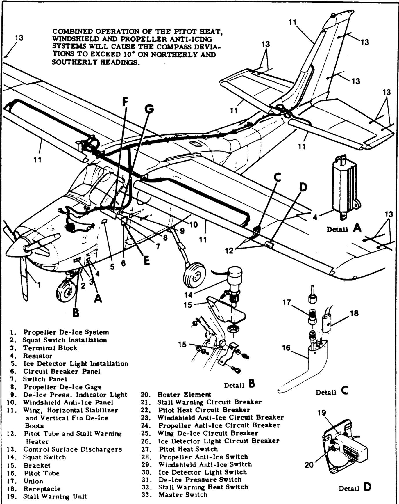
Figure 15-6A. Known Icing Equipment (Sheet 1 of 4)
