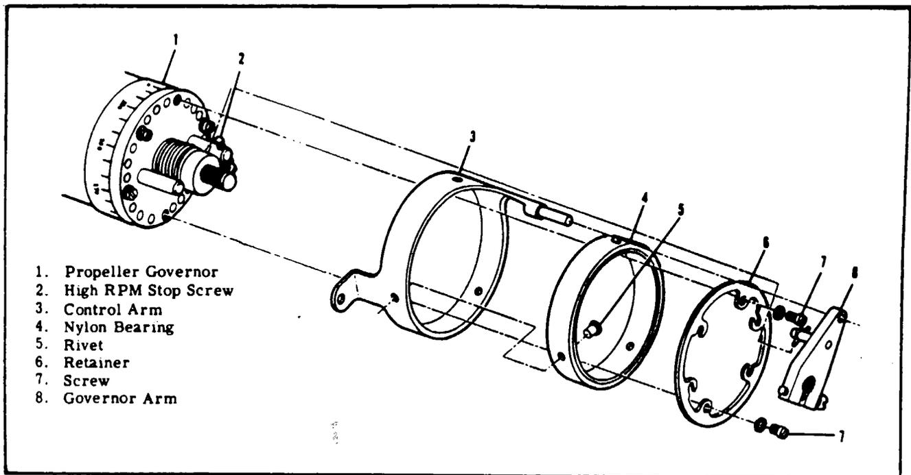
Figure 14-2. Governor Control Arm and Bearing Assembly
