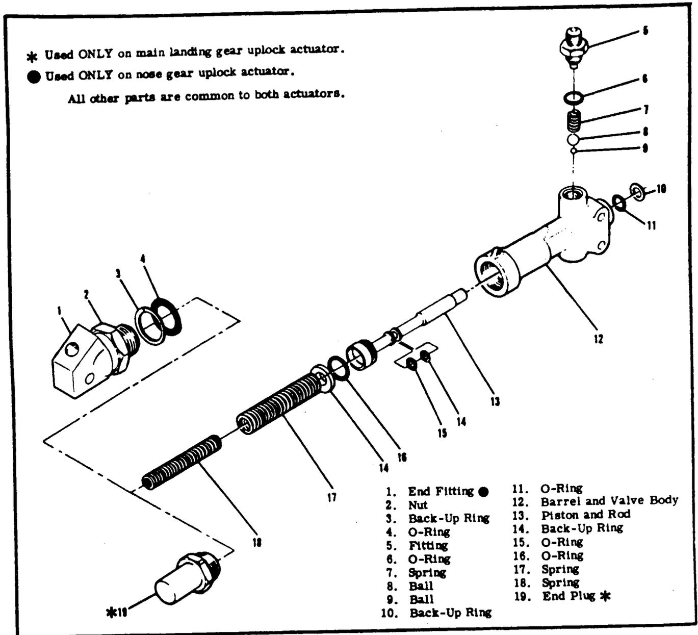
Figure 5-5. Lock and Unlock Actuators
