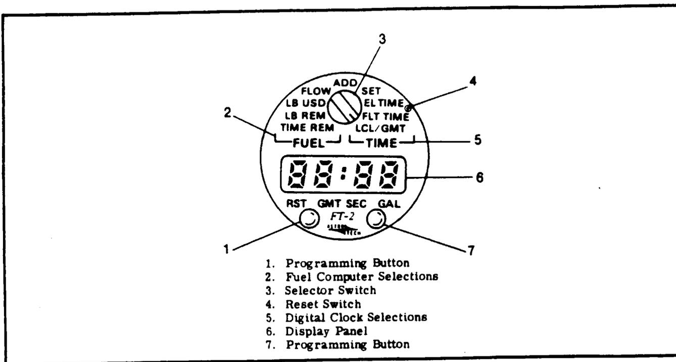
Figure 16-9. Fuel Computer/Digital Clock.
