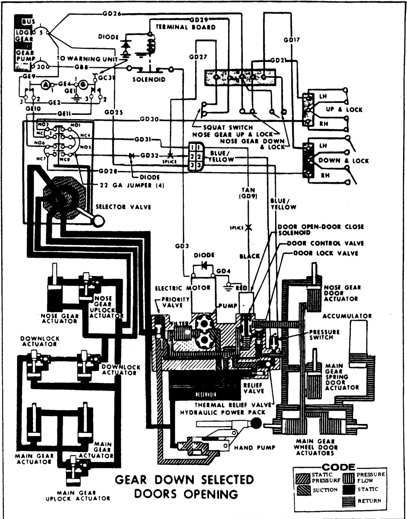
Figure 5-38. Hydraulic and Electrical System Schematic (Sheet 2 of 7)
