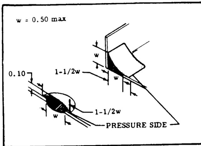
Figure 18-5. Hole Filling
