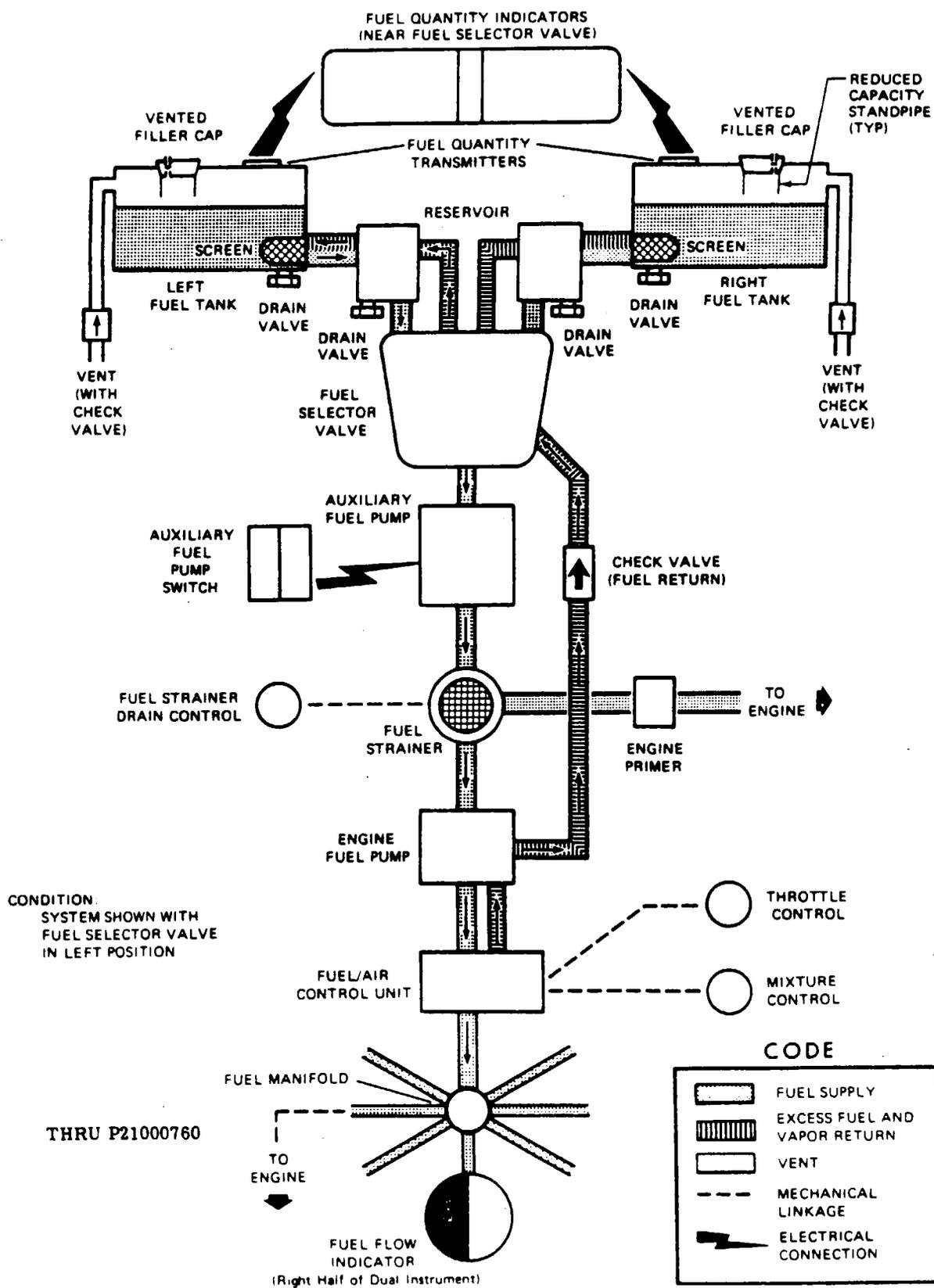
Figure 13-1. Fuel System Schematic
