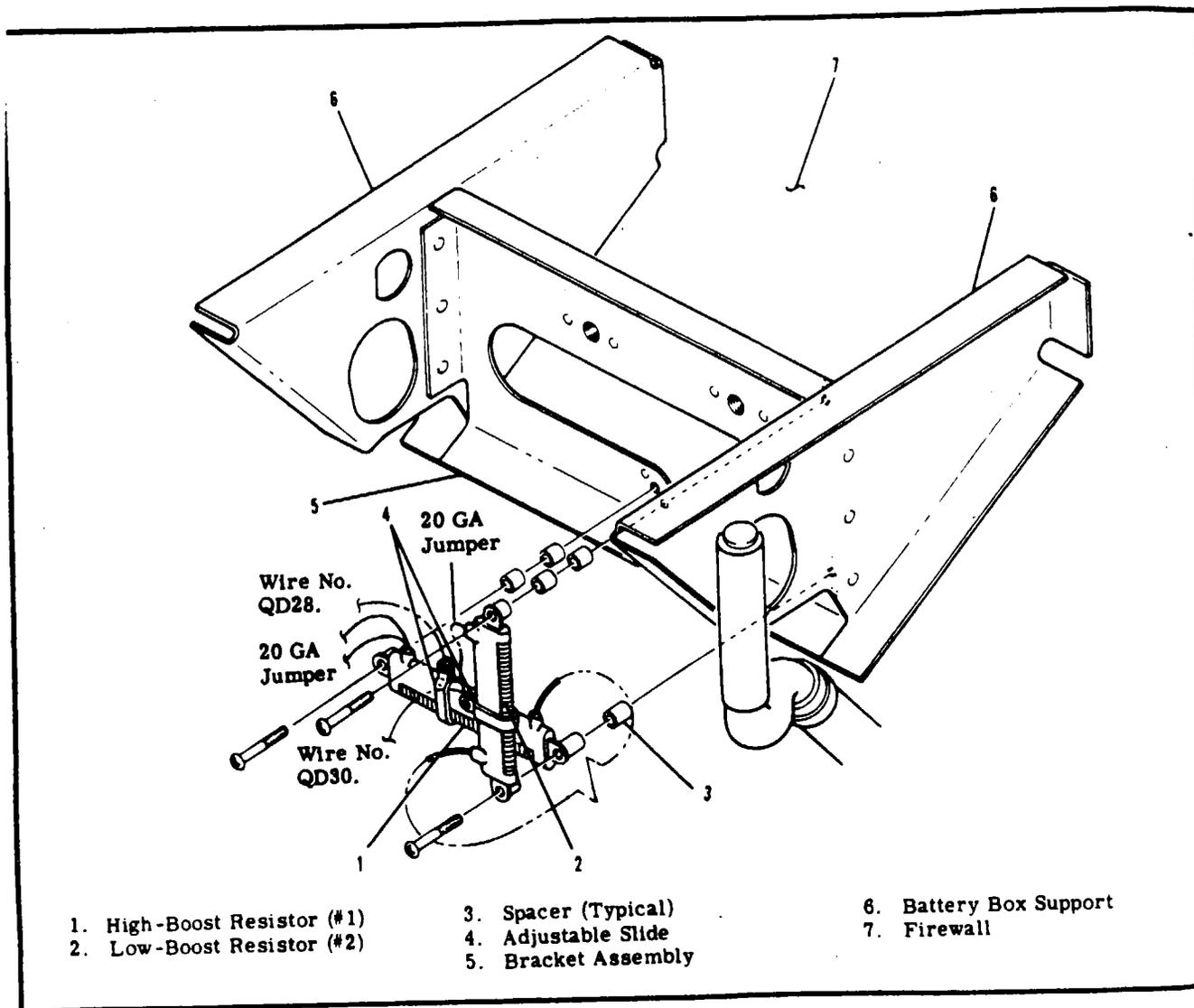
Figure 13-8. Auxiliary Fuel Pump Resistors
