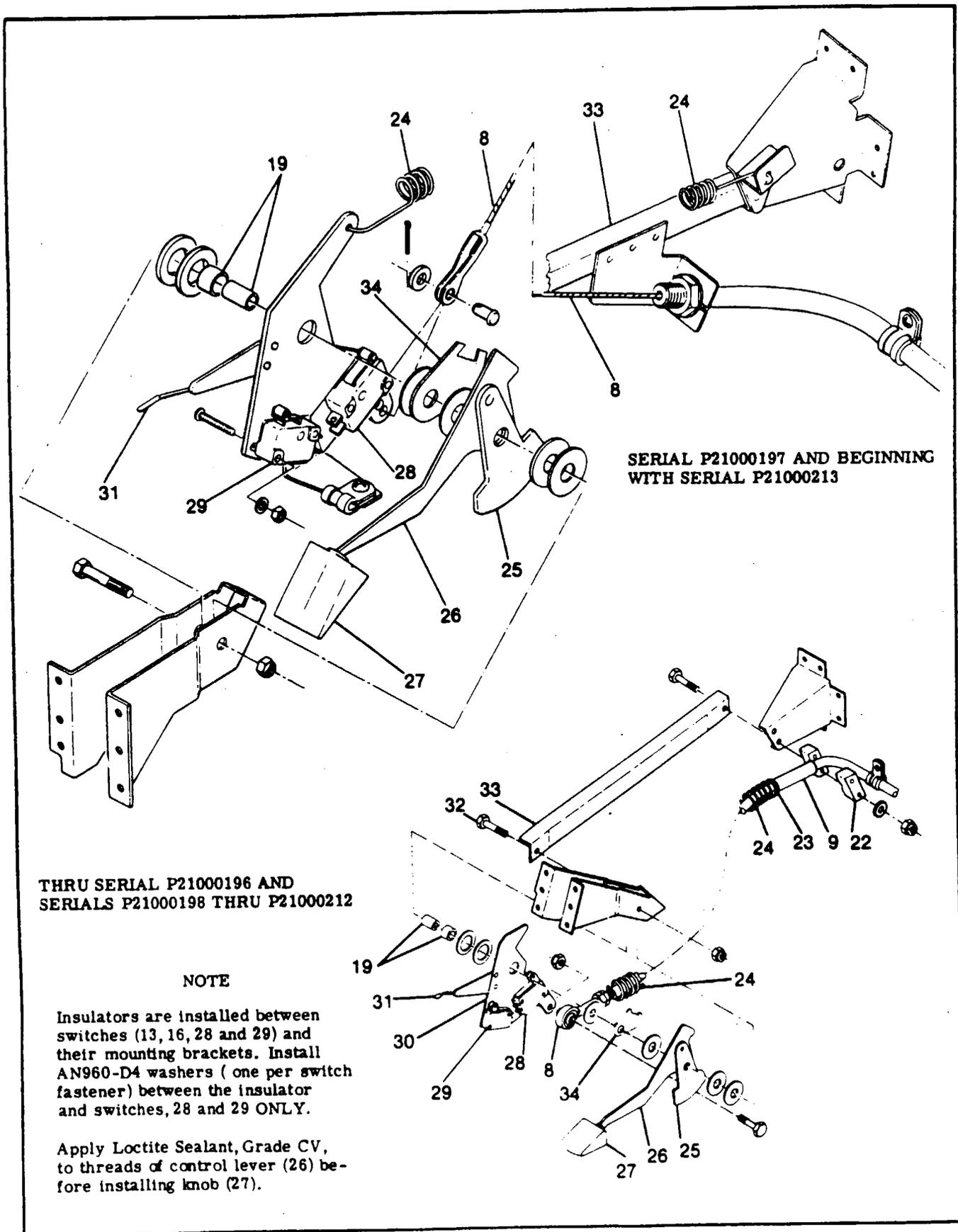
Figure 7-1. Wing Flap Control System (Sheet 3 of 3)
