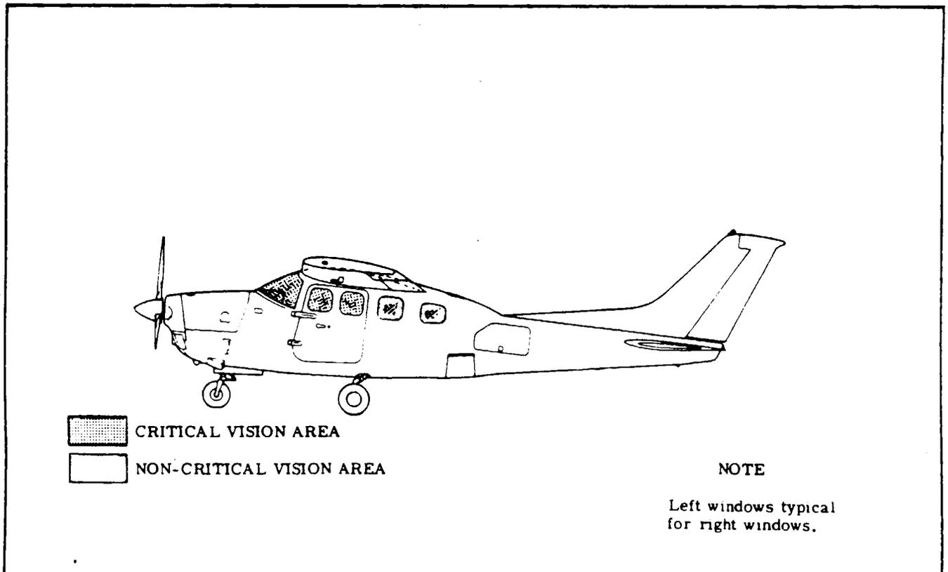
Figure 3-1. Critical Vision Diagram
