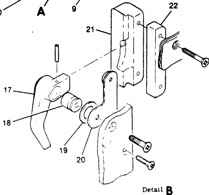
Figure 3-4. Cabin Door Sliding Window Installation
