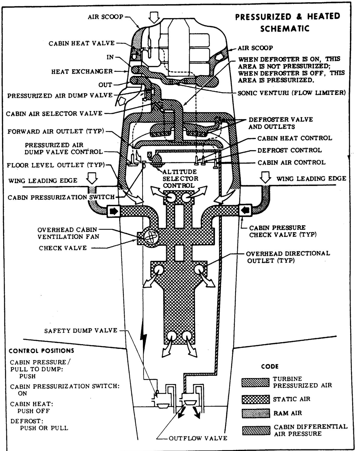
Figure 15-2. Cabin Air Flow Schematic (Sheet 6 of 6)
