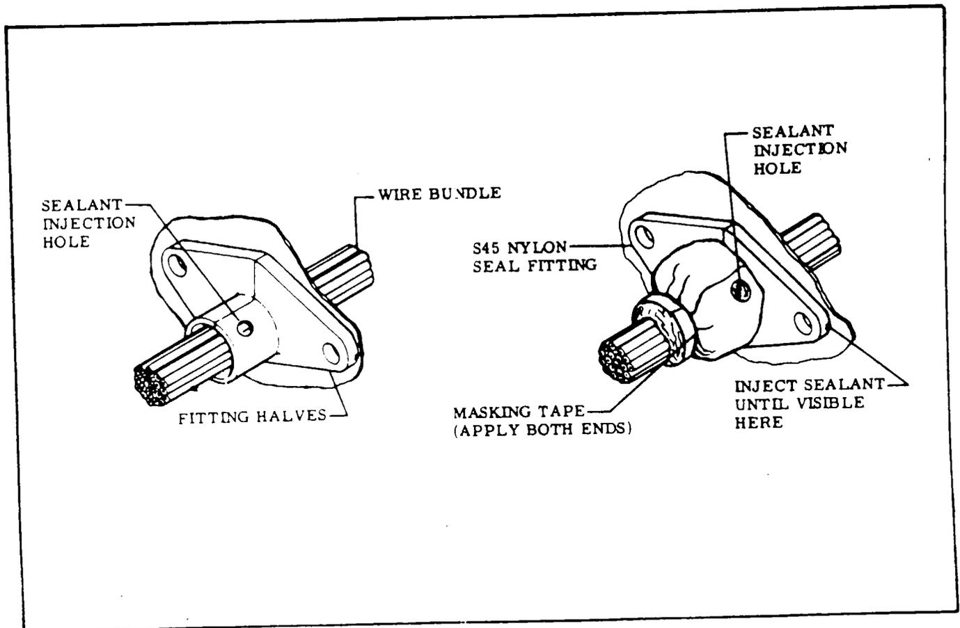
Figure 18-10. Electrical Sealing
