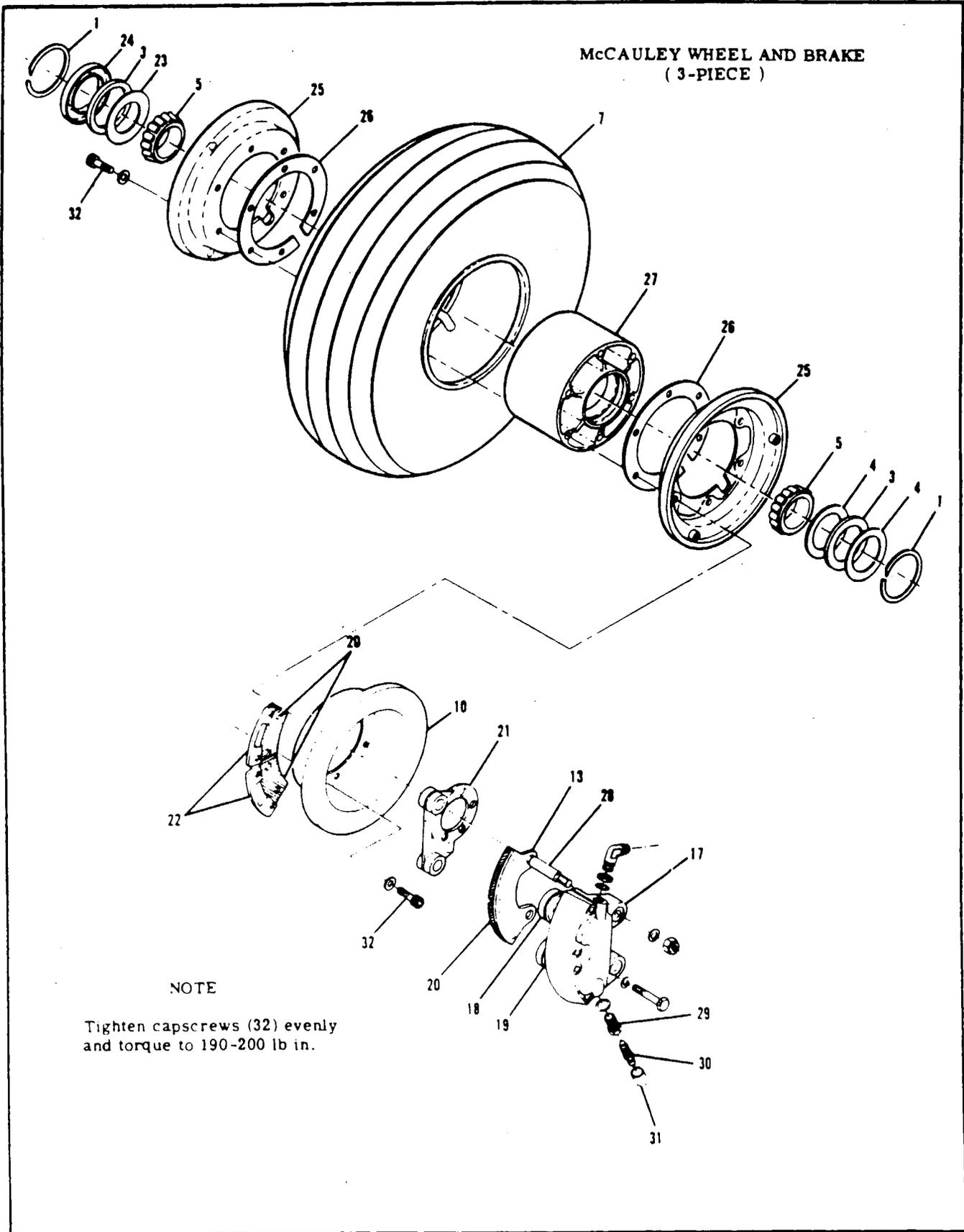
Figure 5-10 Main Landing Gear Wheel, Tire and Brake Assembly ( Sheet 3 of 3 )
