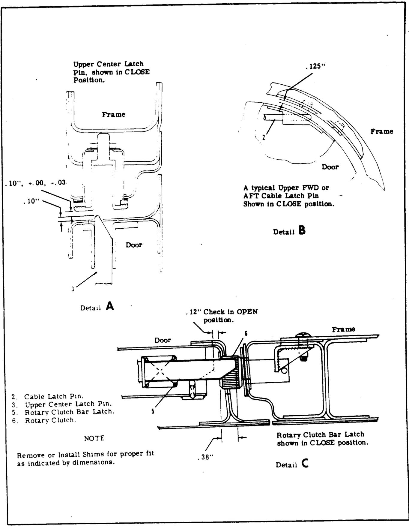
Figure 3-5. Door Latch Mechanism (Sheet 4 of 4).
