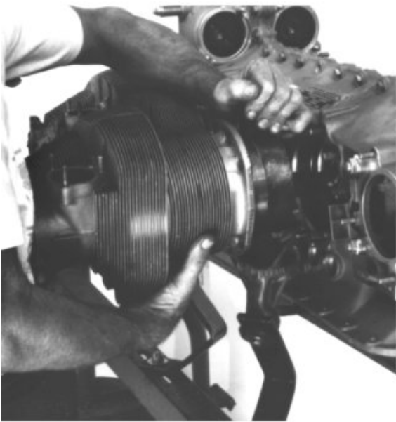
FIGURE 18-9A. INSTALLING NO. 3 CYLINDER
