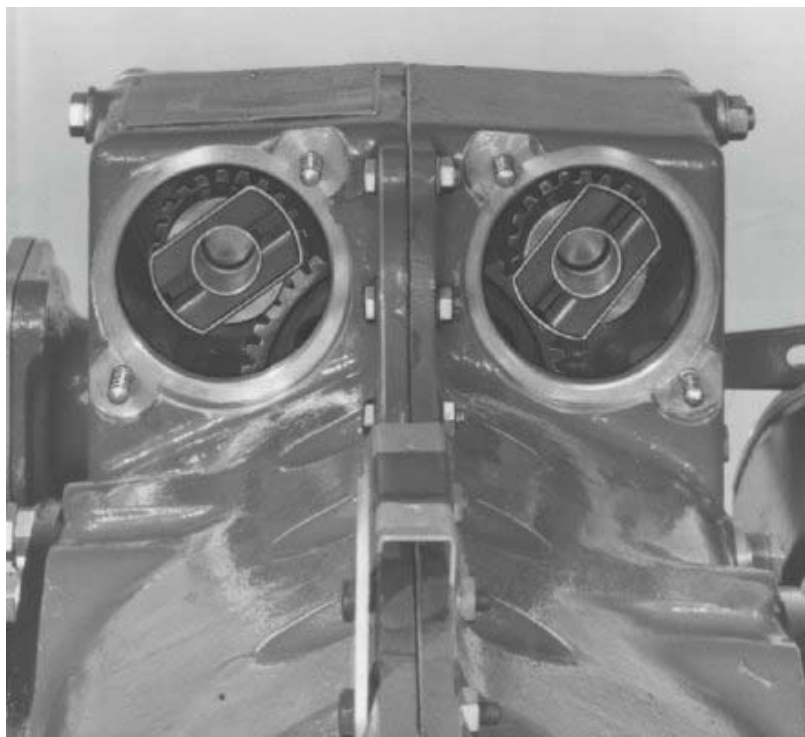
FIGURE 18-19. POSITION OF MAGNETO COUPLINGS
