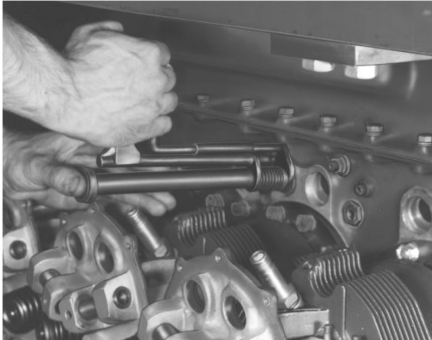
FIGURE 18-17. INSTALLING PUSHROD HOUSING
