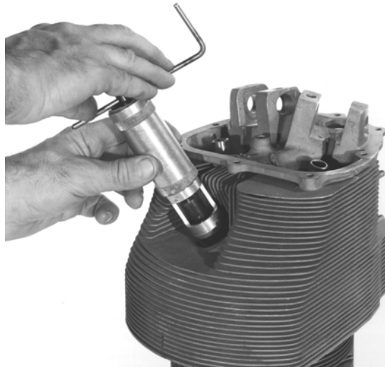
FIGURE 15-6B. INSTALLING SPARK PLUG HELICAL COIL
