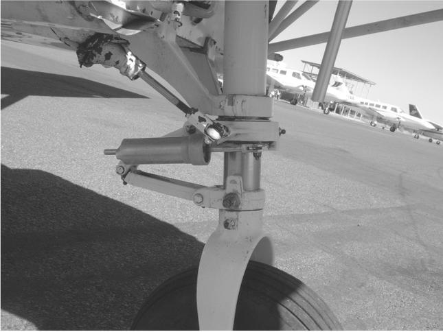
Check security of nuts and split pins, state of tyre
