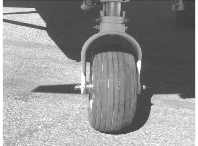
Check freedom of operating linkage, and security and state of shimmy damper.
