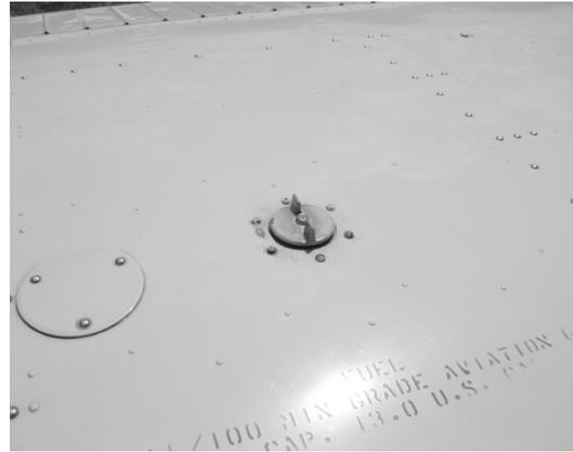
Check that fuel cap is secure again after checking the fuel level.
