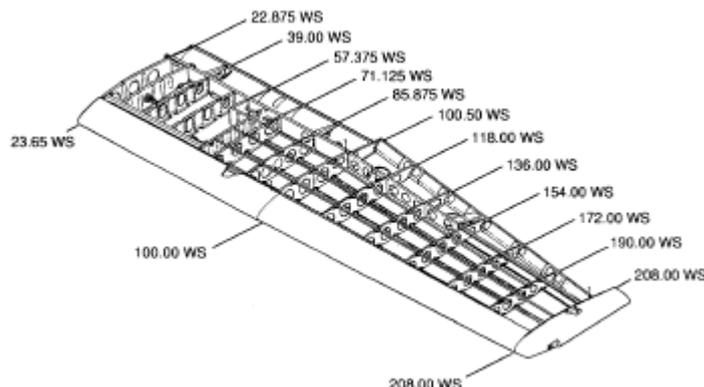
The front spars are equipped with wing-to-fuselage and wing-to-strut attach fittings. The aft spars are equipped with wing-to-fuselage attach fitting, and are partial-span spars. The wings contain the integral ie. non bladder type fuel tanks. The empennage or tail assembly consists of the vertical stabilizer and rudder, horizontal stabilizer and elevator.
