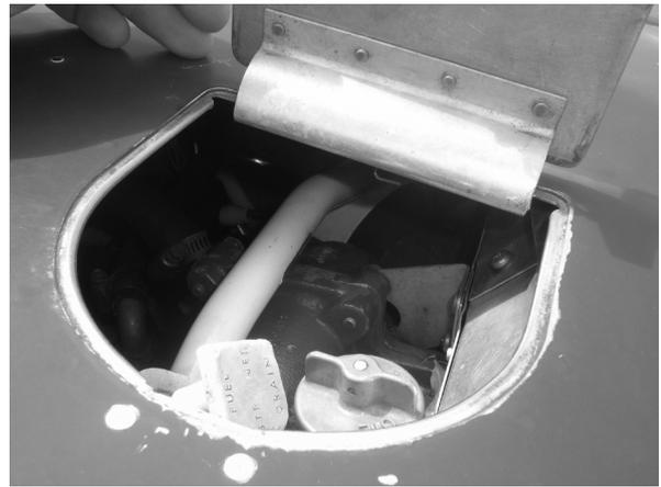
Check oil level above minimum. Before first flight of the day and after each refuelling, take a fuel sample. Check strainer drain valve, oil cap and inspection cover are properly closed once inspection complete.
