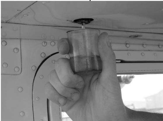
Use sampler cup and drain a small quantity of fuel from wing tank quick-drain valve to check for water, sediment and proper fuel grade.
