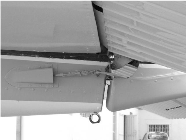
Check rudder linkages and turn-buckles secure, unobstructed, and elevator has free movement (do not check full movement with nose wheel on the ground).
