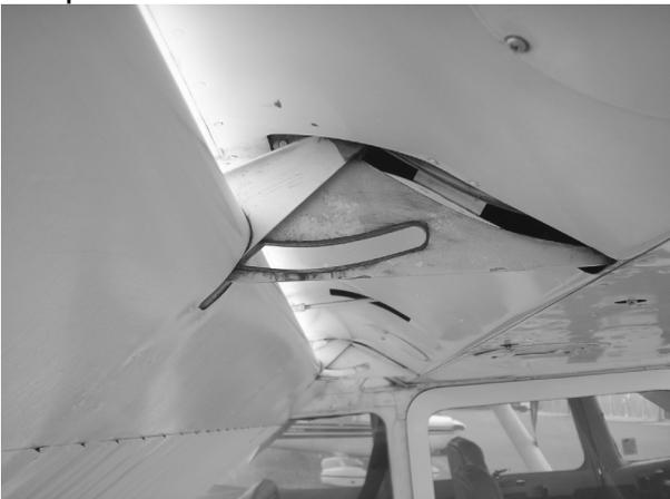
Check for damage to surfaces or flap tracks, ensure rollers are free and in good condition, and all fastenings secure.
