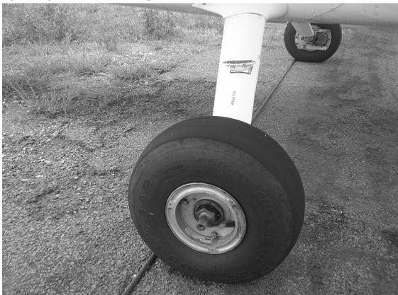
Check the tyre for wear, cuts, bruises, slippage and recommended tyre pressure. Remember, any drop in temperature of air inside a tyre causes a corresponding drop in air pressure.
