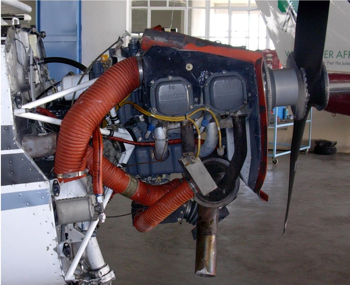
Early models of 172 (before 1967 models) are powered with Lycoming O-300, six cylinder engine, in later models was replaced with Lycoming O-320, four cylinder engine. The O-320 engine had three versions before being replaced by the O-360 engine. The O-360 had two variations before introduction of the fuel injected IO-360 engine in the "restart" models (1996 and later)
