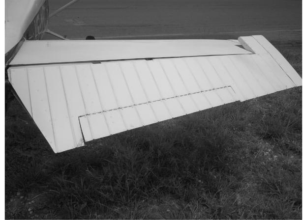
Ensure elevator and trim secure and undamaged, linkages free and unobstructed, check full and free movement of elevator.
