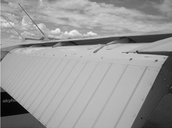
Ensure aeriels undamaged and secure. Check flap does not retract if pushed and flap rollers allow small amount of play in down position.
