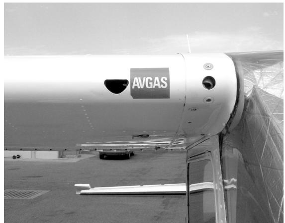
Check top and bottom wing surfaces for any damage or accumulations. *Ice or excessive dirt must be removed before flight.*
