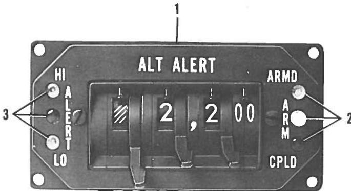
1. **ALTITUDE SELECTOR AND DISPLAY** - Three minilever switches select desired altitude between 100 feet and the aircraft's maximum service ceiling in 100-foot increments. Digital readout displays selected altitude. Black/white flag in first window, when visible, indicates selected altitude is less than 10,000 feet.
