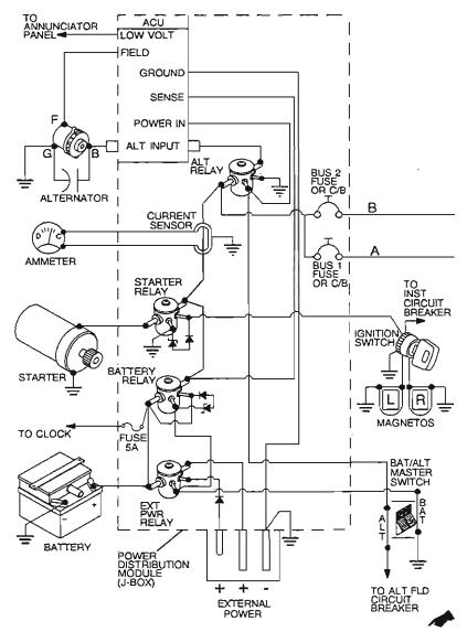
Figure 7-7A. Electrical Schematic (Serials 172S8704 and On) (Sheet 1 of 2)
