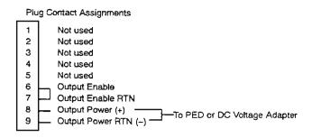
Figure 3. Mating Plug Wiring
