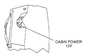
Figure 1. 12 Volt Cabin Power System Connector
