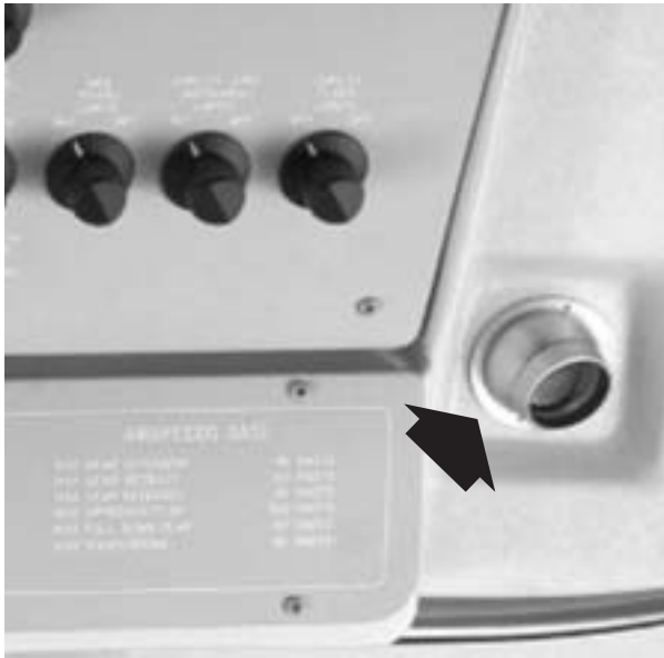
Figure 11-5. Cockpit “Eyeball” Outlets
