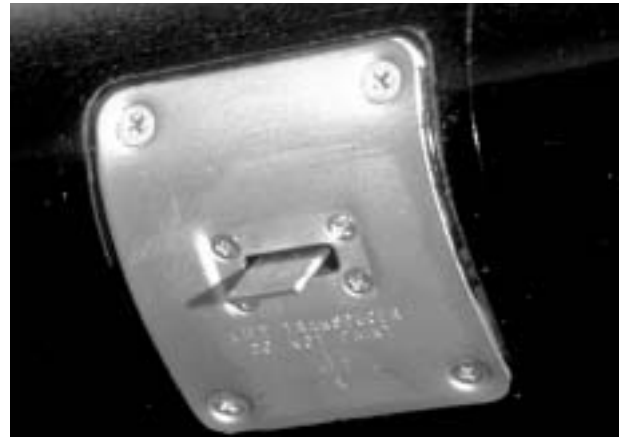
Figure 16-20. Stall Warning Transducer Vane
