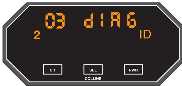
IND-42C SELF-TEST DISPLAY 03 (TRANSMITTER) FAULT FOUND
