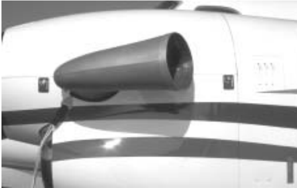
27. EXHAUST STACK (OUTBOARD)—CHECK FOR CRACKS 28. TOP COWLING LOCKS (OUTBOARD)—SECURE
