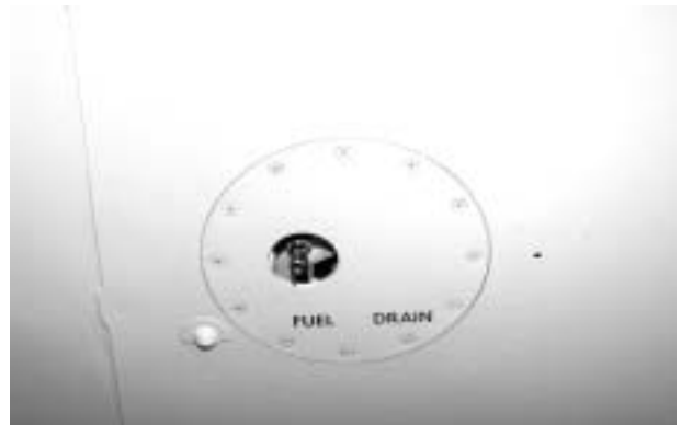
41. AUXILIARY FUEL TANK SUMP—DRAIN
