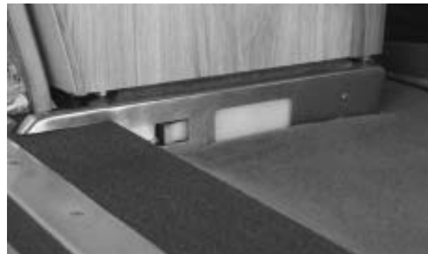
Figure 3-13. Threshold, Aisle, and Baggage Lights
