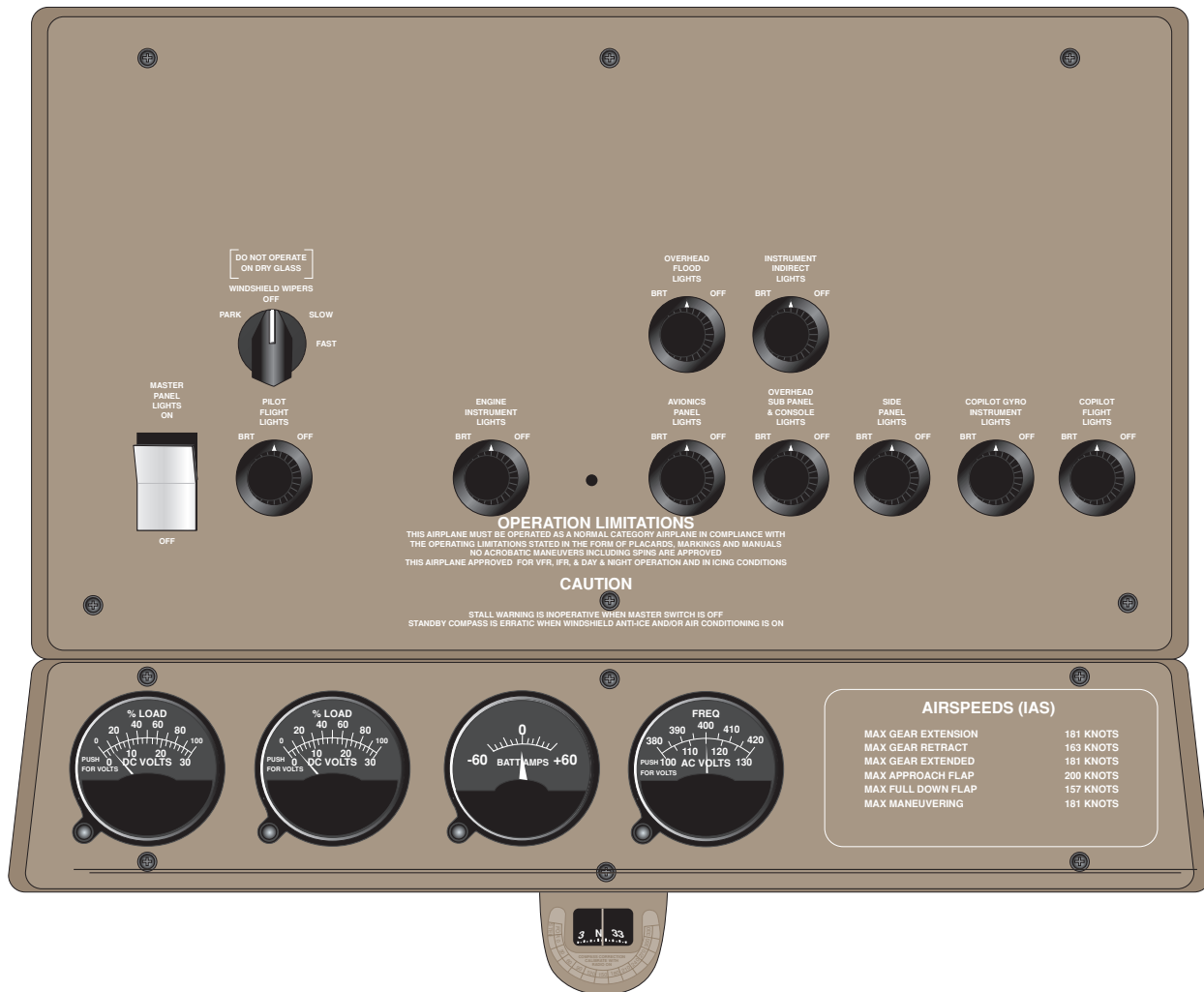
Figure 3-1. Overhead Lighting Controls
