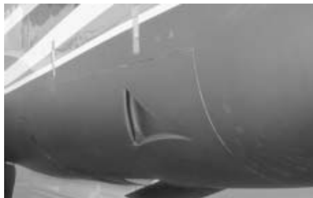
35. GENERATOR COOLING INLET—CLEAR
