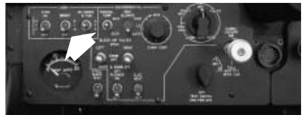
Figure 3-10. Fluorescent Light Switch
