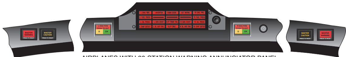
AIRPLANES WITH 20-STATION WARNING ANNUNCIATOR PANEL
