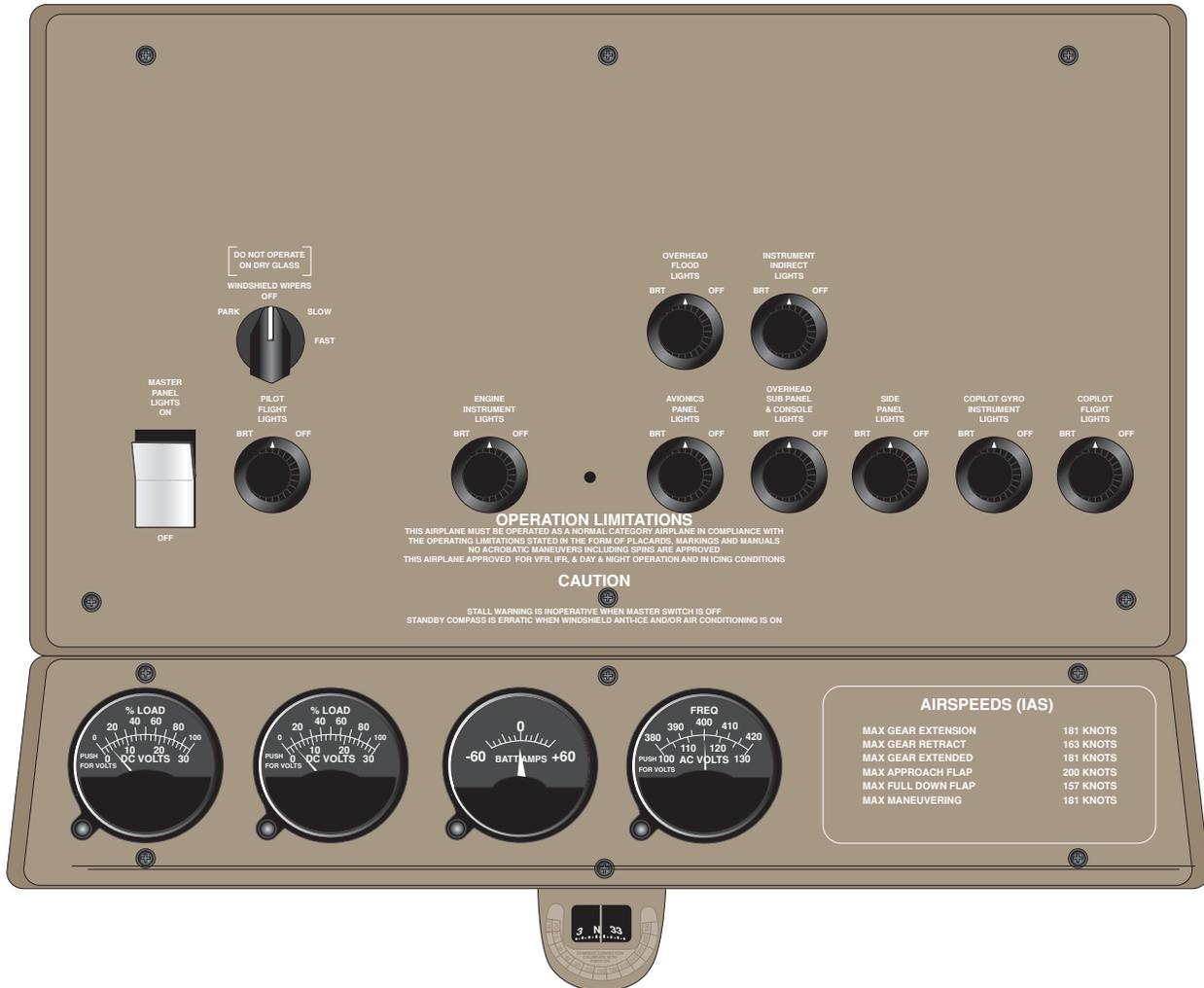
**Figure 3-1. Overhead Lighting Controls**
