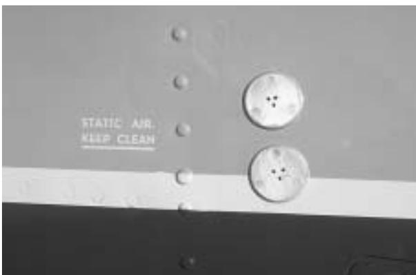
**Figure 16-16. Static Ports Location**
