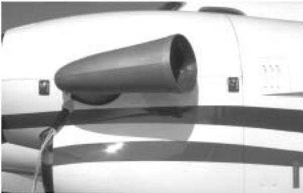
27. EXHAUST STACK (OUTBOARD)—CHECK FOR CRACKS
