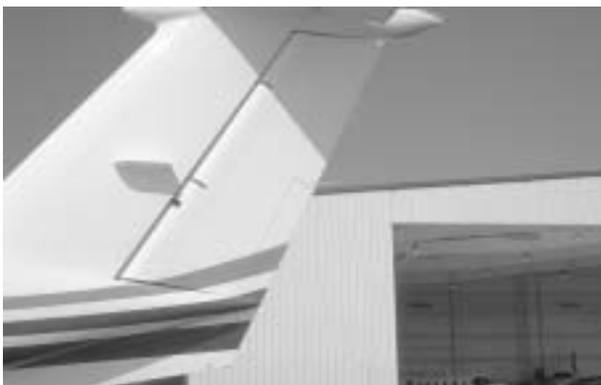
**106. RUDDER, STATIC WICKS (4)—CHECKED**
