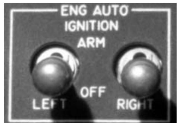
**Figure 7-14. Engine Autoignition Switches**
