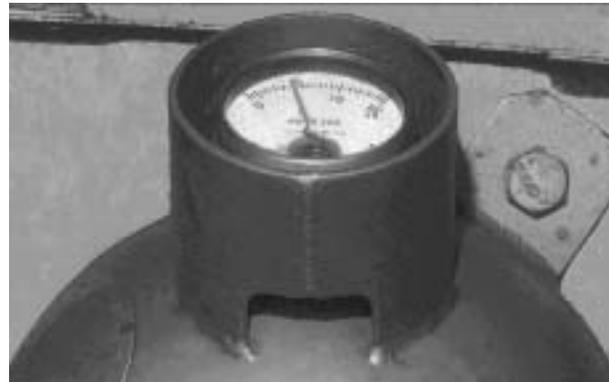
7. FIRE EXTINGUISHER PRESSURE (IF INSTALLED)—CHECK
