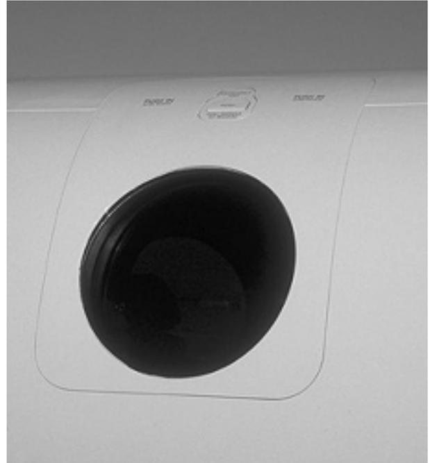
**Figure 1-31. Emergency Exit Release Handles**
