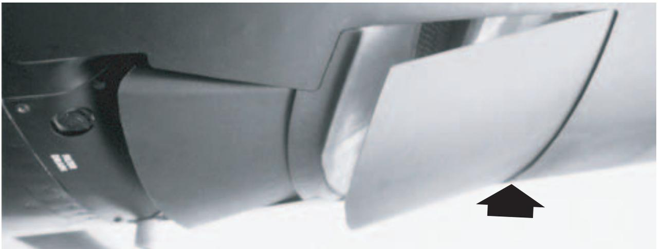
INERTIAL VANE BYPASS DOOR EXTENDED
