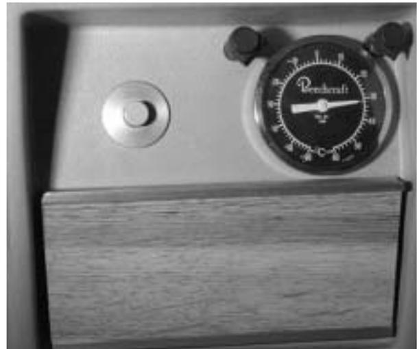
**Figure 3-9. Free Air Temperature Switch**
