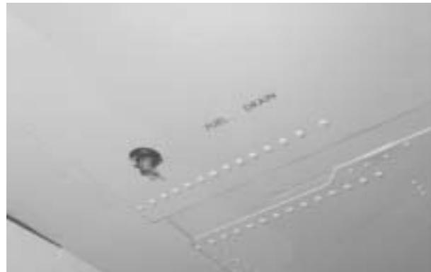
**19. WING LEADING EDGE TANK SUMP—DRAIN**
