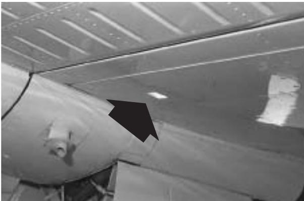
**Figure 3-16. Airstair Floodlight**
