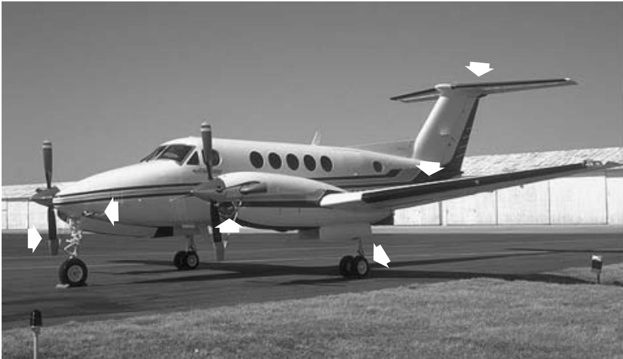
**Figure 10-1. Weather-Protected Airplane Surfaces**
