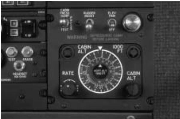
**Figure 1-12. Cabin Pressurization Controller**
