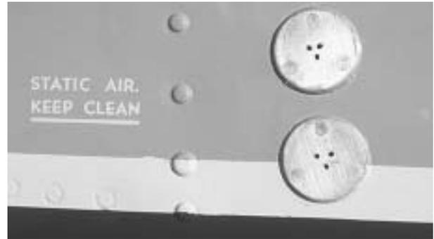
**Figure 1-20. Static Ports**
