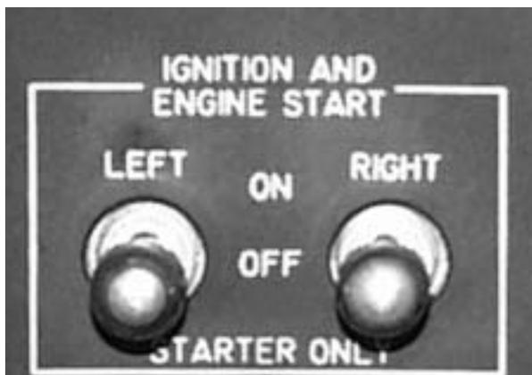
**Figure 7-13. Engine Start and Ignition Switches**
