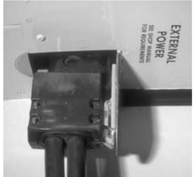
**Figure 1-3. External Power Socket**
