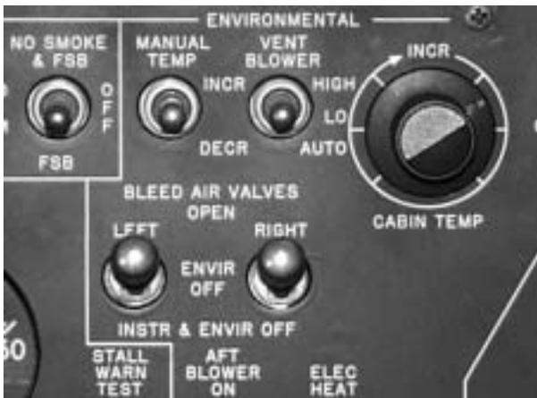
Figure 9-6. BLEED AIR VALVE Switches
