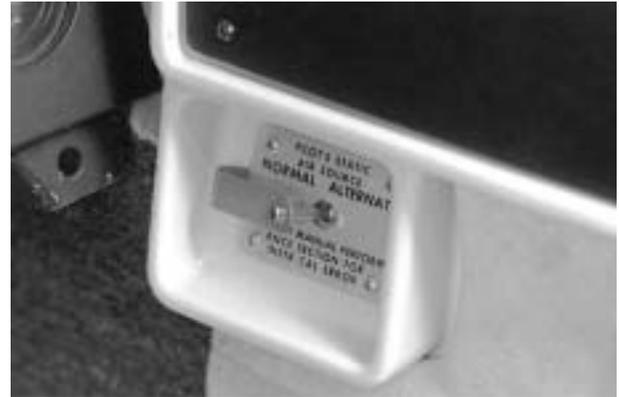
**Figure 16-17. Pilot's Static Air Source Valve Switch**
