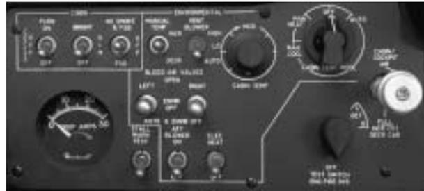
**Figure 1-5. Cabin Lights Control Switch (BB-1439, 1444 and After)**
