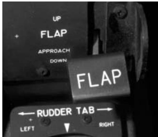
**Figure 1-18. Flap Control Lever**
