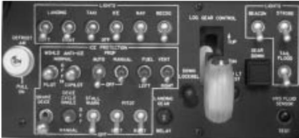
**Figure 1-6. Exterior Lights Control Switches**
