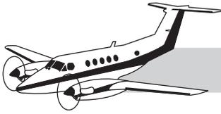
A minimum of 85% power on each engine is necessary to maintain proper boot inflation if the hot brake system is on.
