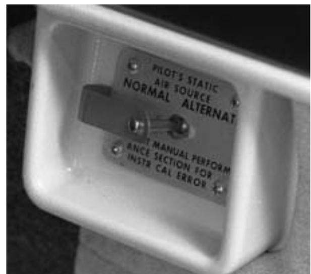
**Figure 1-21. Pilot's Static Air Source Valve Handle**
