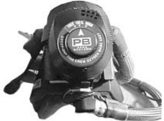
**Figure 17-4. O<sub>2</sub> Mask Selector (BB-1439, 1444 and After—Puritan Bennett)**
