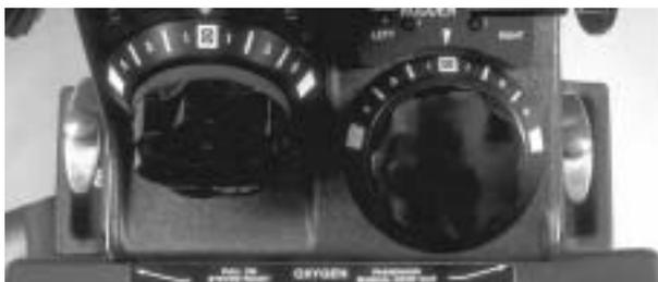
**Figure 17-7. Oxygen System Push-Pull Handles (BB-1439, 1444 and Subsequent)**
