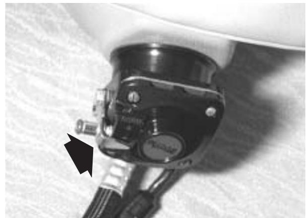
**Figure 17-5. O<sub>2</sub> Mask Selector (Prior to BB-1444, Except 1439)**
