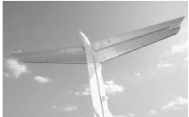
**108. ELEVATOR, ELEVATOR TAB, STATIC WICKS (3 EACH SIDE)—CHECKED**
