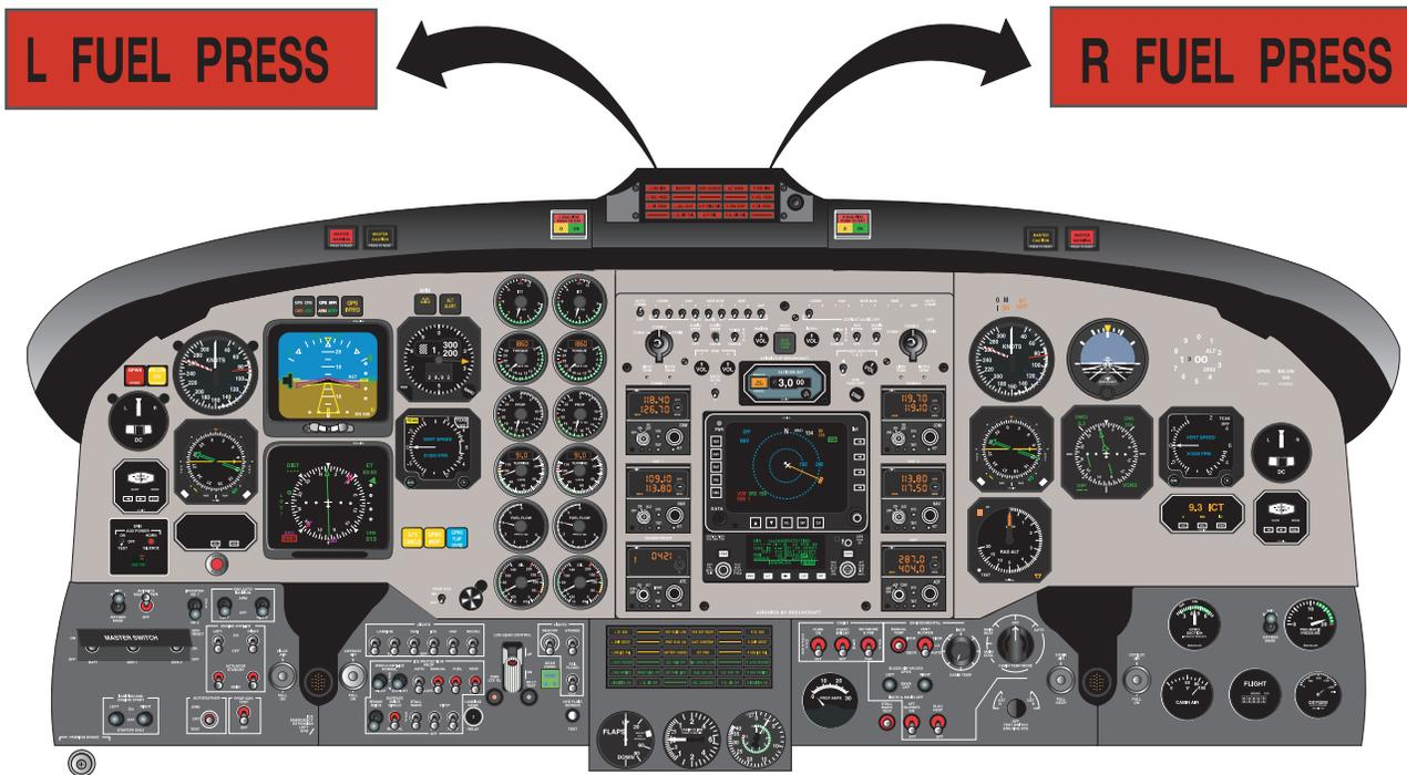
Figure 5-4. Fuel Pressure Warning Lights
