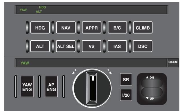
**Figure 15-5. Autopilot and Yaw Damp Switches**
