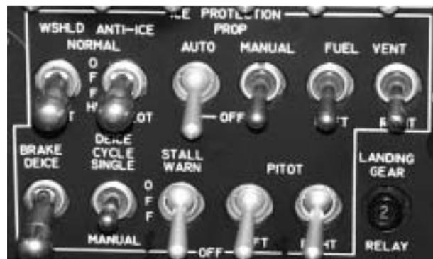
**Figure 1-10. Ice Protection Switches—Pilot's Subpanel**
