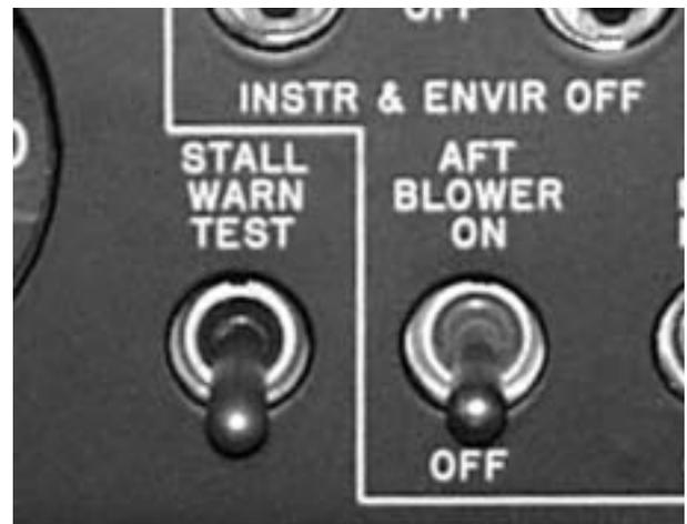
Figure 16-21. STALL WARN TEST Switch (Copilot's Left Subpanel)
