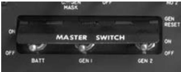
**Figure 2-7. Generator Switches**
