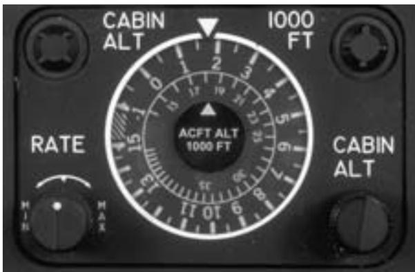
Figure 12-6. Pressurization Controller
