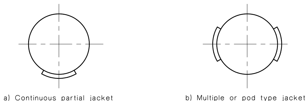
FIGURE 3.23.7 SOME TYPES OF PARTIAL JACKET
